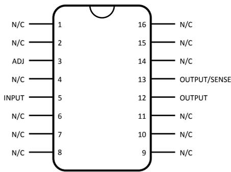
For the Ceramic SOIC device to function properly, the "Output" and "Output/Sense" pins must be connected on the users printed circuit board.
