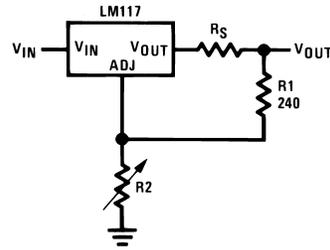
**Figure 17. Regulator with Line Resistance in Output Lead**
