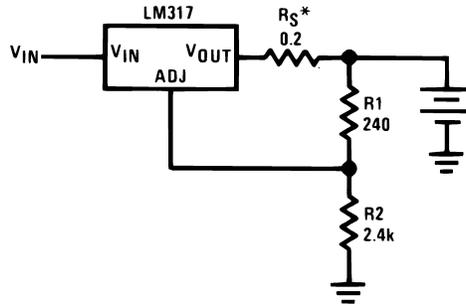
\* $R_S$ —sets output impedance of charger:  $Z_{OUT} = R_S \left( 1 + \frac{R_2}{R_1} \right)$
