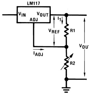
Since the 100µA current from the adjustment terminal represents an error term, the LM117 was designed to minimize  $I_{ADJ}$  and make it very constant with line and load changes. To do this, all quiescent operating current is returned to the output establishing a minimum load current requirement. If there is insufficient load on the output, the output will rise.
