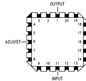
**Figure 4. 20-Pin LCCC Top View See NAJ0020A Package**
