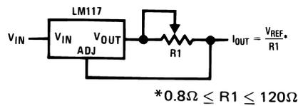
Figure 32. Precision Current Limiter
