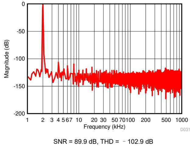
图 8-3. Typical FFT With a 2-kHz Signal
