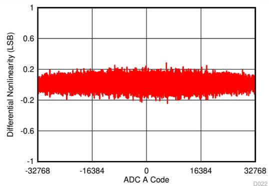
图 6-15. Typical DNL ADC A
