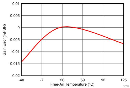
图 6-14. Gain Error vs Free-Air Temperature
