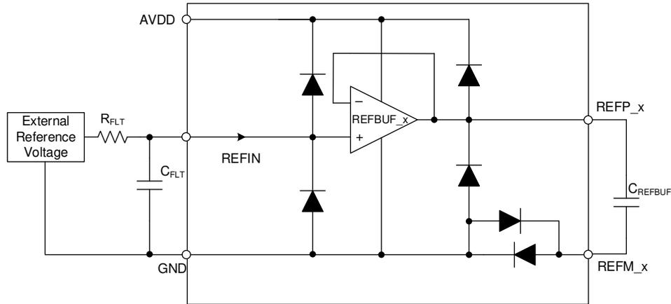
图 7-4. Connection Diagram for Reference and Reference Buffers
