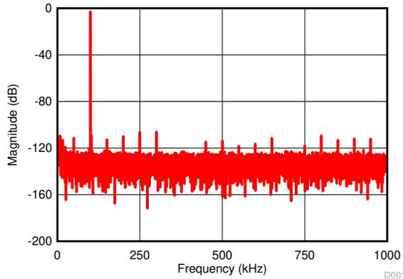
$f_{\text{IN}} = 100\text{ kHz}$ , SNR = 90.1 dB, THD = -99.3 dB
