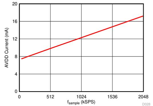
图 6-21. Dynamic AVDD Current vs Sampling Rate
