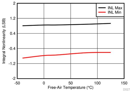
图 6-20. INL vs Free-Air Temperature
