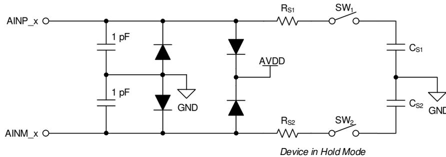
图 7-2. Analog Input Structure for Converter Module
