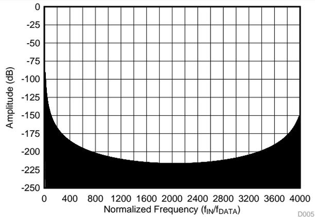
Figure 49. Sinc<sup>3</sup> Filter Frequency Response (OSR 4096)
