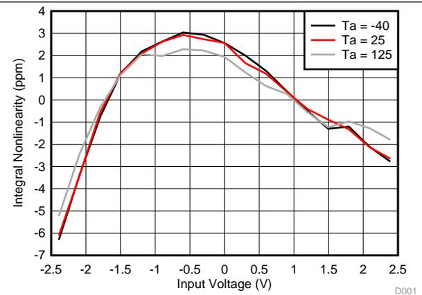
Figure 18. INL vs Temperature
