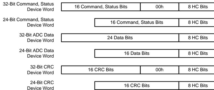
**Figure 58. Hamming Code on Each Device Word**
