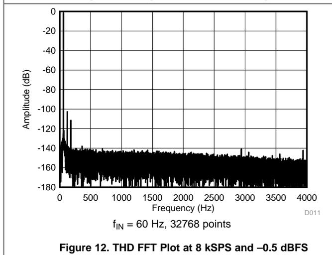
Figure 12. THD FFT Plot at 8 kSPS and  $-0.5\text{ dBFS}$
