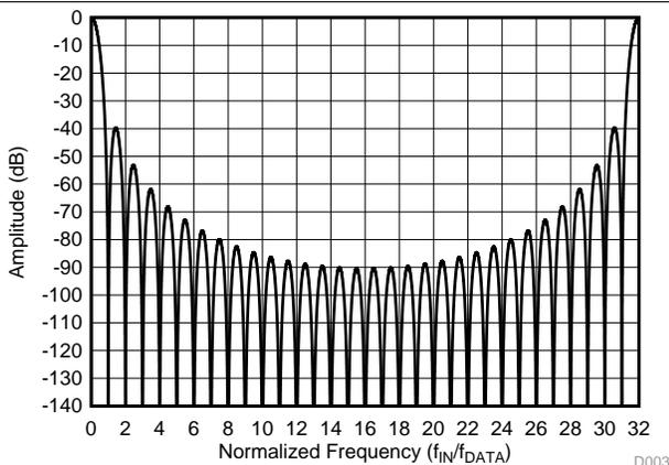
Figure 47. Sinc<sup>3</sup> Filter Frequency Response (OSR 32)
