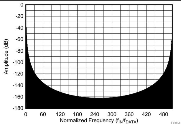
Figure 48. Sinc<sup>3</sup> Filter Frequency Response (OSR 512)
