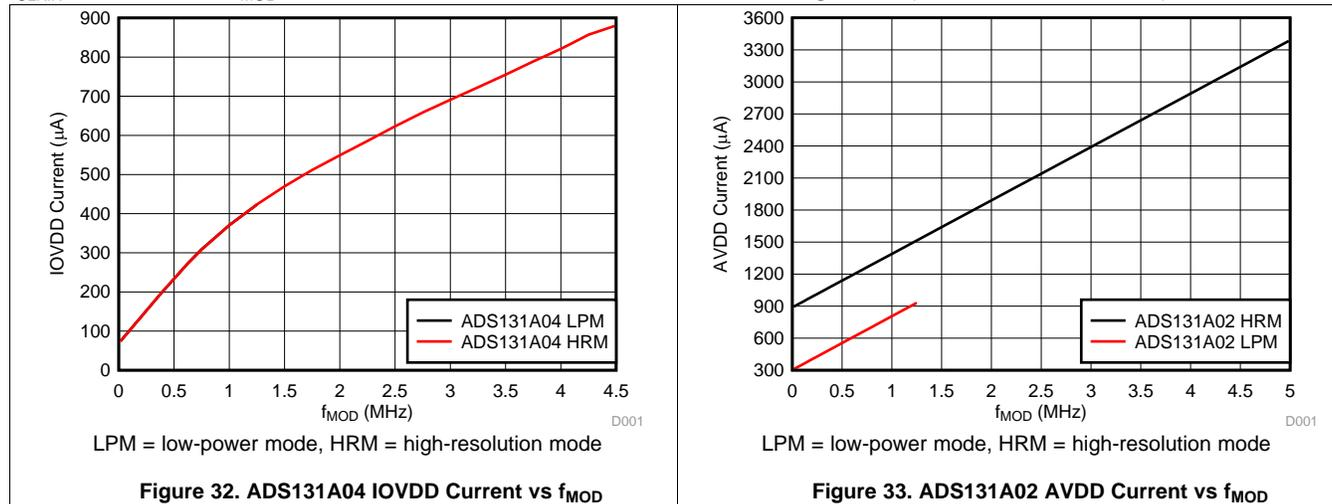
Figure 32. ADS131A04 IOVDD Current vs f<sub>MOD</sub>
