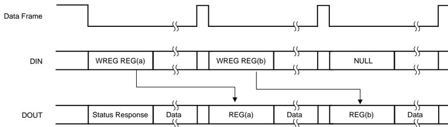
Figure 77. WREG Command Status Response (Single Register Write)
