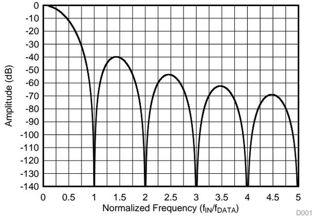
Figure 45. Sinc<sup>3</sup> Filter Frequency Response
