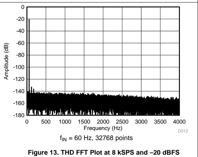
Figure 13. THD FFT Plot at 8 kSPS and  $-20\text{ dBFS}$
