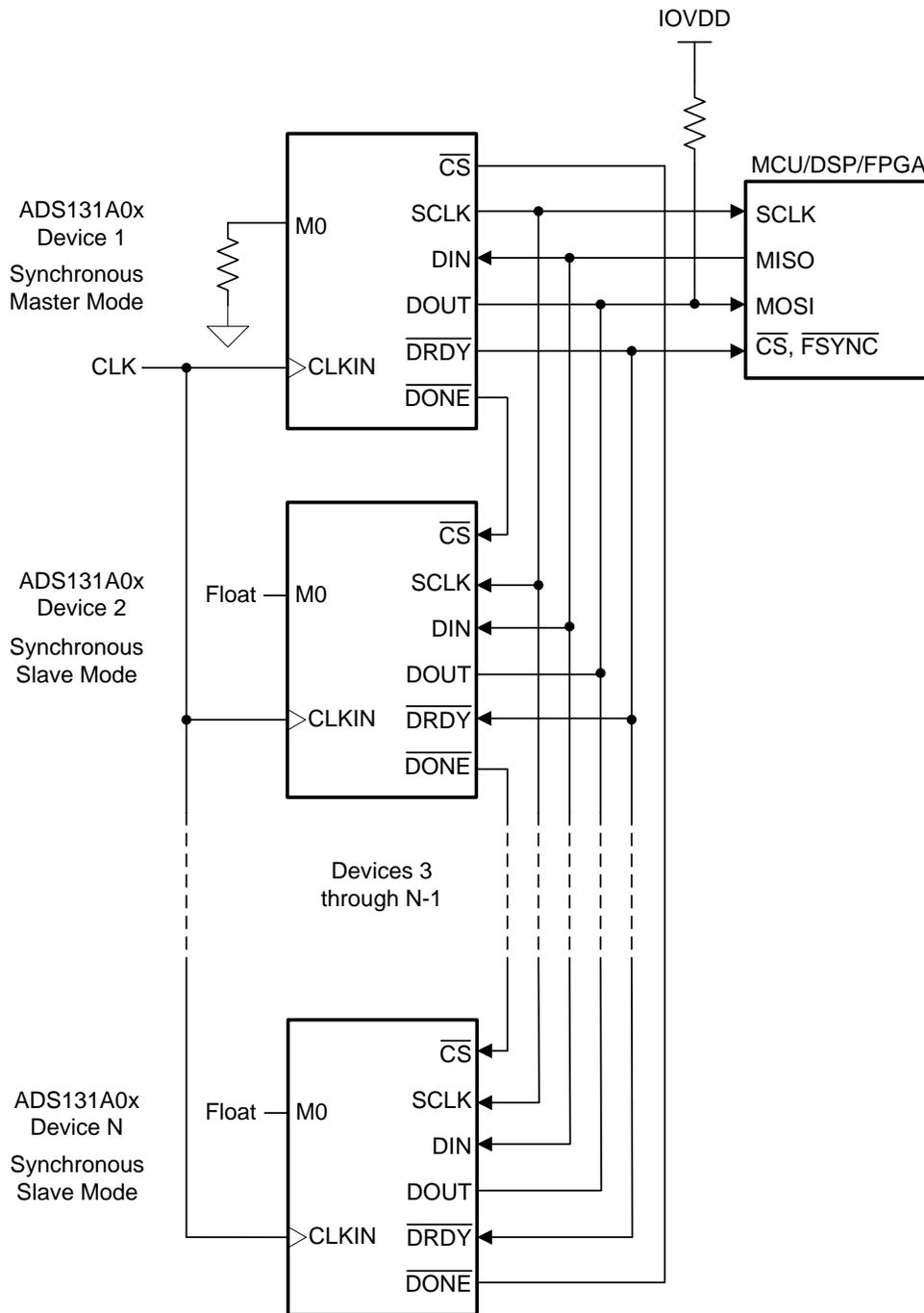
Figure 98. Multiple Device Configuration Using Synchronous Master Mode
