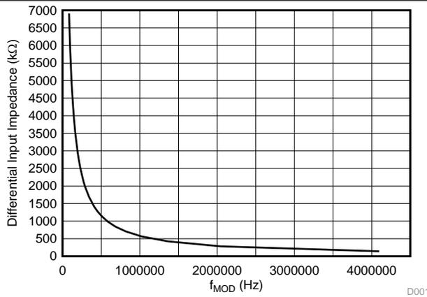
Figure 28. Differential Input Impedance vs Modulator Clock
