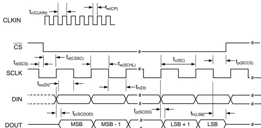
NOTE: SPI settings are CPOL = 0 and CPHA = 1.  $\overline{CS}$  can be tied directly to  $\overline{DRDY}$ .
