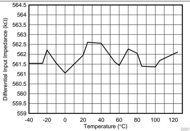
Figure 30. Differential Input Impedance vs Temperature at 1.024-MHz  $f_{\text{MOD}}$
