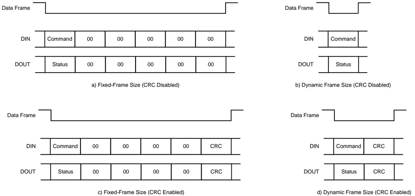
**Figure 53. Fixed versus Dynamic-Frame Modes in Standby Mode**
