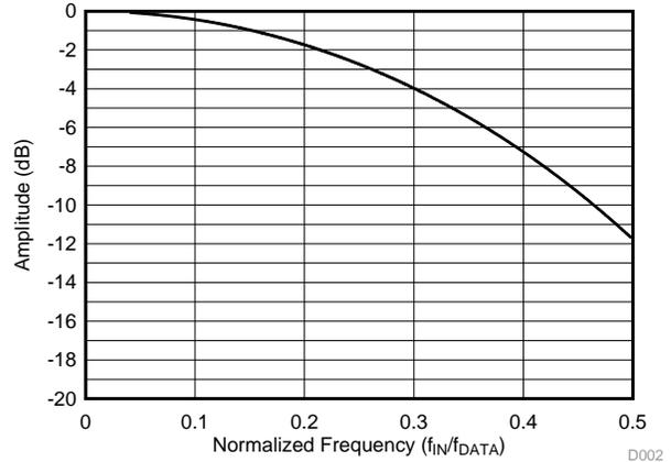
Figure 46. Sinc<sup>3</sup> Filter Roll-Off
