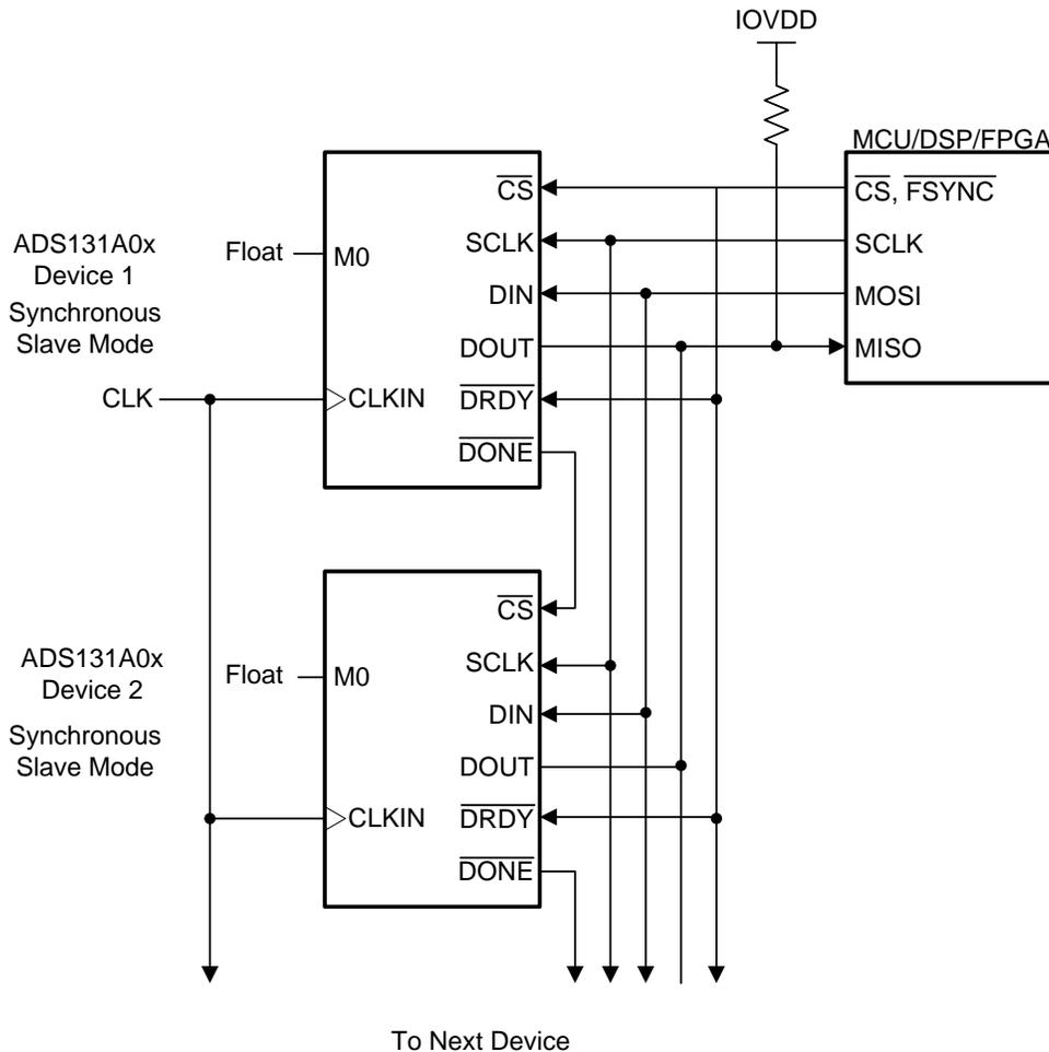
Figure 100. Multiple Device Configuration Using Synchronous Slave Mode
