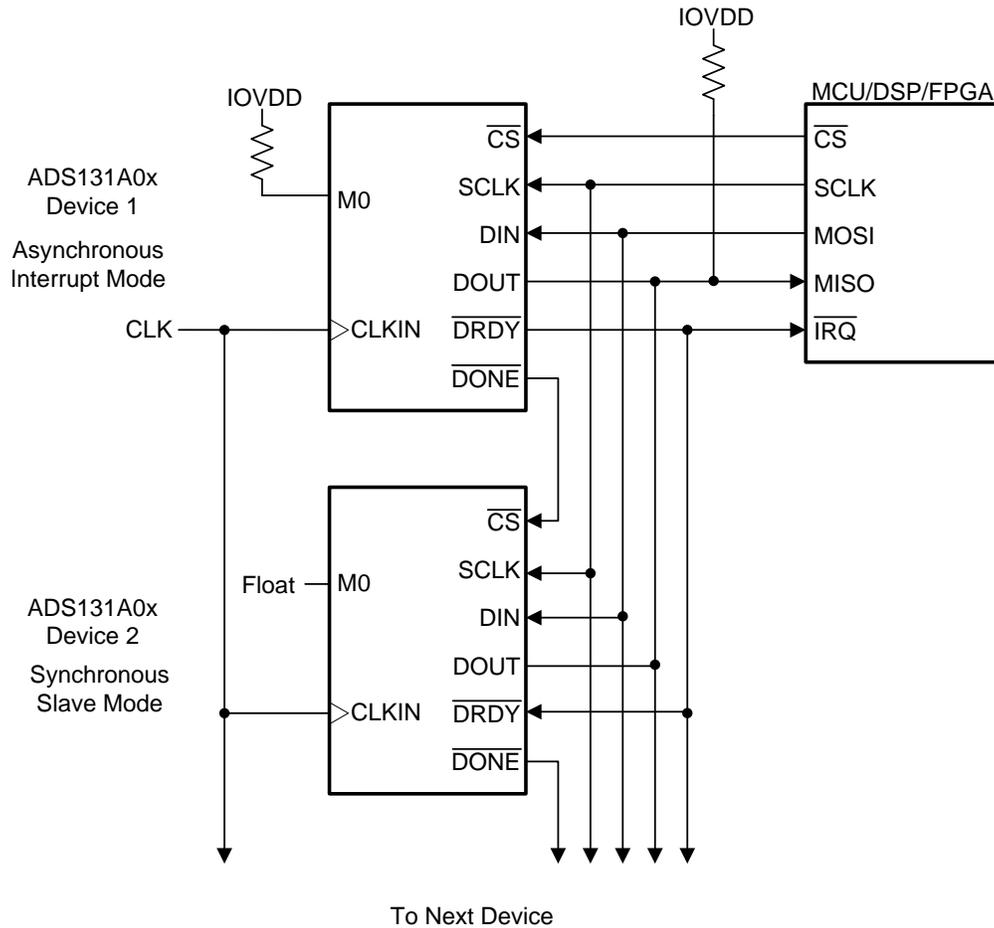
Figure 96. Multiple Device Configuration Using Asynchronous Interrupt Mode
