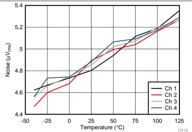
Figure 19. Noise RMS vs Temperature
