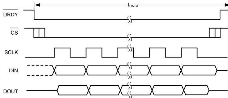
Figure 66. Data Retrieval in Synchronous Slave Mode
