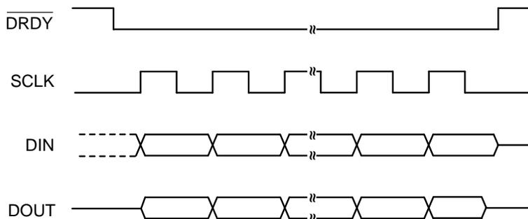
Figure 64. Data Retrieval in Synchronous Master Mode
