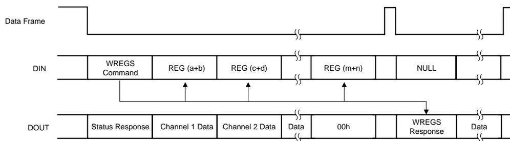
**Figure 78. WREGS Command Status Response (Multiple Register Write)**
