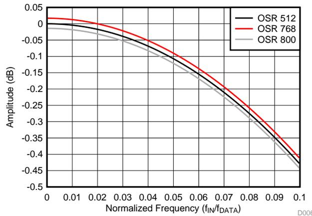
**Figure 50. Non-Binary OSR  $\text{Sinc}^3$  Filter Frequency Response**
