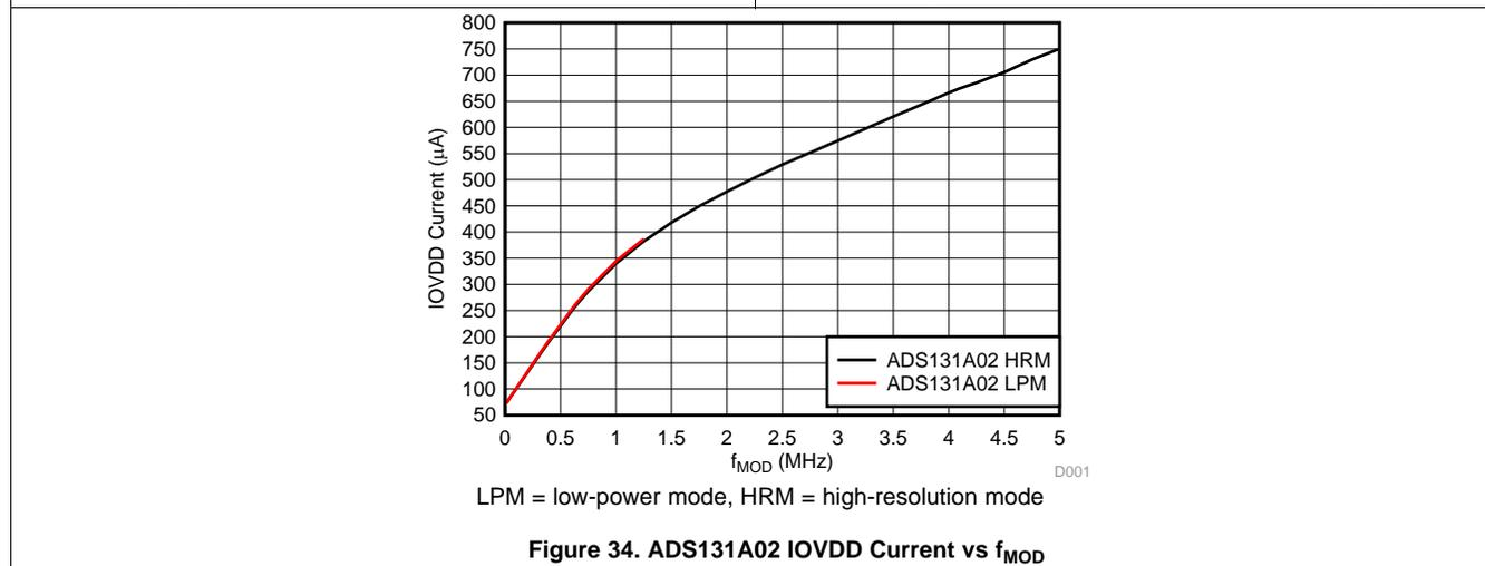
Figure 34. ADS131A02 IOVDD Current vs f<sub>MOD</sub>
