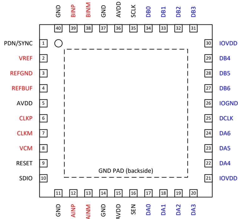
图 5-1. RSB Package, 40-Pin WQFN, Top View
