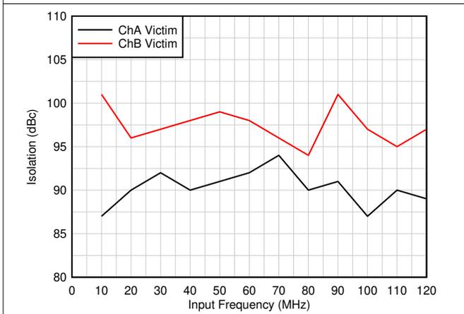
图 6-53. Isolation vs Input Frequency
