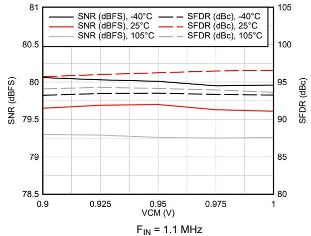
图 6-29. AC Performance vs VCM vs Temperature
