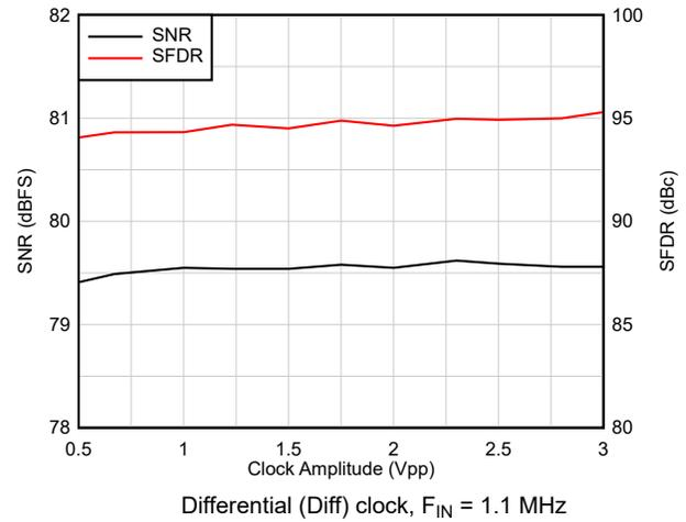
图 6-8. AC Performance vs Clock Amplitude
