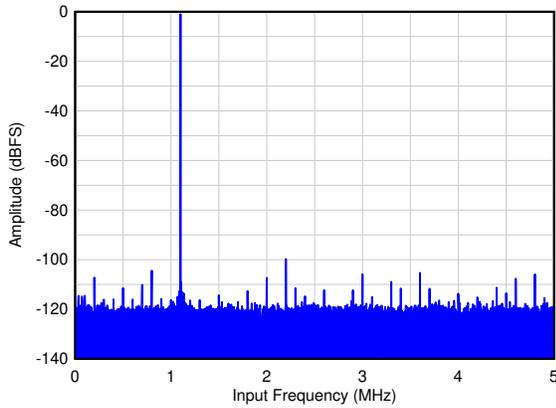
图 6-1. Single Tone FFT at  $F_{IN} = 1.1\text{ MHz}$
