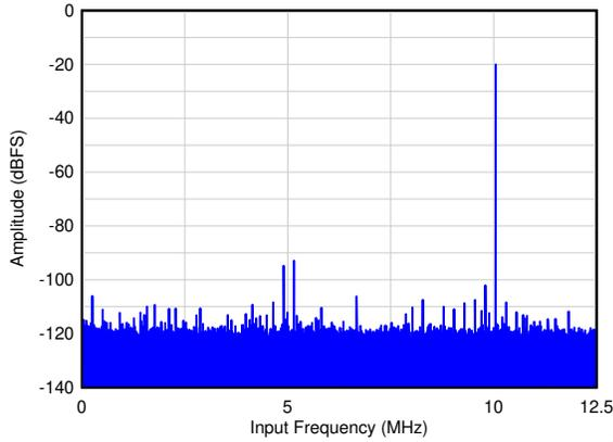
图 6-20. Single Tone FFT at  $F_{IN} = 10\text{ MHz}$
