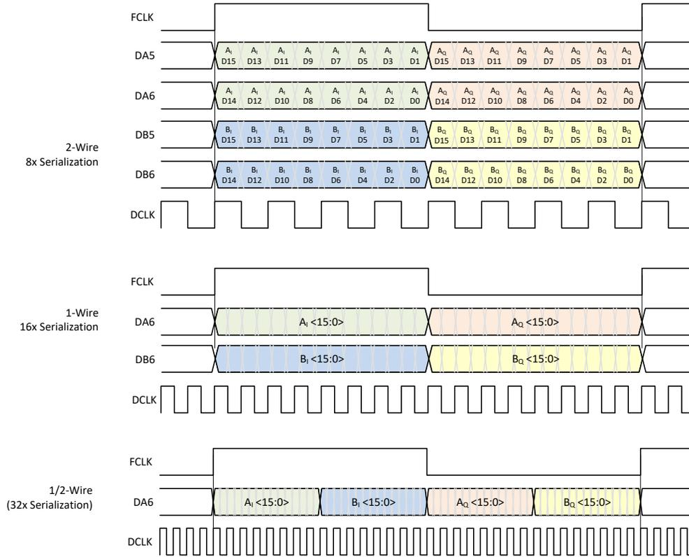
**图 8-38. Output Data Format in Complex Decimation**
