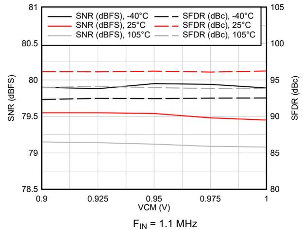
图 6-10. AC Performance vs VCM vs Temperature
