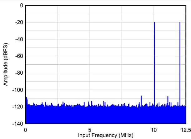
图 6-22. Two Tone FFT at  $F_{IN} = 10, 12\text{ MHz}$
