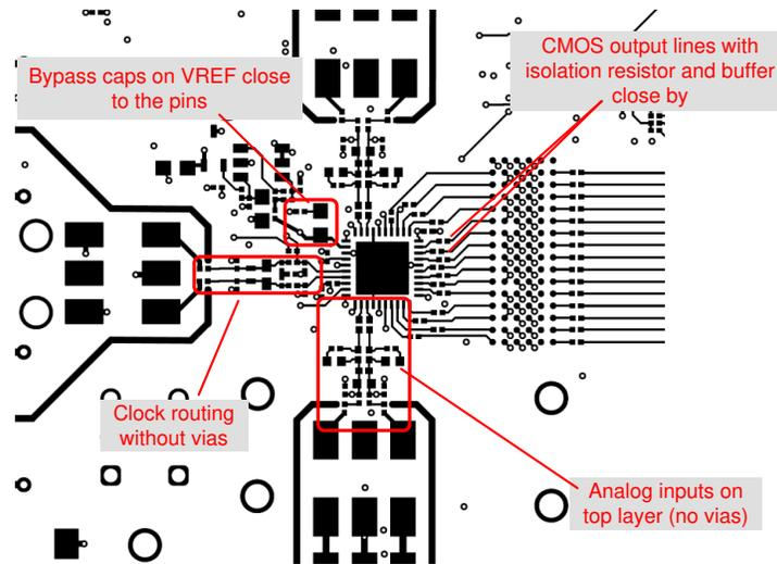
图 9-10. Layout example: top layer of ADC364x EVM
