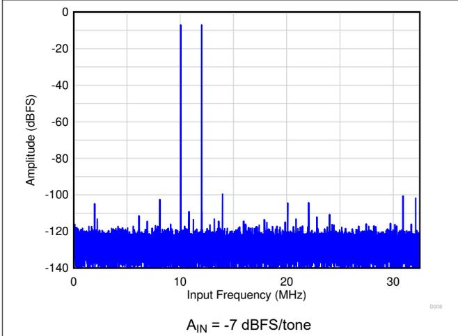
图 6-43. Two Tone FFT at  $F_{IN} = 10/12 \text{ MHz}$
