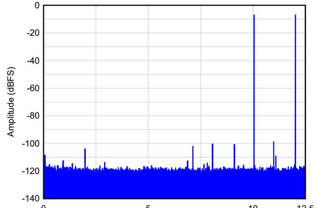
图 6-21. Two Tone FFT at  $F_{IN} = 10, 12\text{ MHz}$
