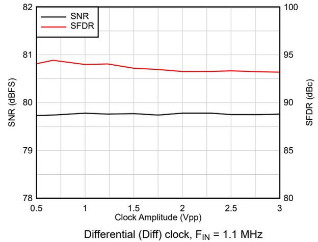
图 6-27. AC Performance vs Clock Amplitude
