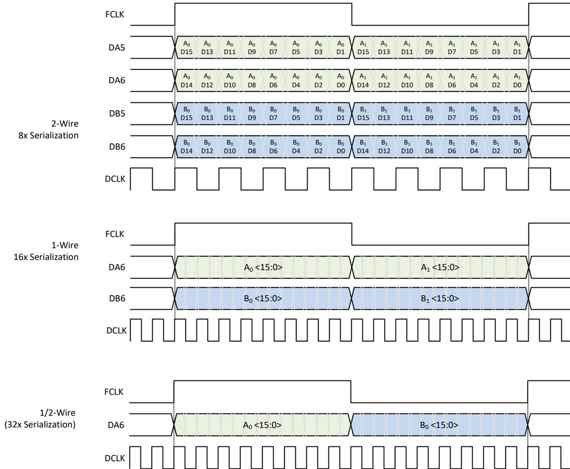
**图 8-39. Output Data Format in Real Decimation**
