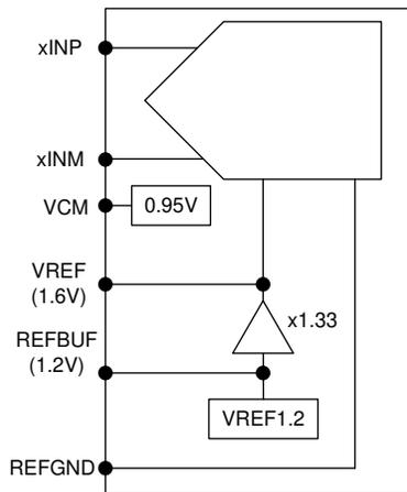
**图 8-16. Different voltage reference options for ADC364x**
