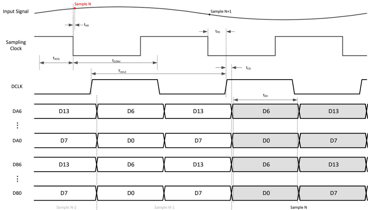
图 7-1. Timing diagram: DDR CMOS (default bit mapper)
