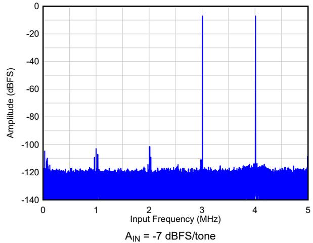
图 6-2. Two Tone FFT at  $F_{IN} = 3, 4\text{ MHz}$
