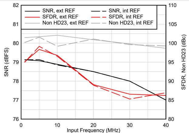
图 6-23. AC Performance vs Input Frequency
