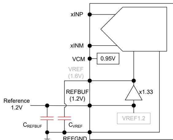
图 8-19. External 1.2V reference using internal reference buffer
