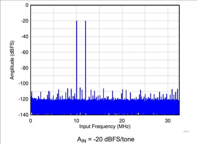
图 6-44. Two Tone FFT at  $F_{IN} = 10/12 \text{ MHz}$
