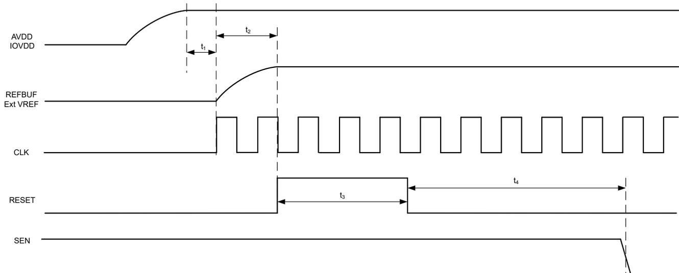
图 9-6. Initialization of serial registers after power up
