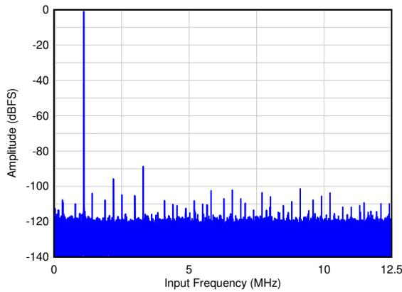
图 6-18. Single Tone FFT at  $F_{IN} = 1.1\text{ MHz}$
