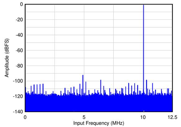
图 6-19. Single Tone FFT at  $F_{IN} = 10\text{ MHz}$
