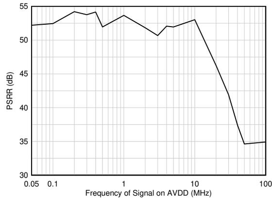
**图 9-7. Power supply rejection ratio (PSRR) vs frequency**
