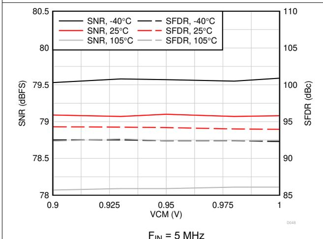
图 6-51. AC Performance vs VCM vs Temperature
