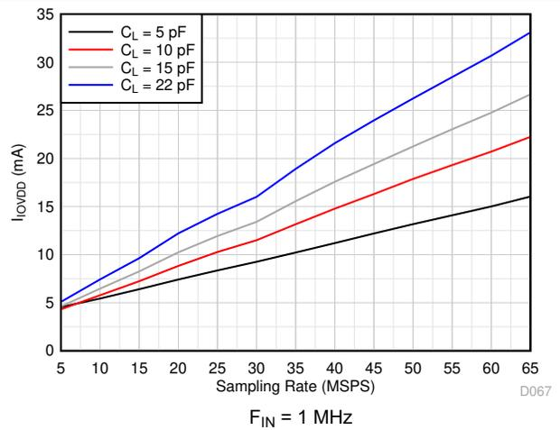
图 6-60. I\_OVDD Current vs Load Capacitance
