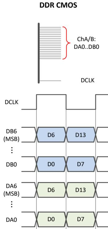
**图 8-37. Output Data Format in Real Decimation**
