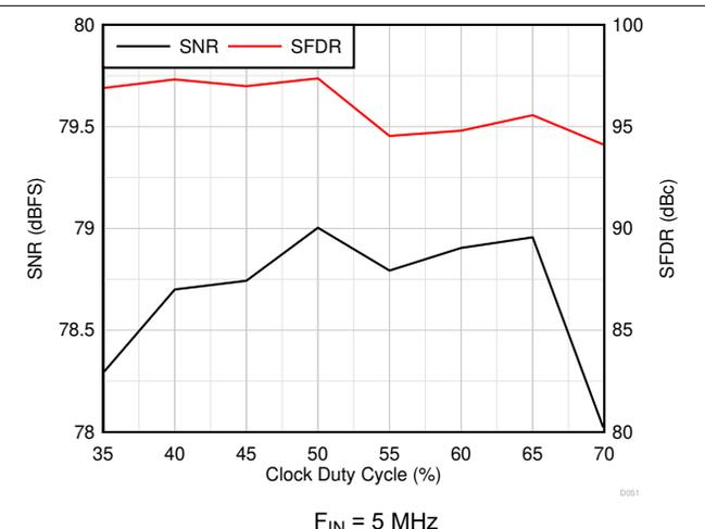
图 6-52. AC Performance vs Clock Duty Cycle
