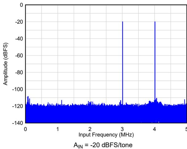
图 6-3. Two Tone FFT at  $F_{IN} = 3, 4\text{ MHz}$
