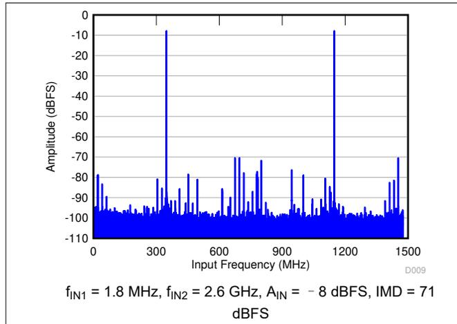
图 6-23. FFT for Two-Tone Input Signal (-8 dBFS)
