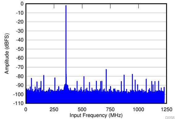
SNR = 57.5 dBFS; SFDR = 70 dBc; HD2 = -70 dBc; HD3 = -81 dBc; non HD2, HD3 = 75 dBc; IL spur = 77 dBc;  $f_{IN}$  = 2.1 GHz
