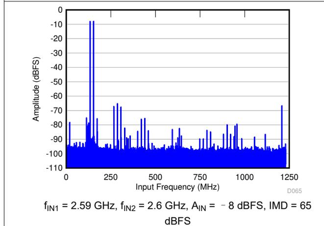
图 6-29. FFT for Two-Tone Input Signal (-8 dBFS,  $f_s = 2457.6$  MSPS)
