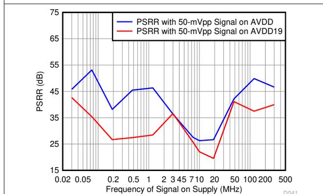
图 6-65. Power-Supply Rejection Ratio vs. Tone Frequency
