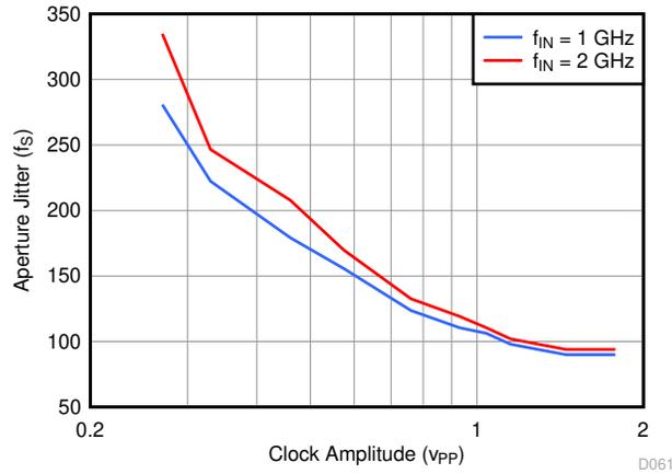
图 8-9. Equivalent Aperture Jitter vs. Input Clock Amplitude
