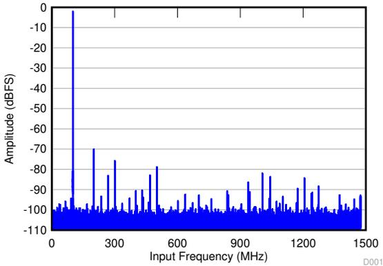
SNR = 62.2 dBFS; SFDR = 68 dBc; HD2 = -68 dBc; HD3 = -73 dBc; non HD2, HD3 = 77 dBc; IL spur = 86 dBc;  $f_{IN}$  = 100 MHz
