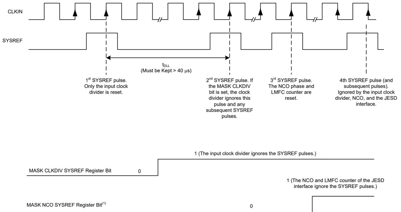
Alternatively, the SYSREF buffer can be powered down with the PDN SYSREF bit.
