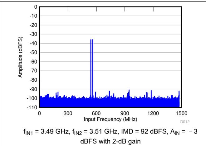
图 6-28. FFT for Two-Tone Input Signal (-36 dBFS)
