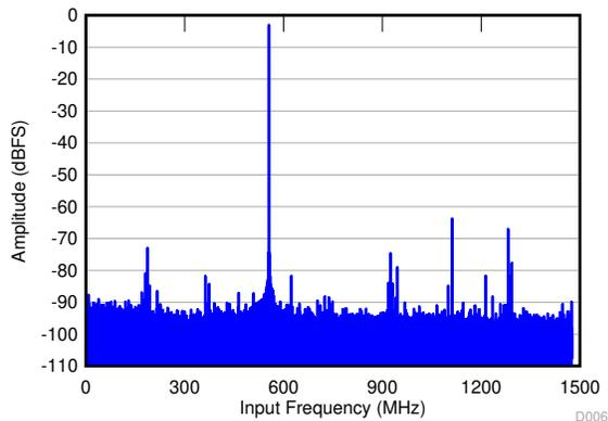
SNR = 54.2 dBFS; SFDR = 60 dBc; HD2 = -60 dBc; HD3 = -64 dBc; non HD2, HD3 = 71 dBc; IL spur = 80 dBc;  $f_{IN}$  = 3.5 GHz,  $A_{IN}$  = -3 dBFS with 2-dB gain
