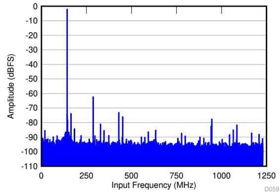
SNR = 55.4 dBFS; SFDR = 60 dBc; HD2 = -60 dBc; HD3 = -67 dBc; non HD2, HD3 = 72 dBc; IL spur = 75 dBc;  $f_{IN}$  = 2.6 GHz
