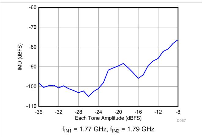
图 6-32. Intermodulation Distortion vs. Input Amplitude (1770 MHz and 1790 MHz,  $f_s = 2457.6$  MSPS)
