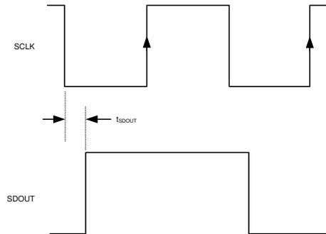
**图 8-57. SDOUT Timing**
