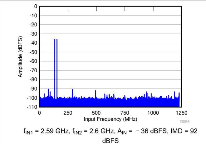
图 6-30. FFT for Two-Tone Input Signal (-36 dBFS,  $f_s = 2457.6$  MSPS)
