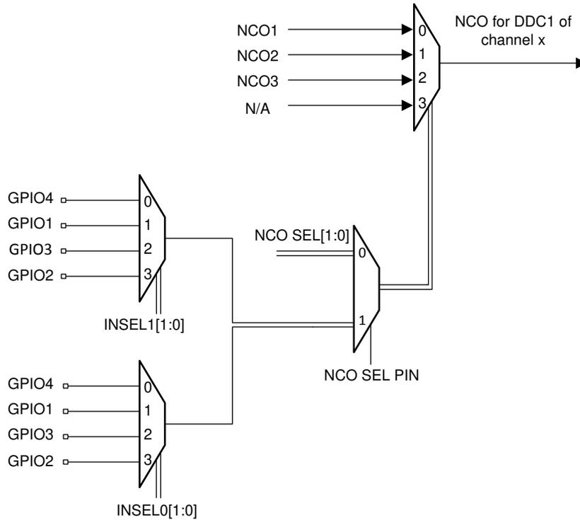
图 8-42. NCO Switching from GPIO and SPI
