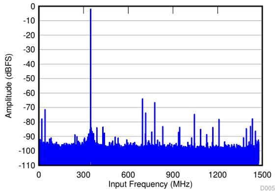
SNR = 56.9 dBFS; SFDR = 62 dBc; HD2 = -62 dBc; HD3 = -72 dBc; non HD2, HD3 = 72 dBc; IL spur = 64 dBc;  $f_{IN}$  = 2.6 GHz
