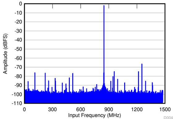
SNR = 58.2 dBFS; SFDR = 64 dBc; HD2 = -64 dBc; HD3 = -85 dBc; non HD2, HD3 = 73 dBc; IL spur = 74 dBc;  $f_{IN}$  = 2.1 GHz
