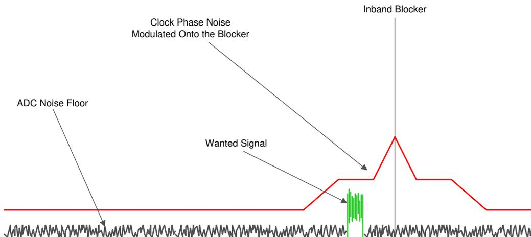
图 9-4. Small Wanted Signal in Presence of Interferer
