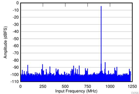
SNR = 62.1 dBFS; SFDR = 76 dBc; HD2 = -76 dBc; HD3 = -83 dBc; non HD2, HD3 = 82 dBc; IL spur = 83 dBc;  $f_{IN}$  = 900 MHz
