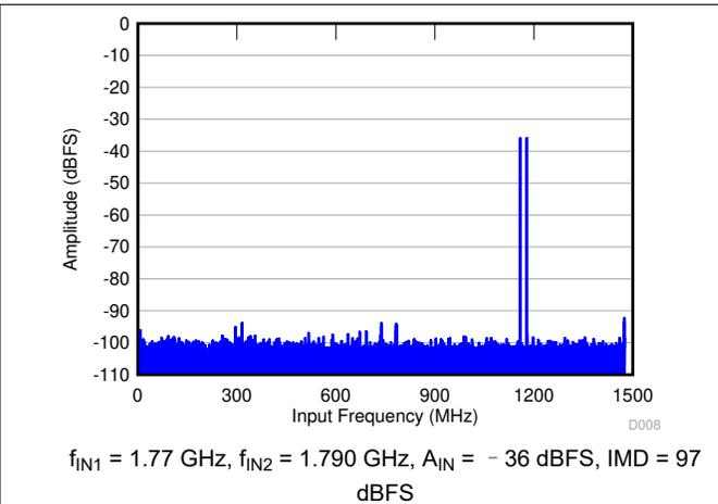
图 6-20. FFT for Two-Tone Input Signal (-36 dBFS)
