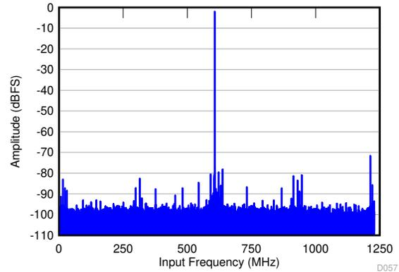
SNR = 58 dBFS; SFDR = 69 dBc; HD2 = -69 dBc; HD3 = -75 dBc; non HD2, HD3 = 74 dBc; IL spur = 78 dBc;  $f_{IN}$  = 1.85 GHz
