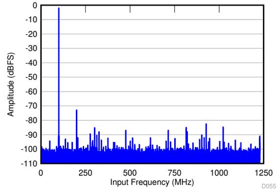
SNR = 62.4 dBFS; SFDR = 71 dBc; HD2 = -71 dBc; HD3 = -83 dBc; non HD2, HD3 = 82 dBc; IL spur = 80 dBc;  $f_{IN}$  = 100 MHz
