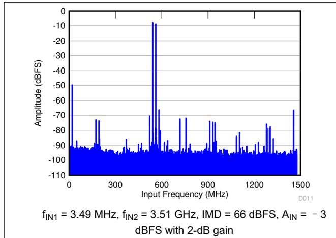
图 6-27. FFT for Two-Tone Input Signal (-8 dBFS)
