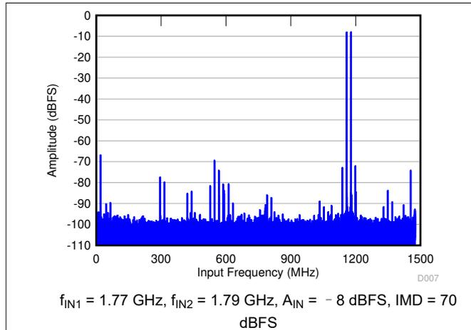
图 6-19. FFT for Two-Tone Input Signal (-8 dBFS)
