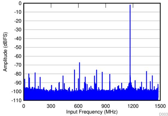
SNR = 59.1 dBFS; SFDR = 65 dBc; HD2 = -65 dBc; HD3 = -73 dBc; non HD2, HD3 = 73 dBc; IL spur = 76 dBc;  $f_{IN}$  = 1.7 GHz
