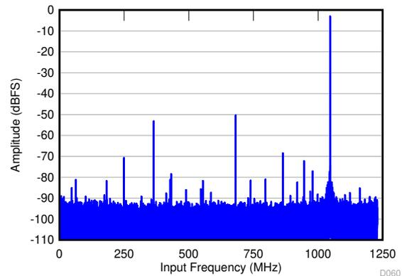
SNR = 53.6 dBFS; SFDR = 47 dBc; HD2 = -50 dBc; HD3 = -47 dBc; non HD2, HD3 = 70 dBc; IL spur = 67 dBc;  $f_{IN}$  = 3.5 GHz,  $A_{IN}$  = -3 dBFS with 2-dB gain
