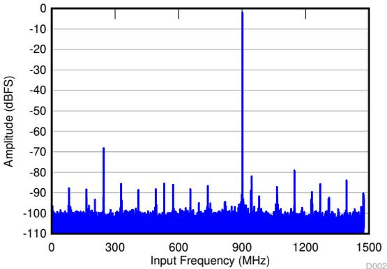
SNR = 61.2 dBFS; SFDR = 66 dBc; HD2 = -77 dBc; HD3 = -66 dBc; non HD2, HD3 = 80 dBc; IL spur = 83 dBc;  $f_{IN}$  = 900 MHz
