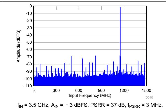
图 6-64. Power-Supply Rejection Ratio FFT for Test Signal on AVDD Supply
