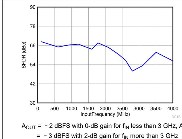
图 6-37. Spurious-Free Dynamic Range vs. Input Frequency
