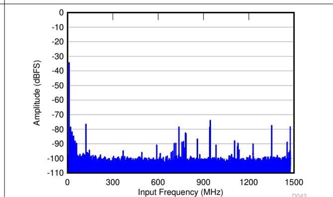
图 6-66. Common-Mode Rejection Ratio FFT
