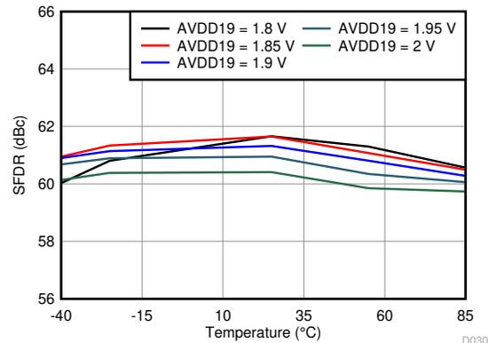
$f_{IN} = 3.5 \text{ GHz}$ ,  $A_{IN} = -3 \text{ dBFS}$  with 2-dB digital gain
