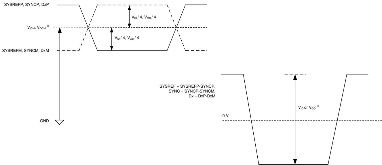
A.  $V_{OCM}$  is not the same as  $V_{ICM}$ . Similarly,  $V_{OD}$  is not the same as  $V_{ID}$ .
