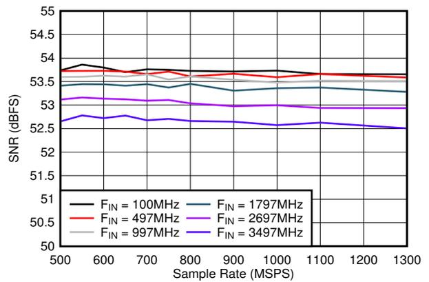
图 7-22. SNR vs Sample Rate
