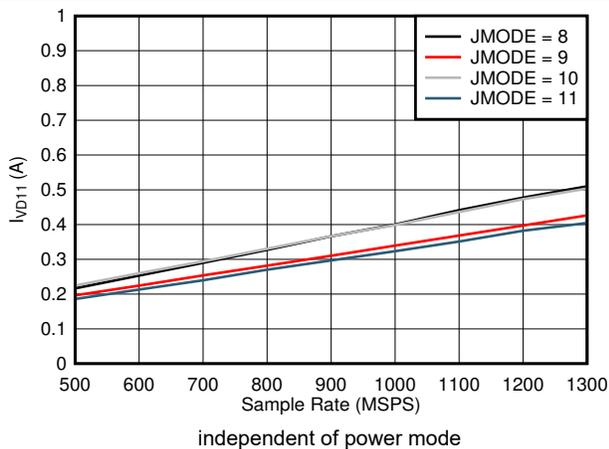
图 7-89. Quad Channel,  $I_{VD11}$  vs FS and JMODE 8 - 11
