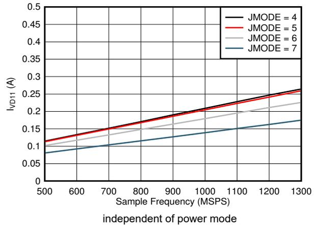
图 7-108. Single Channel,  $I_{VD11}$  vs FS and JMODE 4 - 7
