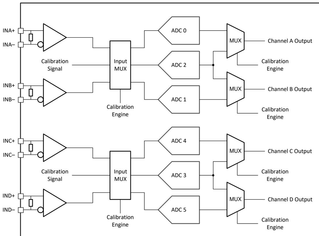
**图 8-15. Quad Channel Calibration System Block Diagram**
