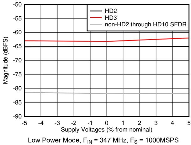
图 7-47. HD2, HD3 and Worst non-HD Spur vs Supply Voltage
