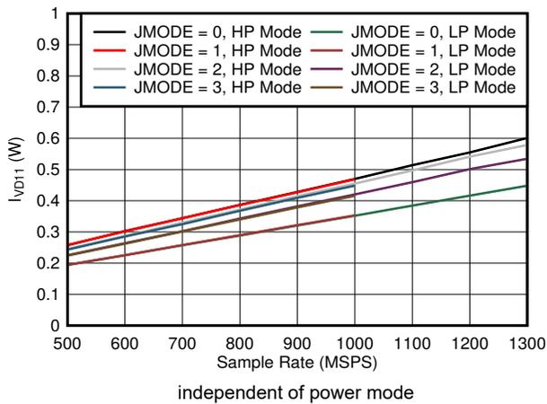
图 7-87. Quad Channel,  $I_{VD11}$  vs FS and JMODE 0 - 3
