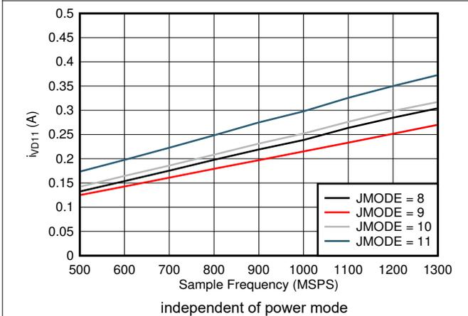
图 7-99. Dual Channel,  $I_{VD11}$  vs FS and JMODE 8 - 11
