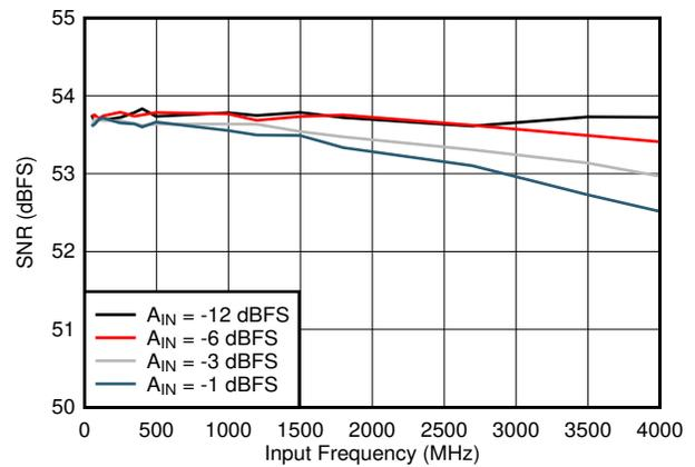
图 7-16. SNR vs Input Frequency
