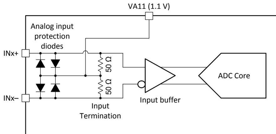
图 8-4. Analog Input Internal Termination and Protection Diagram
