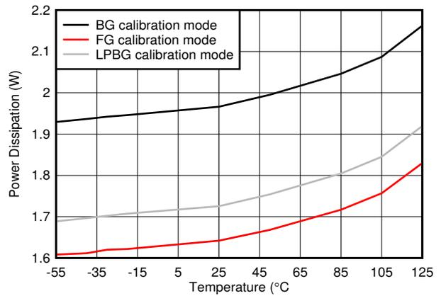
**图 7-124. Dual Channel, Power Dissipation vs Temperature**
