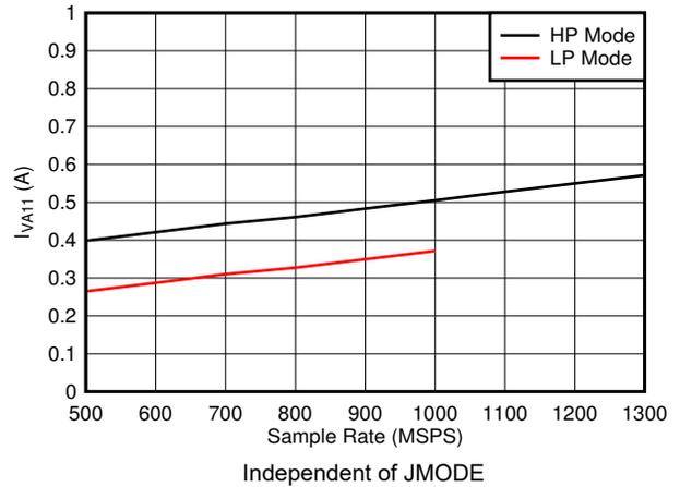
图 7-86. Quad Channel,  $I_{VA11}$  vs FS
