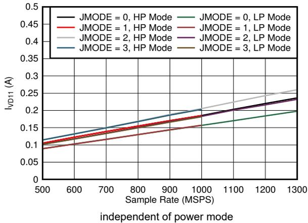
图 7-107. Single Channel,  $I_{VD11}$  vs FS and JMODE 0 - 3
