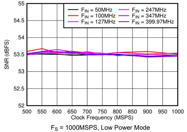
图 7-26. SNR vs Sample Rate
