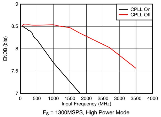
图 7-64. ENOB vs Input Frequency and CPLL
