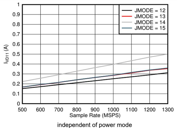
图 7-90. Quad Channel,  $I_{VD11}$  vs FS and JMODE 12 - 15
