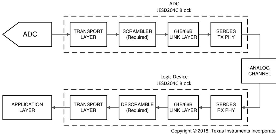
图 8-8. Simplified 64B/66B Encoded JESD204C Interface Diagram
