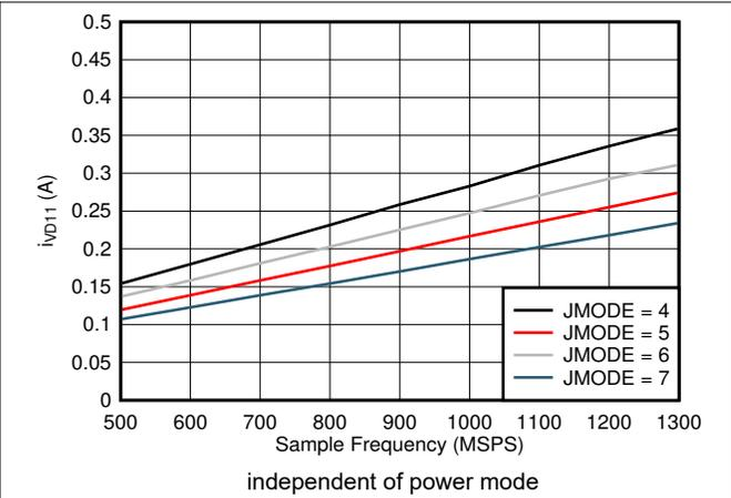
图 7-98. Dual Channel,  $I_{VD11}$  vs FS and JMODE 4 - 7
