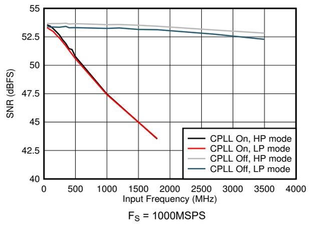
图 7-66. SNR vs Input Frequency and CPLL
