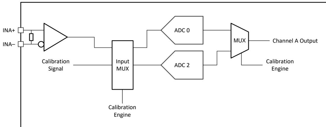
**图 8-17. Single Channel Calibration System Block Diagram**
