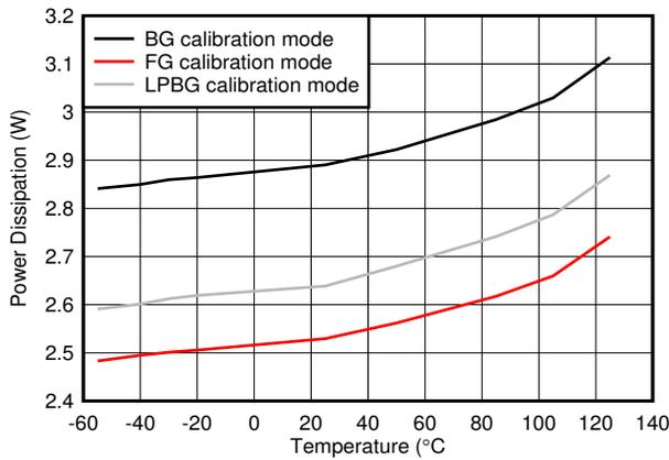
**图 7-123. Quad Channel, Power Dissipation vs Temperature**
