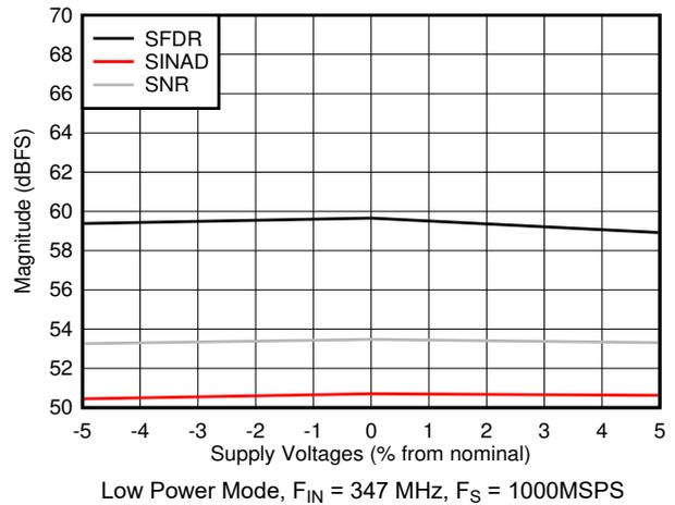
图 7-46. SNR, SFDR and SINAD vs Supply Voltage
