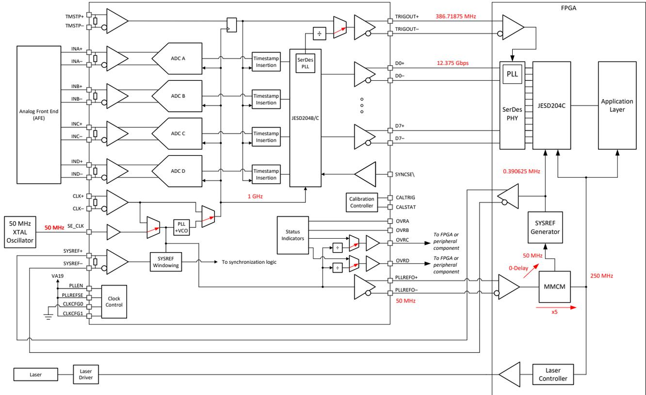
图 9-1. Typical Configuration for a LiDAR Digitizer
