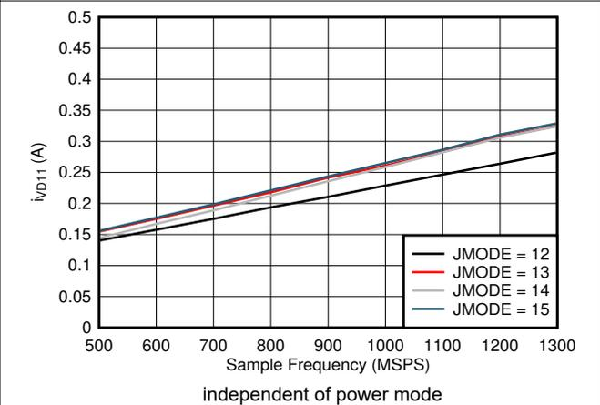
图 7-100. Dual Channel,  $I_{VD11}$  vs FS and JMODE 12 - 15
