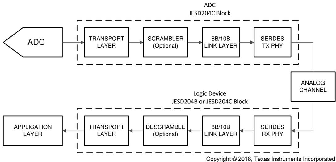
图 8-7. Simplified 8B/10B Encoded JESD204C Interface Diagram
