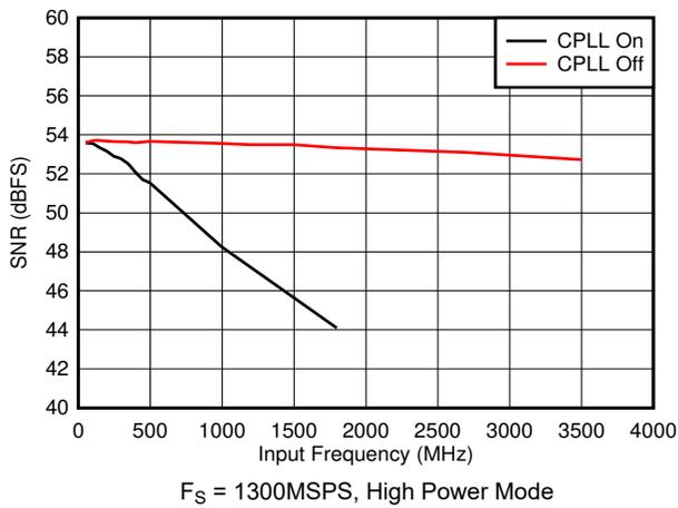
图 7-63. SNR vs Input Frequency and CPLL
