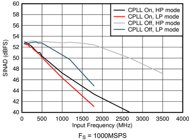
图 7-67. SINAD vs Input Frequency and CPLL
