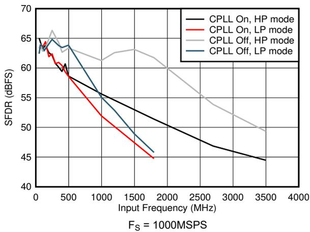
图 7-65. SFDR vs Input Frequency and CPLL
