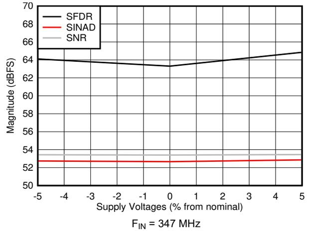
图 7-44. SNR, SFDR and SINAD vs Supply Voltage
