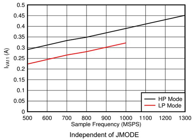
图 7-96. Dual Channel,  $I_{VA11}$  vs FS
