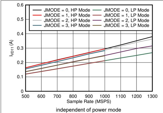
图 7-97. Dual Channel,  $I_{VD11}$  vs FS and JMODE 0 - 3
