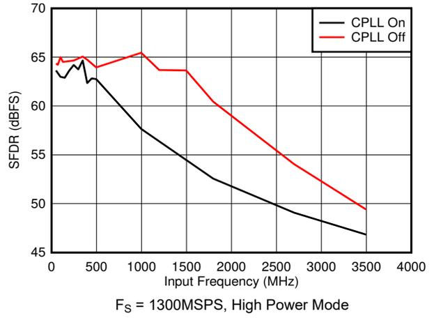
图 7-62. SFDR vs Input Frequency and CPLL
