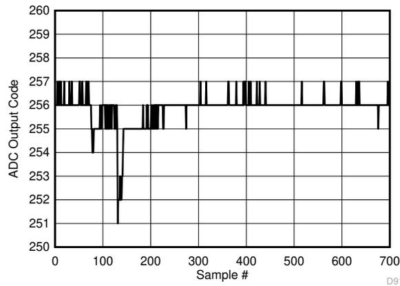
**图 7-129. Background Calibration Core Transition (DC Signal)**
