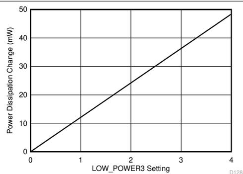
图 8-13. Power Dissipation Change vs LOW\_POWER3 register setting
