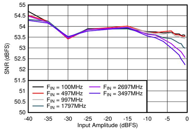
图 7-30. SNR vs Input Amplitude
