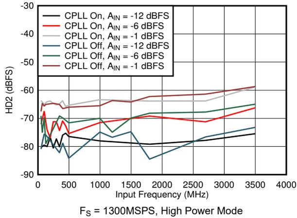
图 7-73. HD2 vs Input Frequency, CPLL and Input Amplitude
