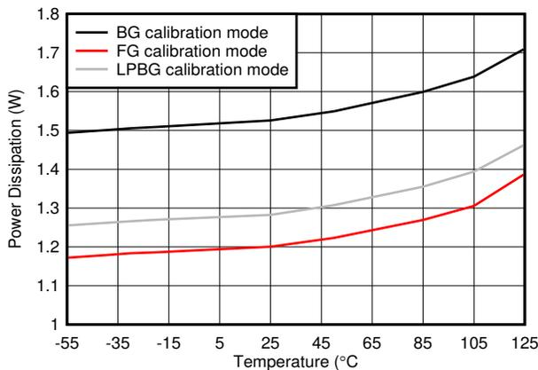
**图 7-125. Single Channel, Power Dissipation vs Temperature**
