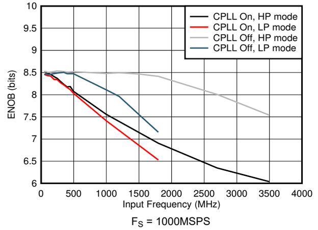
图 7-68. ENOB vs Input Frequency and CPLL
