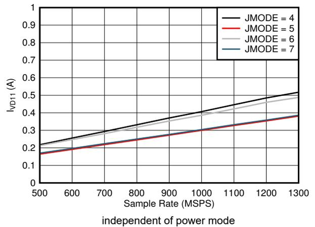
图 7-88. Quad Channel,  $I_{VD11}$  vs FS and JMODE 4 - 7
