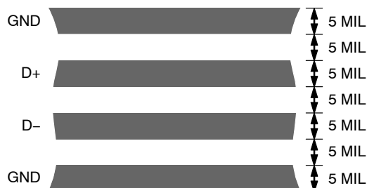
Figure 22. Typical Arrangement of Signal Tracks
