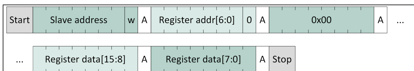
Figure 20 I2C Single Write Access
