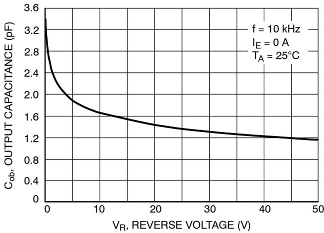
Figure 4. Output Capacitance
