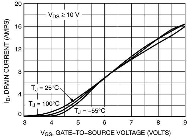
**Figure 2. Transfer Characteristics**
