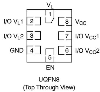
Figure 2. Pin-out Diagram
