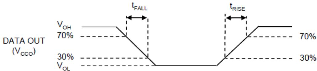
Figure 5. Definition of Rise and Fall Times
