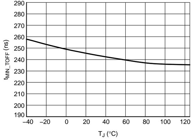
Figure 27. Minimum Off-time R<sub>MIN\_TOFF</sub> = 0 Ω
