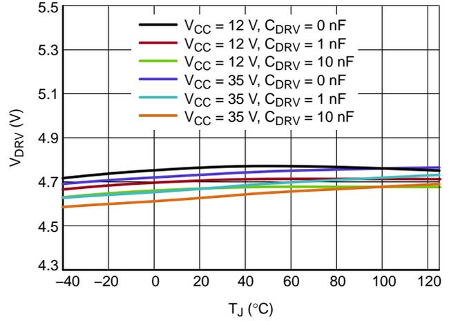
Figure 33. Driver Output Voltage, ver. A and C
