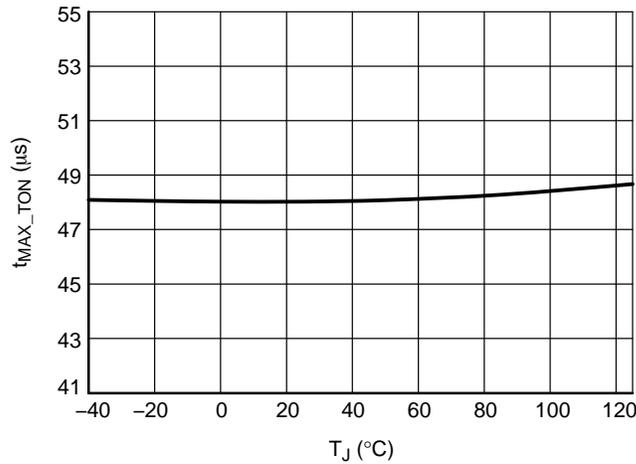
Figure 36. Maximum On-time,  $V_{MAX\_TON} = 0.3 V$ , ver. Q
