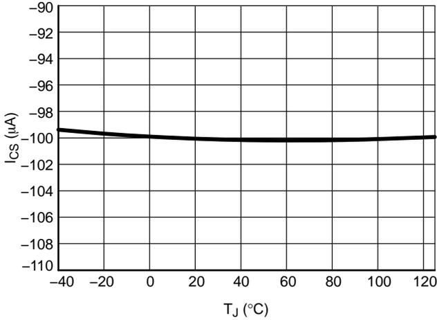
Figure 14. CS Current,  $V_{CS} = -20$  mV
