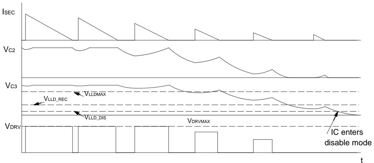
**Figure 55. NCP43080 Driver Clamp Modulation Waveforms in Flyback Application Entering into Light/No Load Condition**
