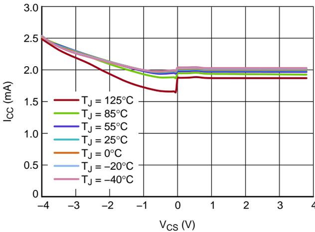
Figure 16. Supply Current vs. CS Voltage,  $V_{CC} = 12$  V
