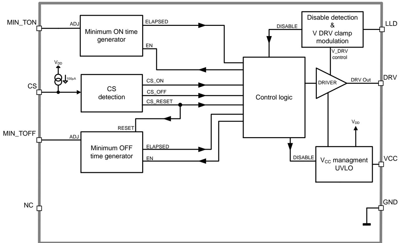
Figure 5. Internal Circuit Architecture – NCP43080A, B, C, D
