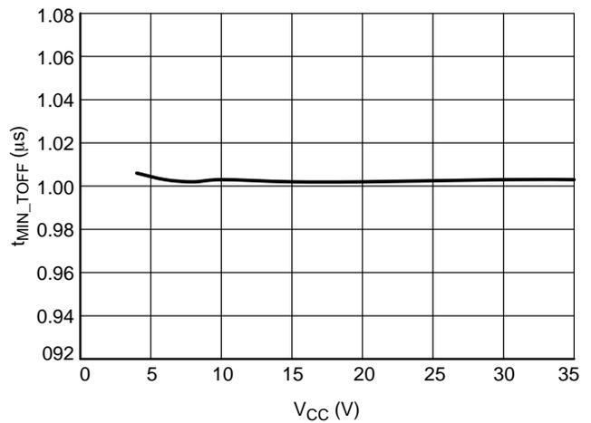
Figure 31. Minimum Off-time R<sub>MIN\_TOFF</sub> = 10 kΩ
