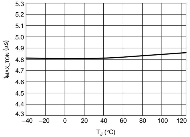
Figure 35. Maximum On-time,  $V_{MAX\_TON} = 3 V$ , ver. Q
