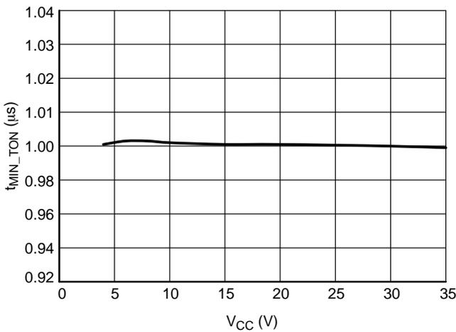
Figure 30. Minimum On-time R<sub>MIN\_TON</sub> = 10 kΩ
