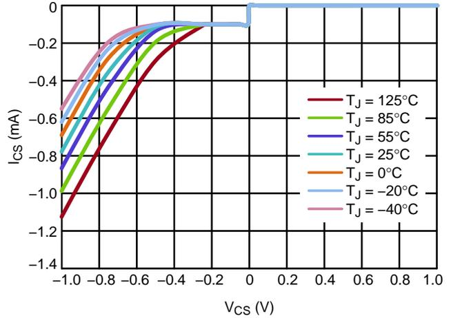
Figure 15. CS Current,  $V_{CC} = 12$  V
