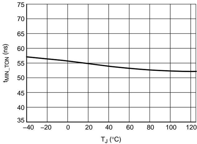
Figure 24. Minimum On-time R<sub>MIN\_TON</sub> = 0 Ω
