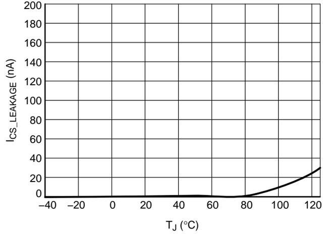
Figure 21. CS Leakage, V<sub>CS</sub> = 150 V
