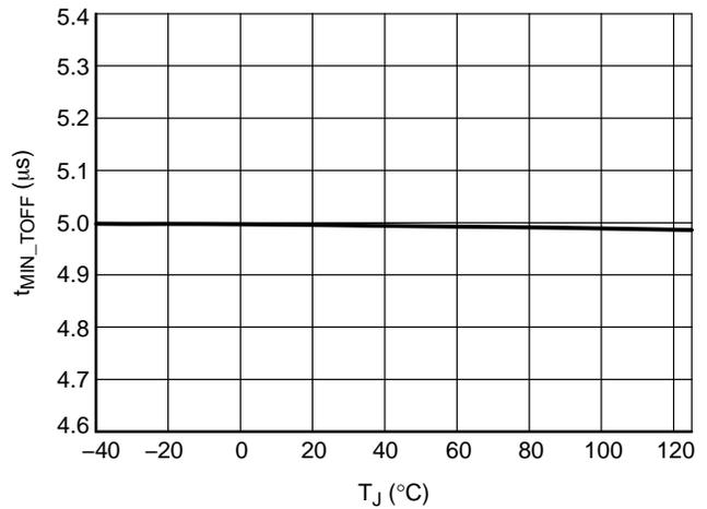
Figure 29. Minimum Off-time R<sub>MIN\_TOFF</sub> = 50 kΩ
