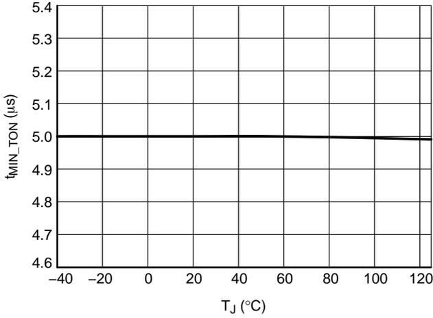
Figure 26. Minimum On-time R<sub>MIN\_TON</sub> = 50 kΩ
