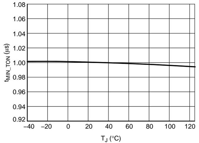
Figure 25. Minimum On-time R<sub>MIN\_TON</sub> = 10 kΩ
