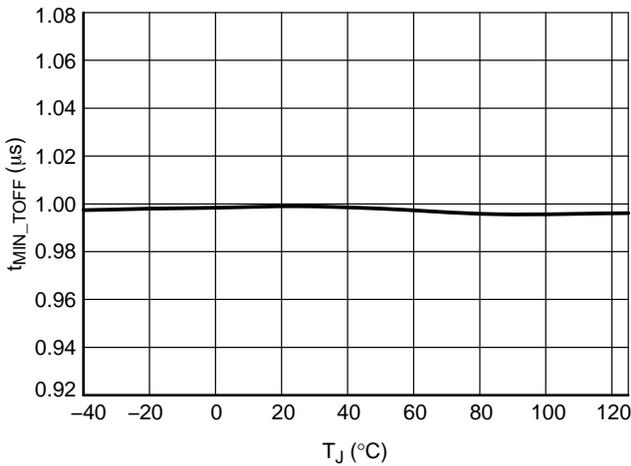
Figure 28. Minimum Off-time R<sub>MIN\_TOFF</sub> = 10 kΩ
