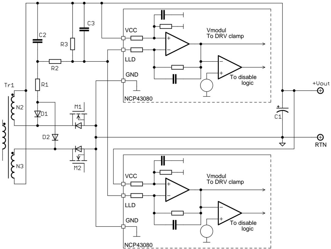
**Figure 57. NCP43080 Light Load Detection in LLC Topology**
