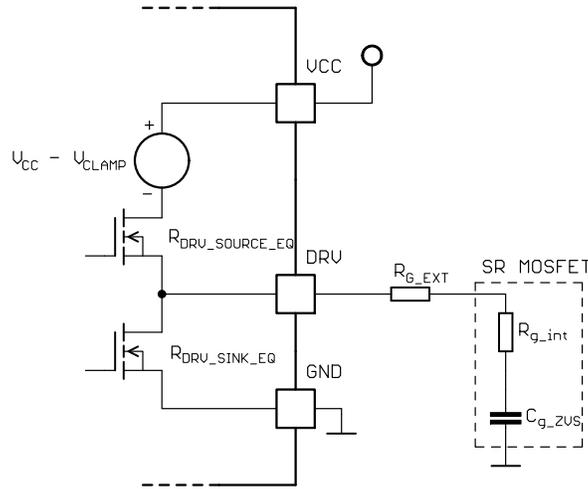
**Figure 63. Equivalent Schematic of Gate Drive Circuitry**
