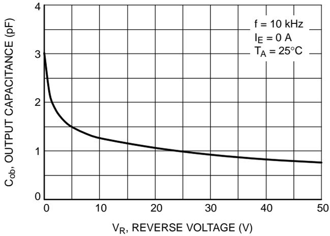
Figure 4. Output Capacitance
