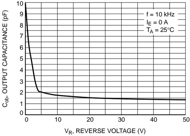
Figure 9. Output Capacitance
