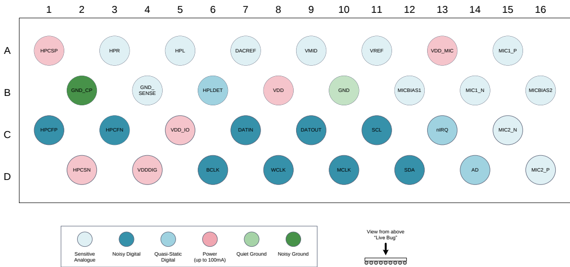
Figure 3: DA7218 Ballout Diagram
