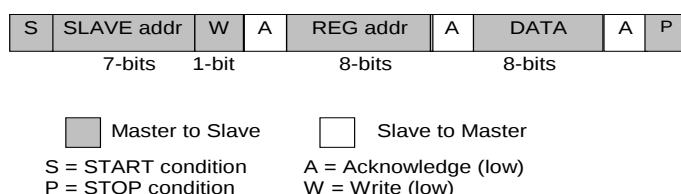
Figure 27: I 2 C Byte Write (SDA signal)
