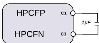
Figure 41: Charge Pump Flying Capacitor
