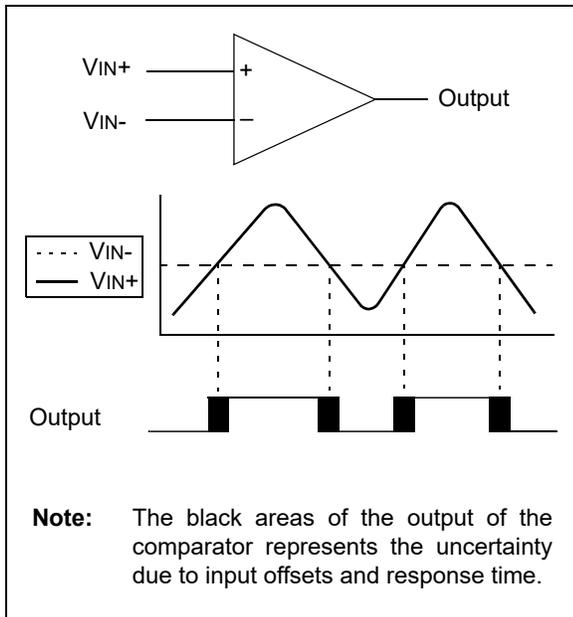
**FIGURE 18-2: COMPARATOR MODULE SIMPLIFIED BLOCK DIAGRAM**
