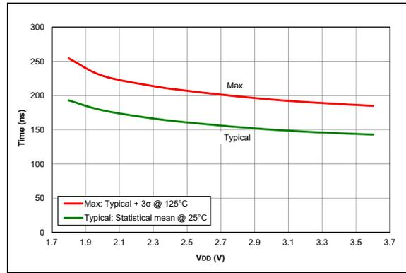
**FIGURE 36-86:** Comparator Response Time Falling edge, PIC16LF18325/18345 Only
