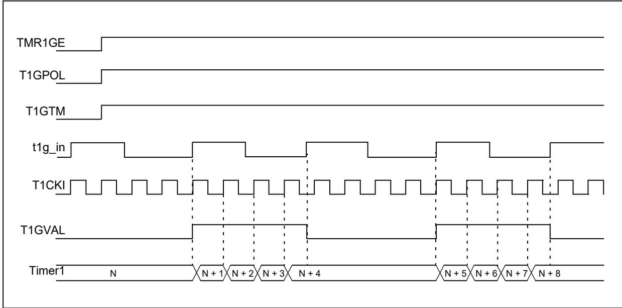
**FIGURE 27-5: TIMER1 GATE SINGLE-PULSE MODE**
