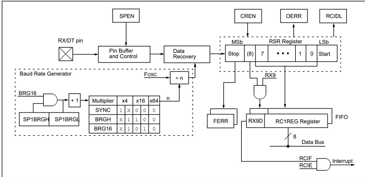
The operation of the EUSART1 module is controlled through three registers:
