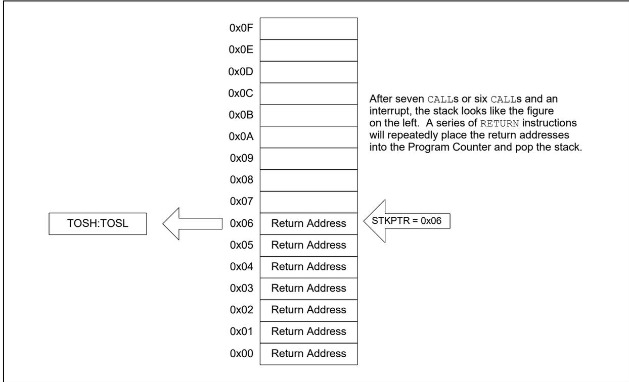
**FIGURE 4-7: ACCESSING THE STACK EXAMPLE 4**
