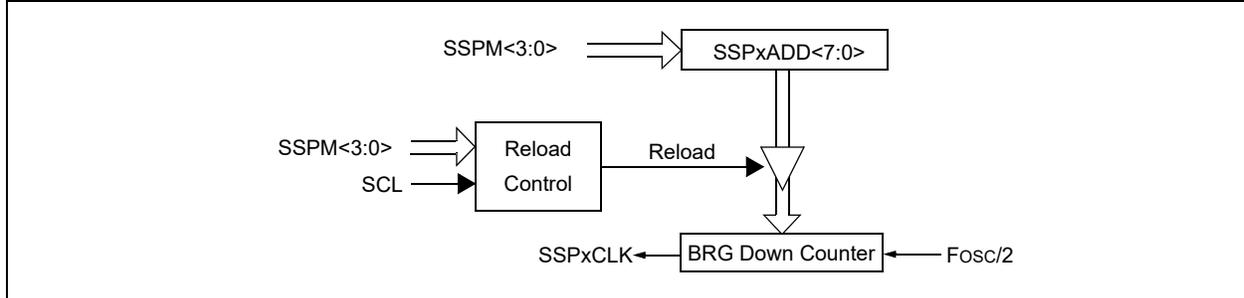
**Note:** Values of 0x00, 0x01 and 0x02 are not valid for SSPxADD when used as a Baud Rate Generator for I<sup>2</sup>C. This is an implementation limitation.
