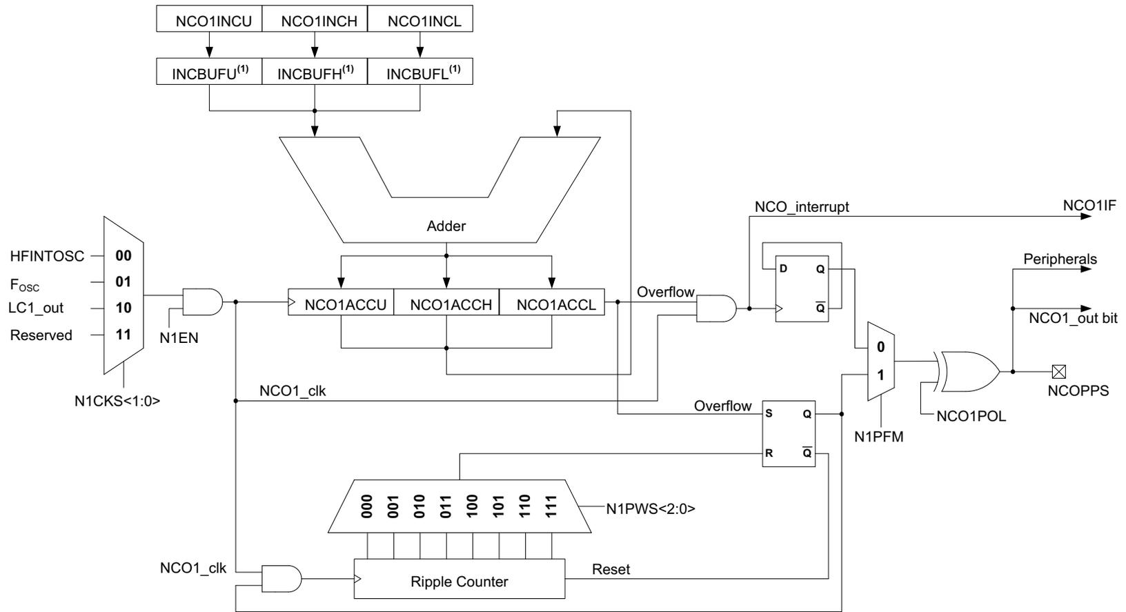
**Note 1:** The increment registers are double-buffered to allow for value changes to be made without first disabling the NCO1 module. They are shown for reference only and are not user accessible.
