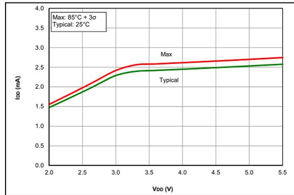
**FIGURE 36-4:**  $I_{DD}$ , HS Oscillator, 32 MHz, PIC16F18325/18345 Only
