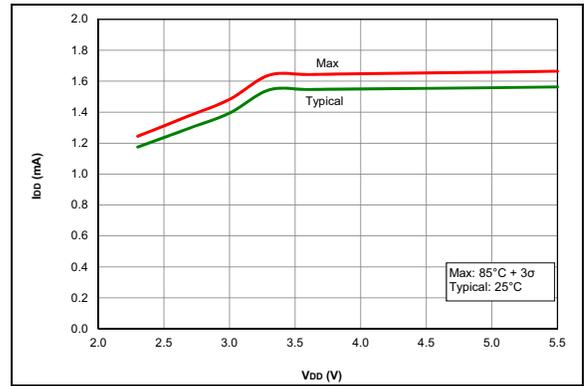
**FIGURE 36-8:**  $I_{DD}$ , HFINTOSC Mode,  $F_{osc} = 16$  MHz, PIC16F18325/18345 Only
