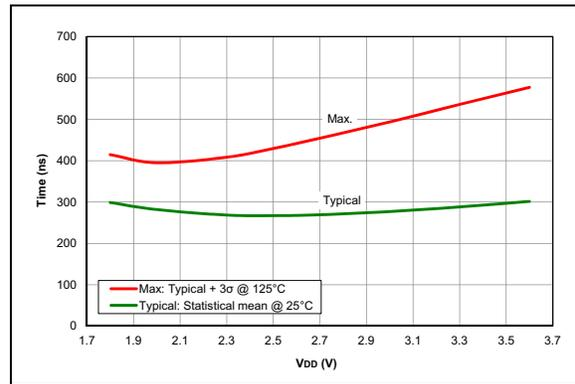
**FIGURE 36-88:** Comparator Response Time Rising edge, PIC16F18325/18345 Only
