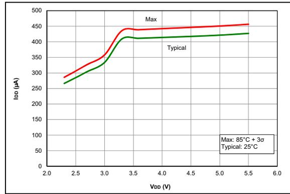
**FIGURE 36-2:**  $I_{DD}$ , XT Oscillator, 4 MHz, PIC16F18325/18345 Only
