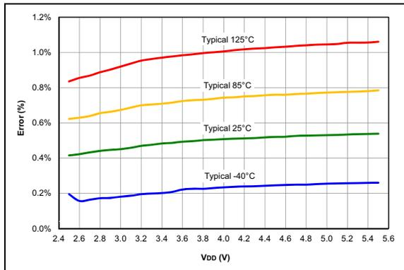
**FIGURE 36-93:** FVR Voltage Error (1x), PIC16F18325/18345 Only
