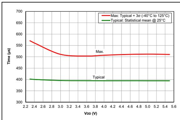
**FIGURE 36-113:** Wake From Sleep, VREGPM = 1, LFINTOSC, PIC16LF18325/18345 Only
