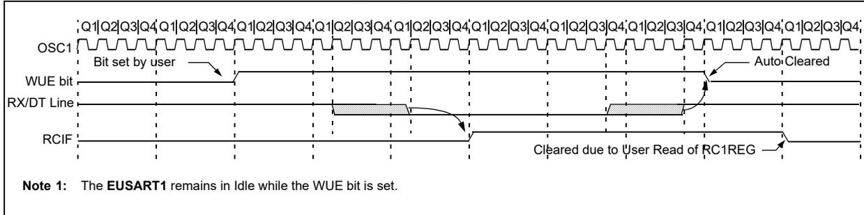
**FIGURE 31-8: AUTO-WAKE-UP BIT (WUE) TIMINGS DURING SLEEP**
