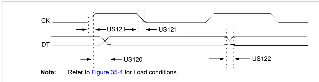
**TABLE 35-20: EUSART SYNCHRONOUS TRANSMISSION CHARACTERISTICS**
