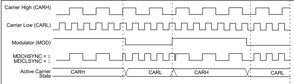
**FIGURE 25-6: FULL SYNCHRONIZATION (MDSHSYNC = 1, MDCLSYNC = 1)**
