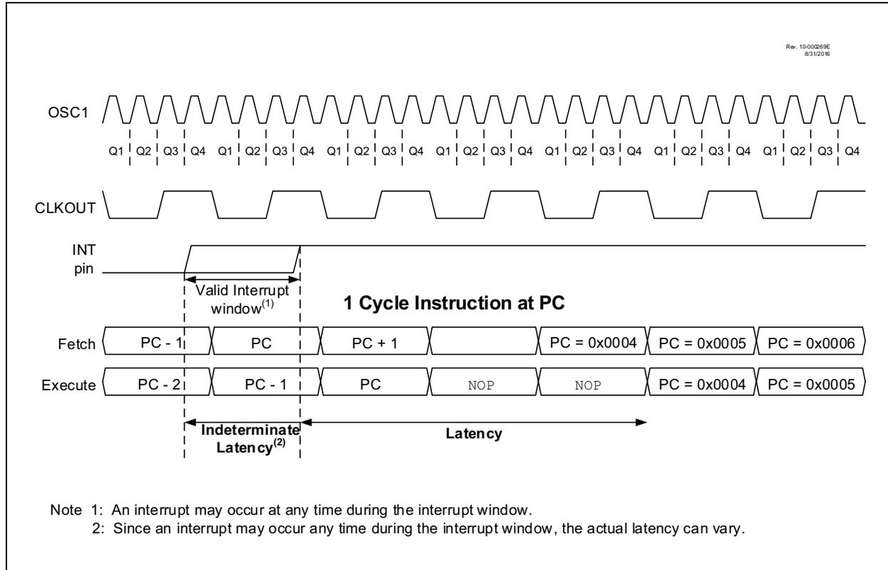
**FIGURE 8-3: INT PIN INTERRUPT TIMING**
