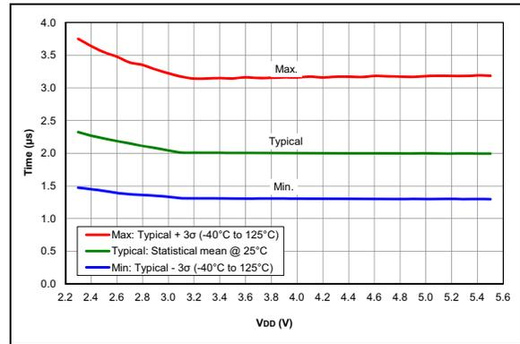
**FIGURE 36-68:** ADC RC Oscillator period, PIC16F18325/18345 Only
