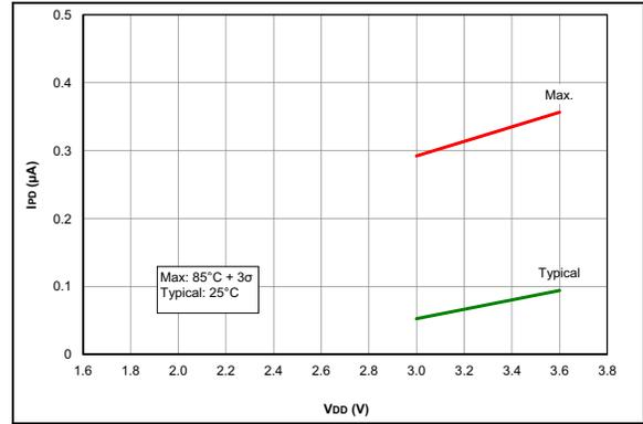
**FIGURE 36-20:** *IPD, Low-Power Brown-out Reset (LPBOR = 0), PIC16LF18325/18345 Only*
