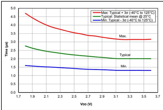
**FIGURE 36-67:** ADC RC Oscillator period, PIC16LF18325/18345 Only
