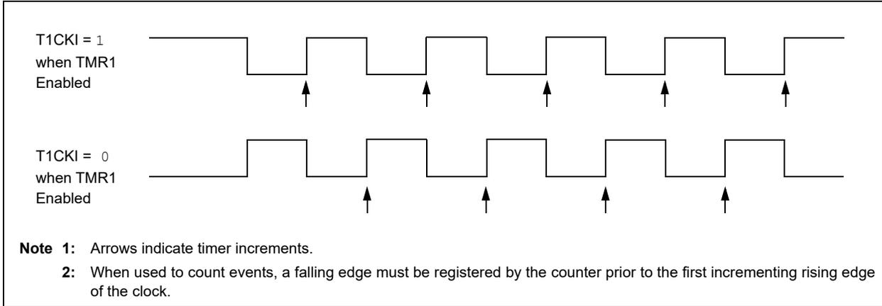
**FIGURE 27-3: TIMER1 GATE ENABLE MODE**
