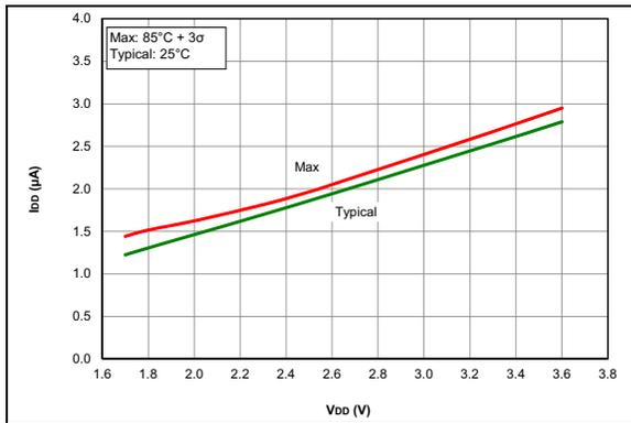
**FIGURE 36-3:**  $I_{DD}$ , HS Oscillator, 32 MHz, PIC16LF18325/18345 Only
