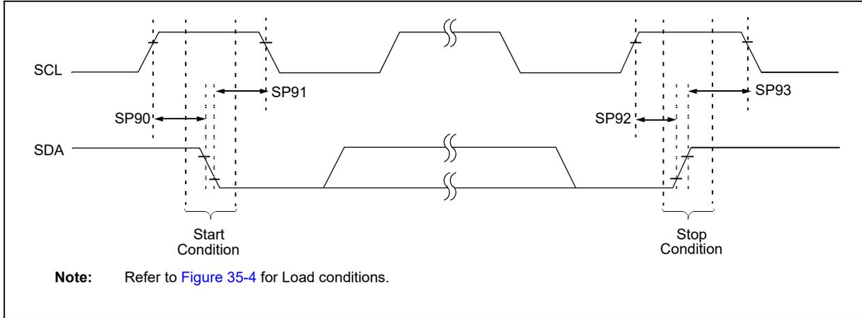
**TABLE 35-23: I<sup>2</sup>C BUS START/STOP BITS CHARACTERISTICS**
