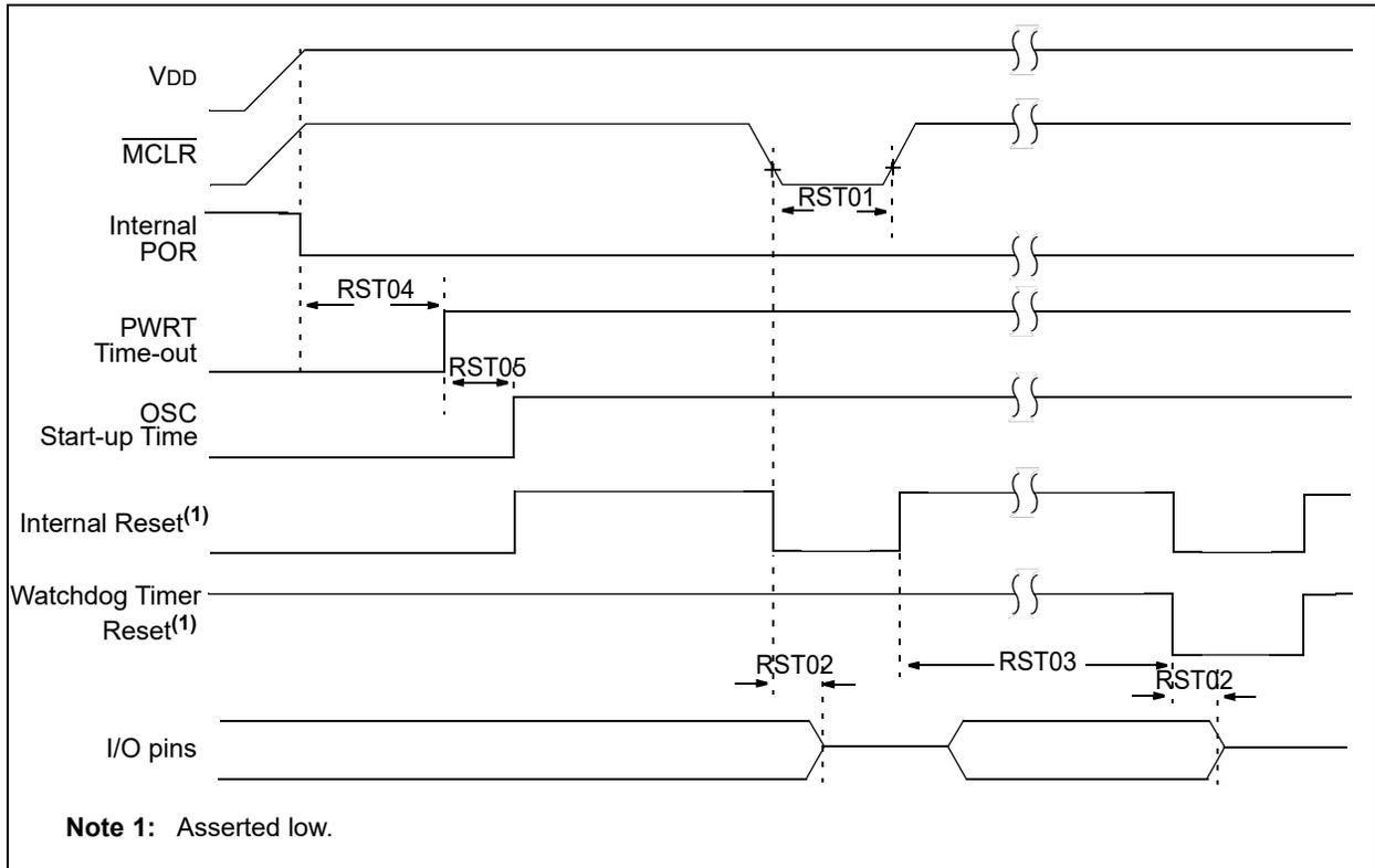
**FIGURE 35-9: BROWN-OUT RESET TIMING AND CHARACTERISTICS**
