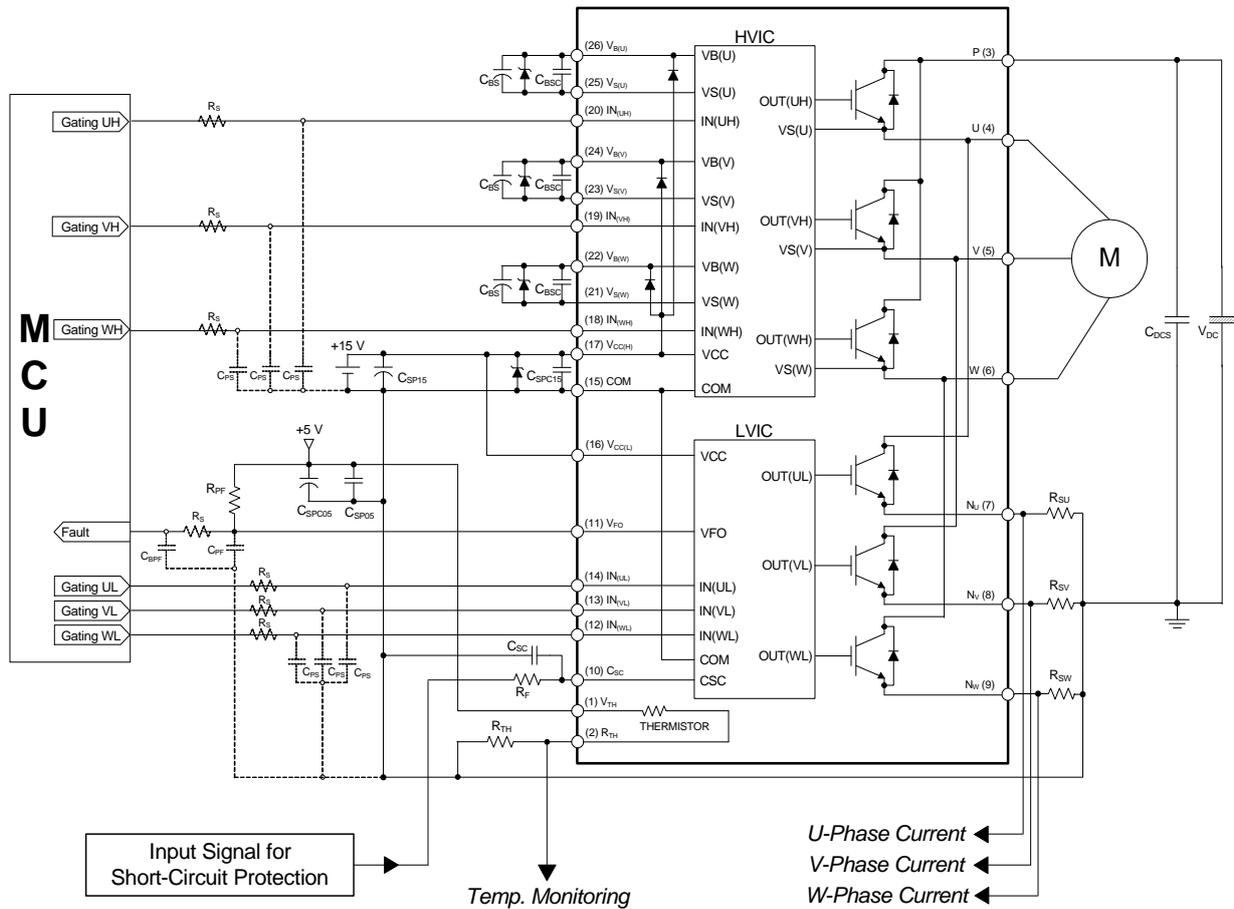
**Figure 15. Typical Application Circuit**
