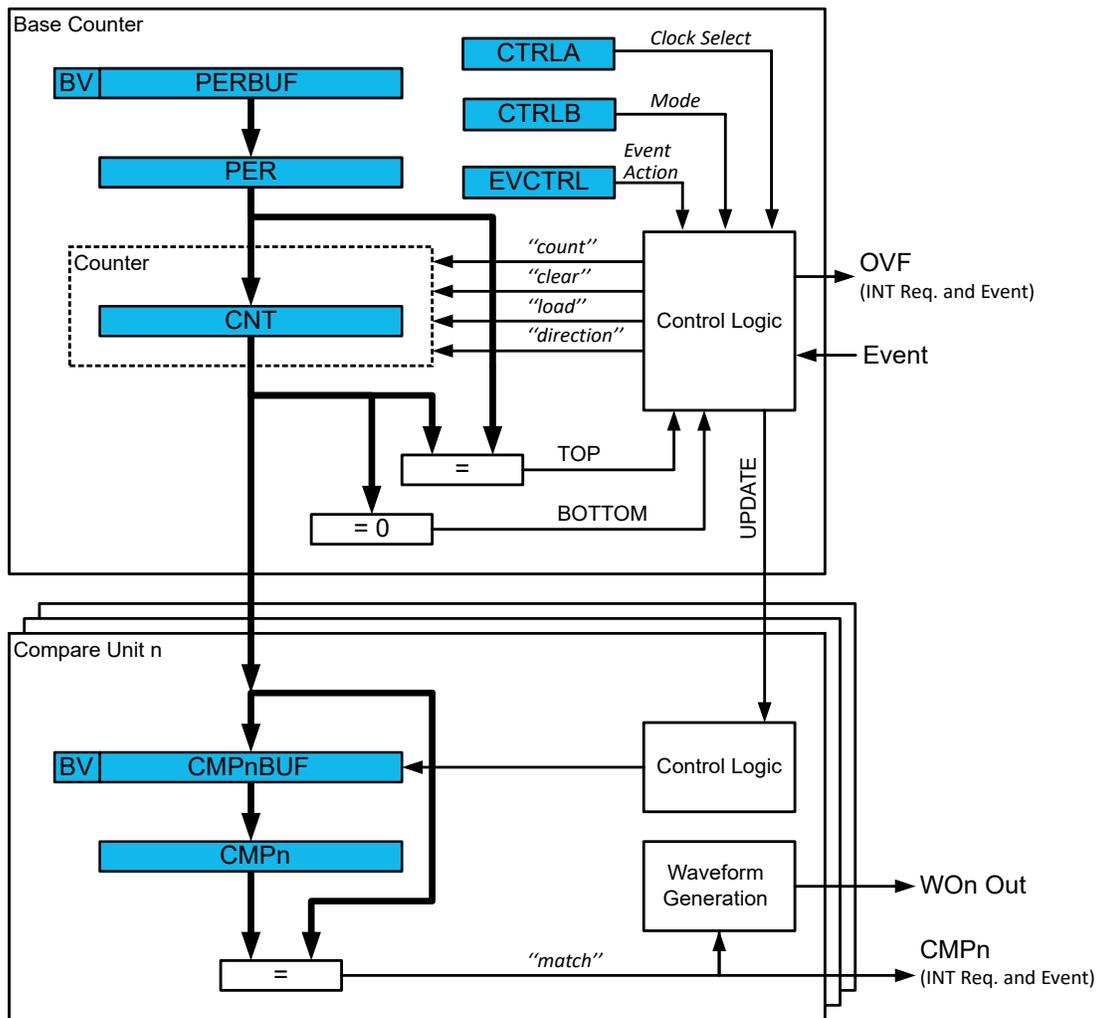
The Counter register (TCA<sub>n</sub>.CNT), Period and Compare registers (TCA<sub>n</sub>.PER and TCA<sub>n</sub>.CMP<sub>m</sub>) and their corresponding buffer registers (TCA<sub>n</sub>.PERBUF and TCA<sub>n</sub>.CMPBUF<sub>m</sub>) are 16-bit registers. All buffer registers have a Buffer Valid (BV) flag that indicates when the buffer contains a new value.
