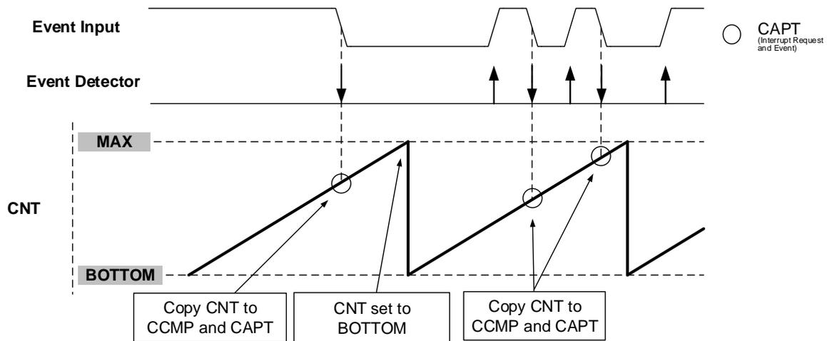
It is recommended to write zero to the TCBn.CNT register when entering this mode from any other mode.
