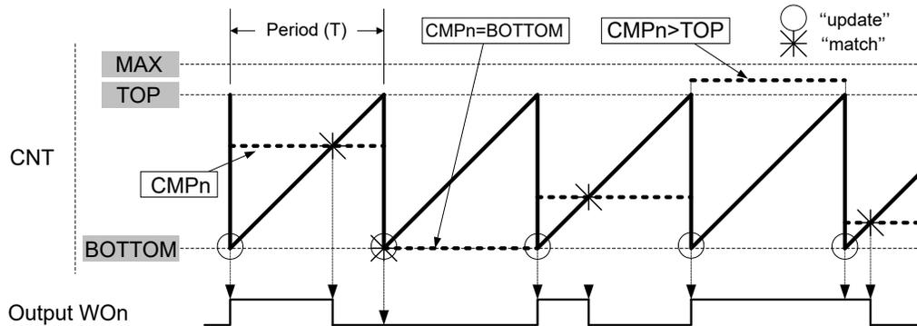
The TCA<sub>n</sub>.PER register defines the PWM resolution. The minimum resolution is 2 bits (TCA.PER = 0x0002), and the maximum resolution is 16 bits (TCA.PER = MAX-1).
