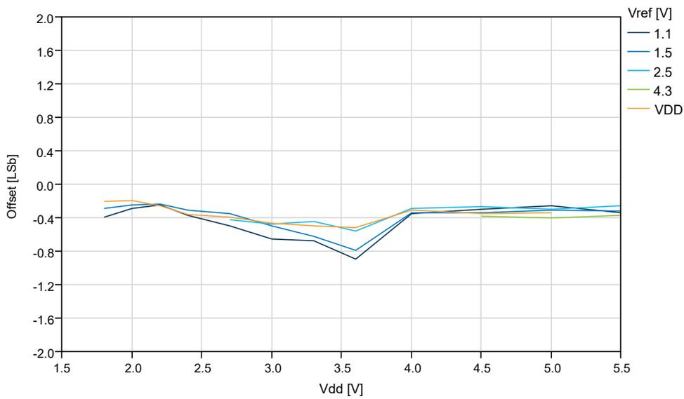
**Figure 33-53. Offset Error vs.  $V_{REF}$  ( $V_{DD} = 5.0V$ ,  $f_{ADC} = 115$  ksp/s), REFSEL = Internal Reference**
