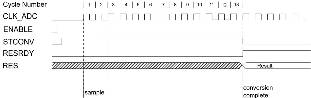
Both sampling time and sampling length can be adjusted using the Sample Delay bit field in Control D (ADCn.CTRLD) and sampling Sample Length bit field in the Sample Control register (ADCn.SAMPCTRL). Both of these control the ADC sampling time in a number of CLK\_ADC cycles. This allows sampling high-impedance sources without relaxing conversion speed. See the register description for further information. Total sampling time is given by:
