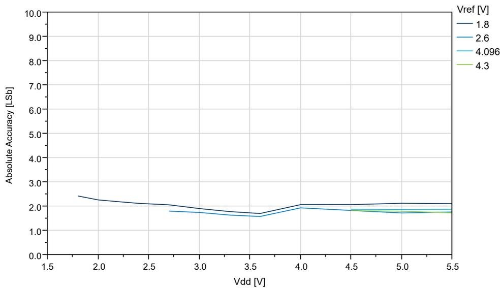
**Figure 33-55. Absolute Accuracy vs. V<sub>REF</sub> (V<sub>DD</sub> = 5.0V, f<sub>ADC</sub> = 115 kps, REFSEL = External Reference)**
