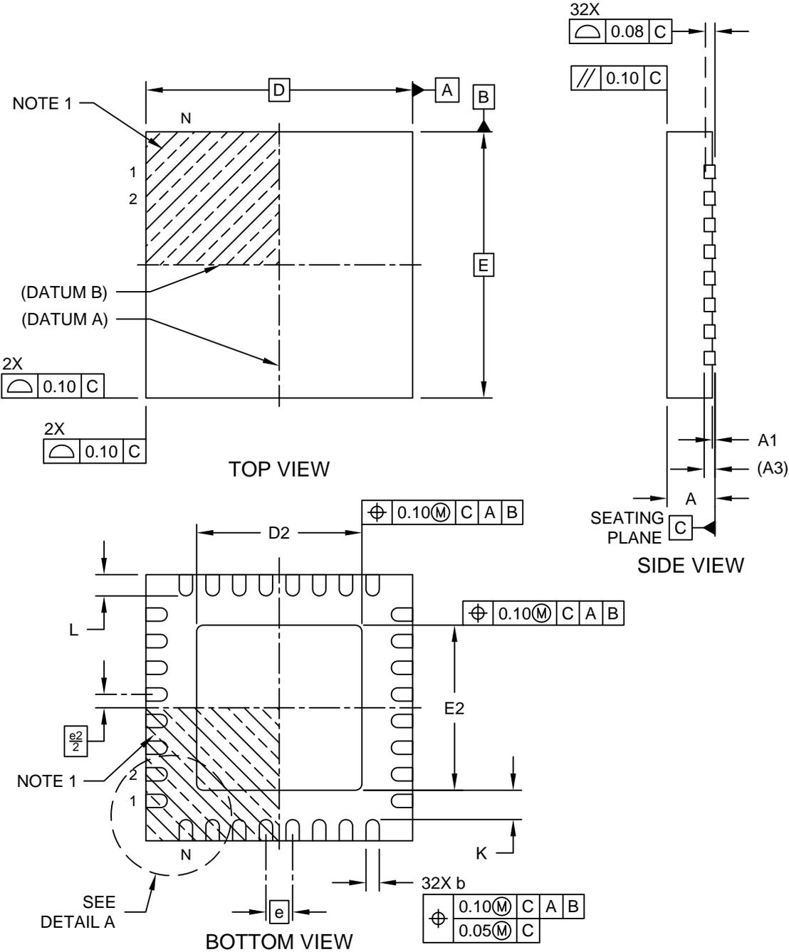
**32-Lead Very Thin Plastic Quad Flat, No Lead Package (RXB) - 5x5x0.9 mm Body [VQFN]
