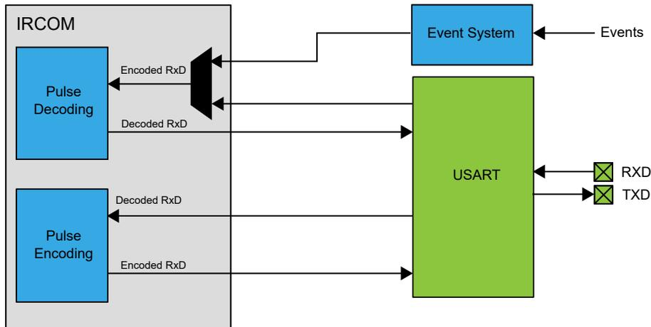
The USART is set in IRCOM mode by writing 0x02 to the CMODE bits in the USARTn.CTRLC register. The data on the TXD/RXD pins are the inverted values of the transmitted/received infrared pulse. It is also possible to select an event channel from the Event System as an input for the IRCOM receiver. This enables the IRCOM to receive input from the I/O pins or sources other than the corresponding RXD pin. This will disable the RxD input from the USART pin.
