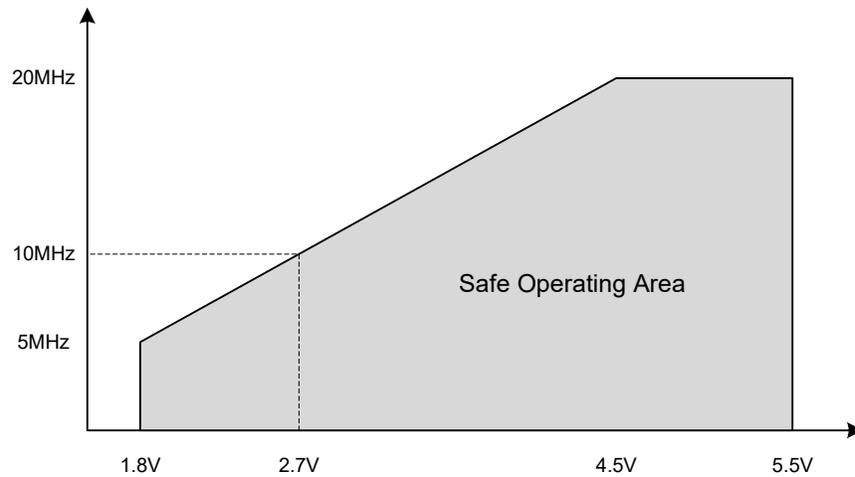
**Figure 32-2. Maximum Frequency vs.  $V_{DD}$  for [-40, 125]°C**
