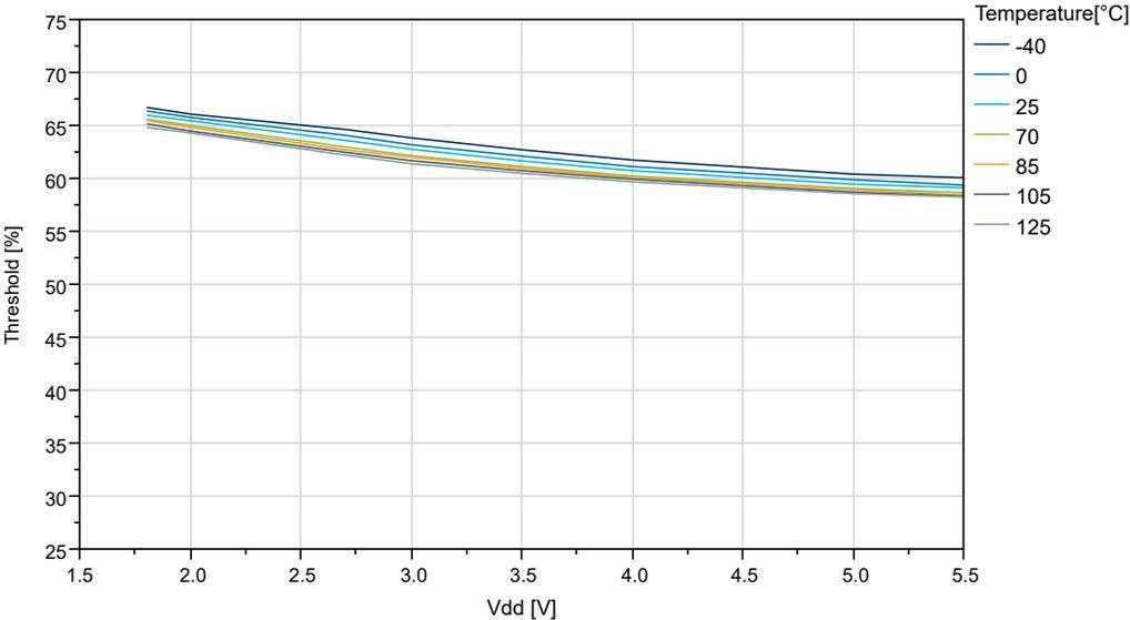
Figure 33-22. I/O Pin Input Threshold Voltage vs. V<sub>DD</sub> (V<sub>IL</sub>)
