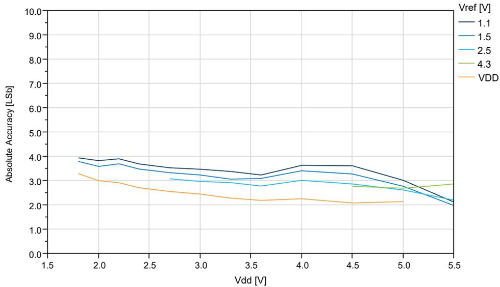
**Figure 33-45. Absolute Accuracy vs.  $V_{REF}$  ( $V_{DD} = 5.0V$ ,  $f_{ADC} = 115$  kps), REFSEL = Internal Reference**
