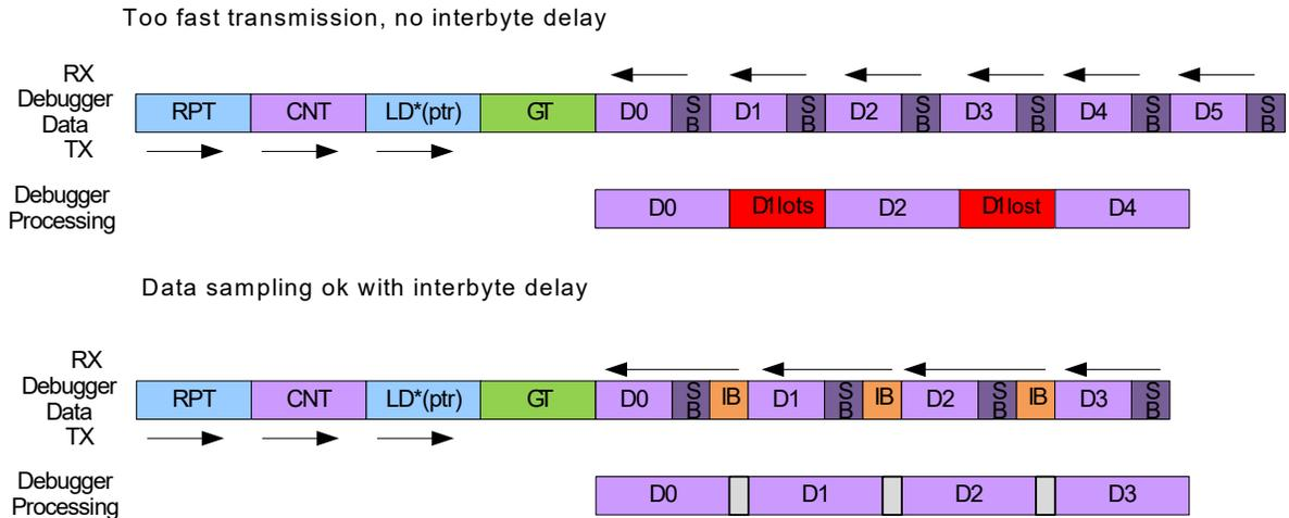
In Figure 30-16, GT denotes the Guard Time insertion, SB is for Stop Bit and IB is the inserted interbyte delay. The rest of the frames are data and instructions.
