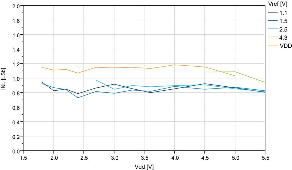
**Figure 33-51. INL vs.  $V_{REF}$  ( $V_{DD} = 5.0V$ ,  $f_{ADC} = 115$  ksps), REFSEL = Internal Reference**
