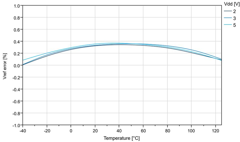
Figure 33-35. Internal 1.1V Reference vs. Temperature
