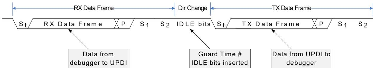
The UPDI Guard Time is the minimum IDLE time (see CTRLA.GTVAL) that the connected debugger will experience when waiting for data from the UPDI. The Maximum is the same as timeout (for example, 65536 UPDI clock cycles).
