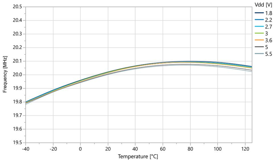
Figure 33-71. OSC20M Internal Oscillator: Frequency vs. V<sub>DD</sub>
