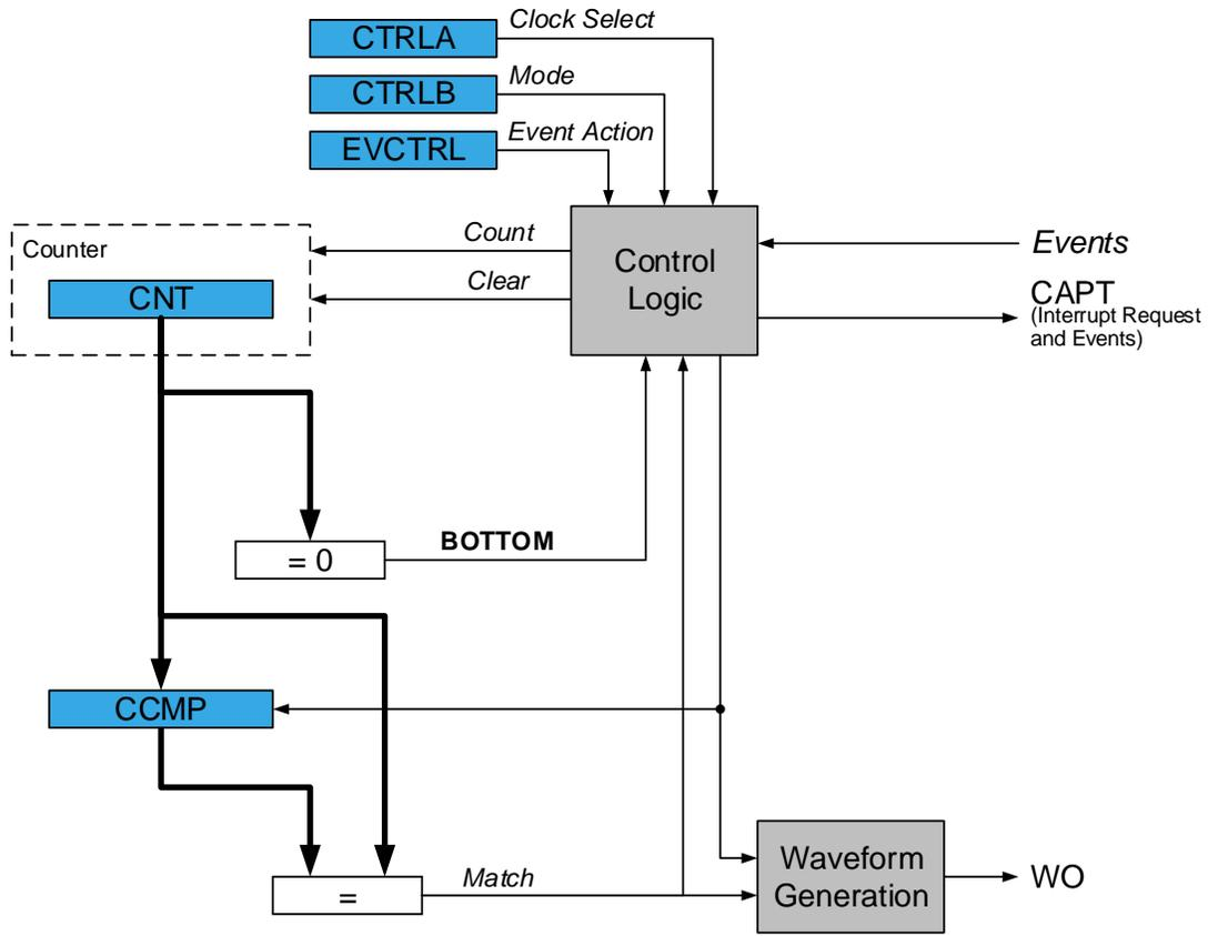
The timer/counter can be clocked from the Peripheral Clock (CLK\_PER), or a 16-bit Timer/Counter type A (CLK\_TCA<sub>n</sub>).
