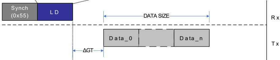
The figure above shows an example of a typical LD sequence, where data is received after the Guard Time period. Loading data from the UPDI Pointer register follows the same transmission protocol.
