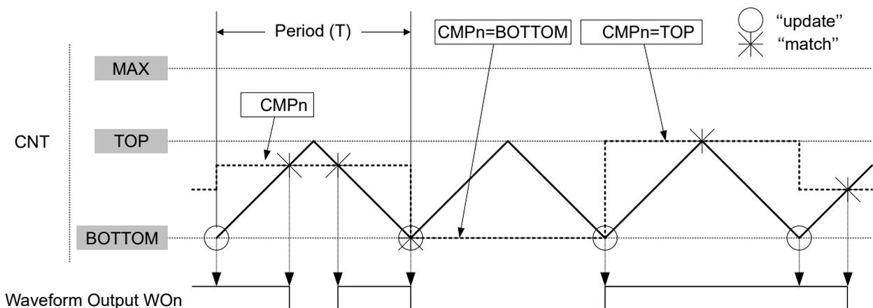
Using dual-slope PWM results in half the maximum operation frequency compared to single-slope PWM operation, due to twice the number of timer increments per period.
