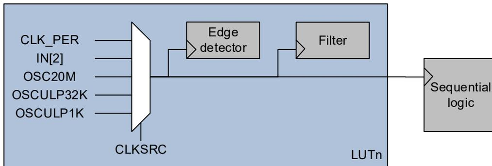
When the Clock Source (CLKSRC) bit is written to 0x1, IN[2] is used to clock the corresponding filter and edge detector (CLK\_LUTn). The sequencer is clocked by the CLK\_LUTn of the even LUT in the pair. When CLKSRC is written to 0x1, IN[2] is treated as OFF (low) in the TRUTH table.
