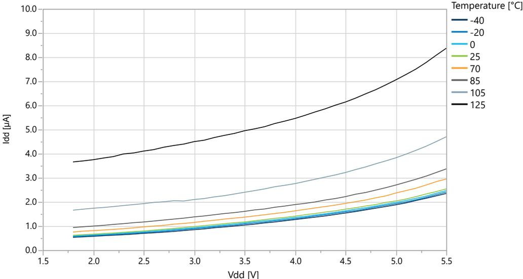
Figure 33-16. Standby Mode Supply Current vs. V<sub>DD</sub> (Sampled BOD running at 125 Hz)
