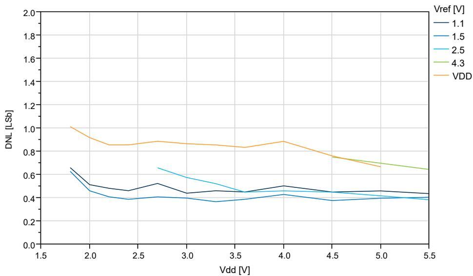
**Figure 33-47. DNL vs.  $V_{REF}$  ( $V_{DD} = 5.0V$ ,  $f_{ADC} = 115$  kps), REFSEL = Internal Reference**
