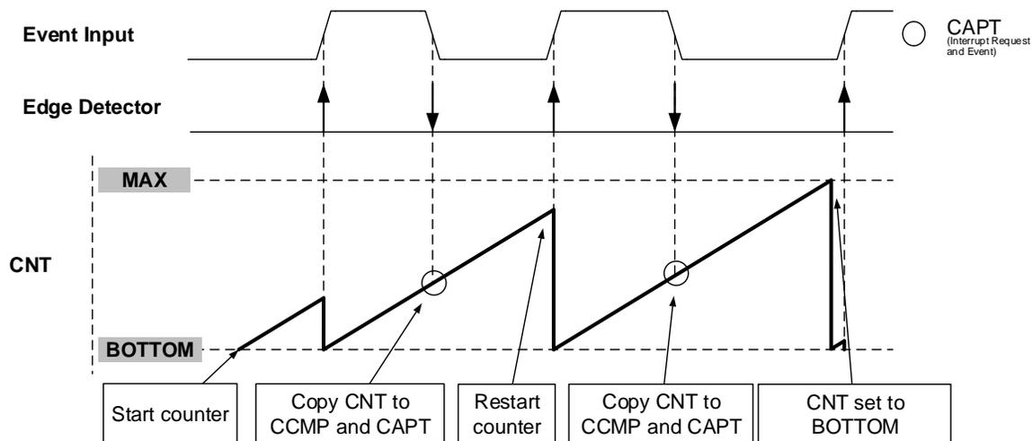
21.3.3.1.6 Input Capture Frequency and Pulse-Width Measurement Mode
