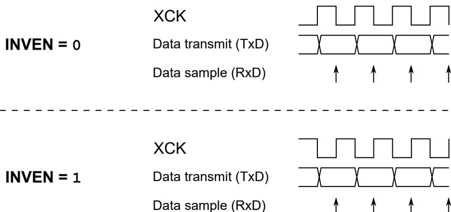
The I/O pin can be inverted by writing a '1' to the Inverted I/O Enable (INVEN) bit in the Pin n Control register of the port peripheral (PORTx.PINnCTRL). Using the inverted I/O setting for the corresponding XCK port pin, the XCK clock edges used for sampling RxD and transmitting on TxD can be selected. If the inverted I/O is disabled (INVEN = 0), the rising XCK clock edge represents the start of a new data bit, and the received data will be sampled at the falling
