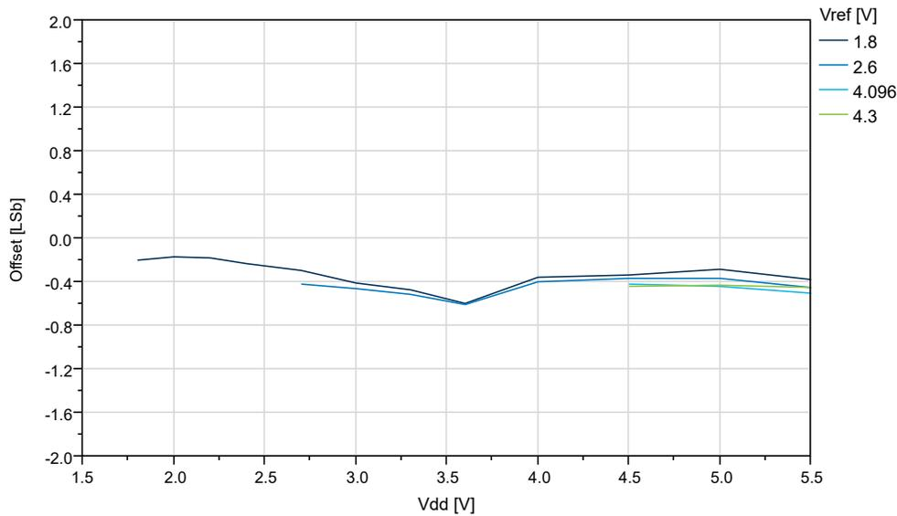
Figure 33-63. Offset vs.  $V_{REF}$  ( $V_{DD} = 5.0V$ ,  $f_{ADC} = 115$  ksp/s, REFSEL = External Reference)
