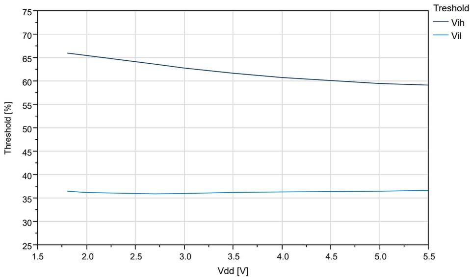
Figure 33-21. I/O Pin Input Threshold Voltage vs. V<sub>DD</sub> (V<sub>IH</sub>)
