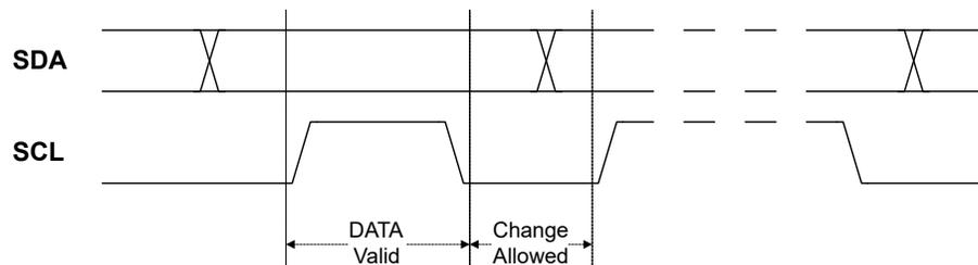
Combining bit transfers result in the formation of address and data packets. These packets consist of eight data bits (one byte) with the Most Significant bit transferred first, plus a single-bit not-Acknowledge (NACK) or Acknowledge (ACK) response. The addressed device signals ACK by pulling the SCL line low during the ninth clock cycle, and signals NACK by leaving the line SCL high.
