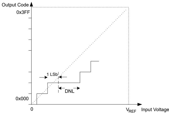
**Quantization Error** Due to the quantization of the input voltage into a finite number of codes, a range of input voltages (1 LSb wide) will code to the same value. Always  $\pm 0.5$  LSb.
