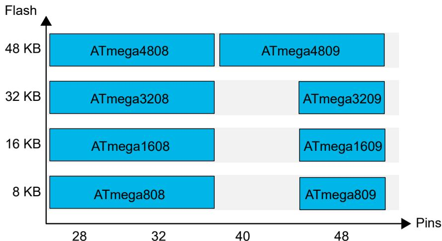
Devices with different Flash memory sizes typically also have different SRAM and EEPROM.
