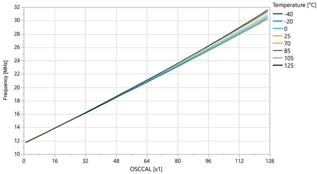
**Figure 33-70. OSC20M Internal Oscillator: Frequency vs. Temperature**
