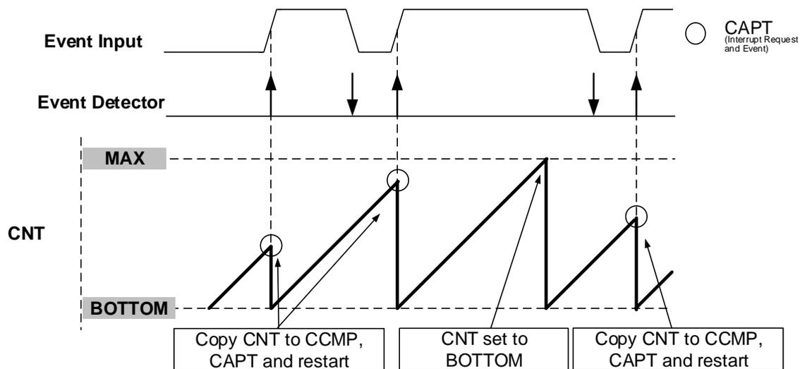
**21.3.3.1.5 Input Capture Pulse-Width Measurement Mode**
