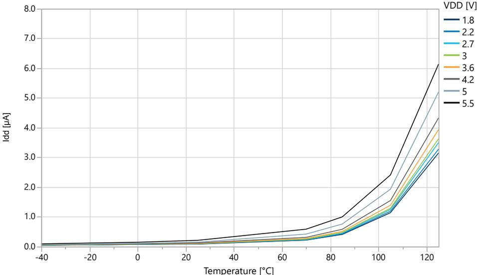
**Figure 33-14. Power-Down Mode Supply Current vs. V<sub>DD</sub> (all functions disabled)**
