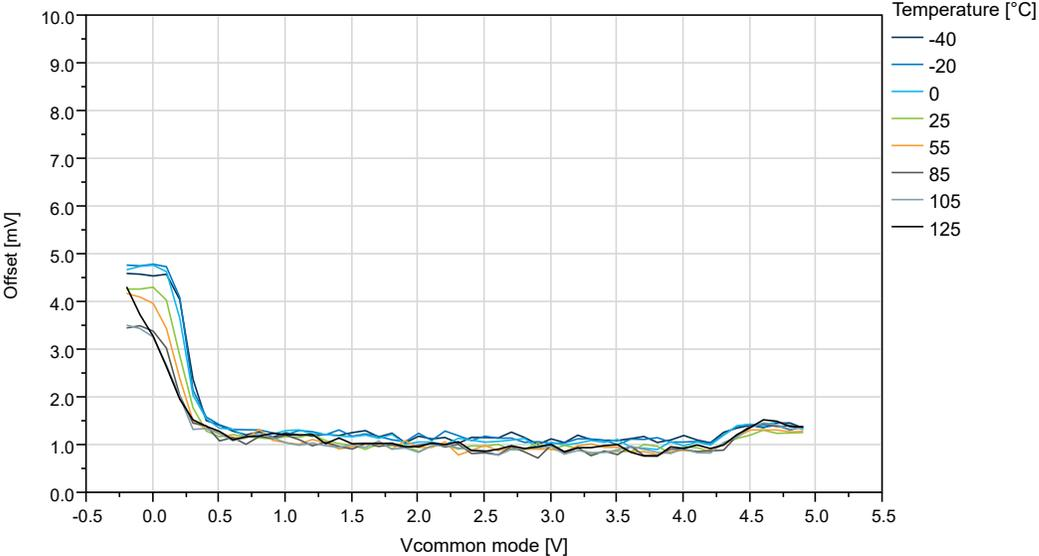
Figure 33-67. Offset vs.  $V_{CM}$  - 10 mV to 50 mV ( $V_{DD} = 5V, T = 25^{\circ}C$ )
