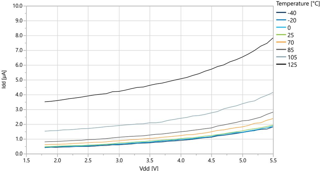
**Figure 33-17. Standby Mode Supply Current vs.  $V_{DD}$  (Sampled BOD running at 1 kHz)**
