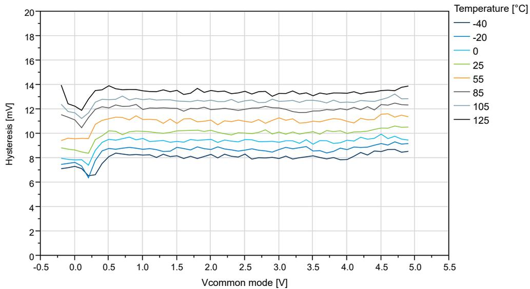
Figure 33-65. Hysteresis vs.  $V_{CM}$  - 10 mV to 50 mV ( $V_{DD} = 5V$ ,  $T = 25^{\circ}C$ )
