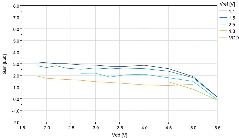
**Figure 33-49. Gain Error vs. V<sub>REF</sub> (V<sub>DD</sub> = 5.0V, f<sub>ADC</sub> = 115 kps), REFSEL = Internal Reference**
