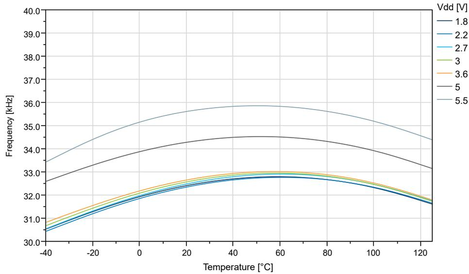
Figure 33-73. OSCULP32K Internal Oscillator: Frequency vs. V<sub>DD</sub>
