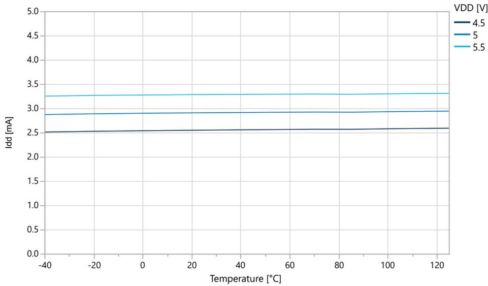
Figure 33-11. Idle Supply Current vs. Temperature (f = 16 MHz)
