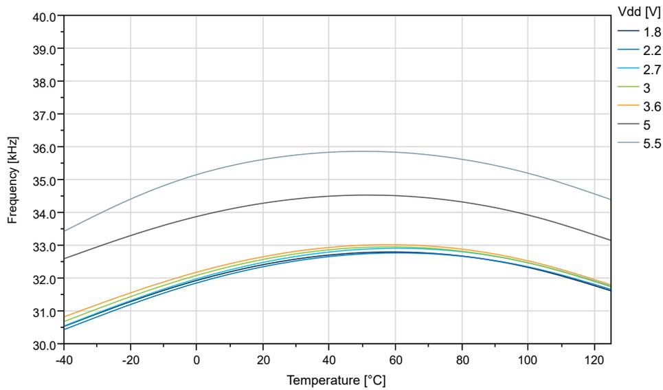
**Figure 34-61. OSCULP32K Internal Oscillator Frequency vs.  $V_{DD}$**
