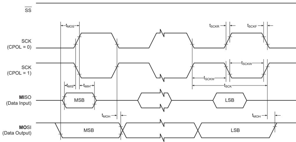
**Figure 33-6. SPI - Timing Requirements in Slave Mode**
