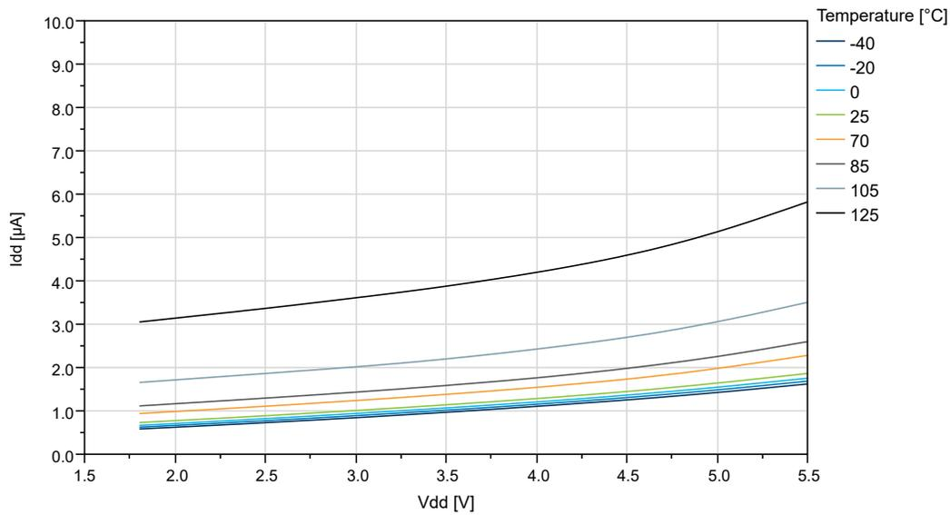
**Figure 34-13. Standby Mode Supply Current vs.  $V_{DD}$  (RTC running with internal OSCULP32K)**
