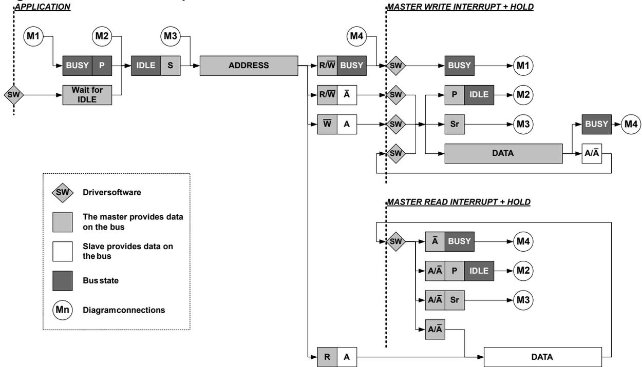
The number of interrupts generated is kept to a minimum by automatic handling of most conditions.
