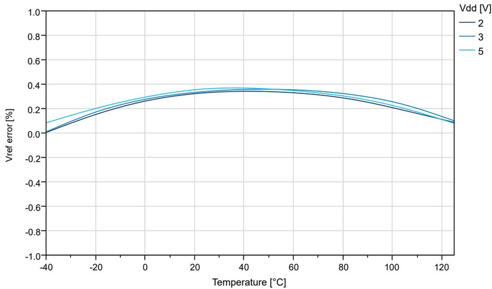
Figure 34-33. Internal 1.1V Reference vs. Temperature
