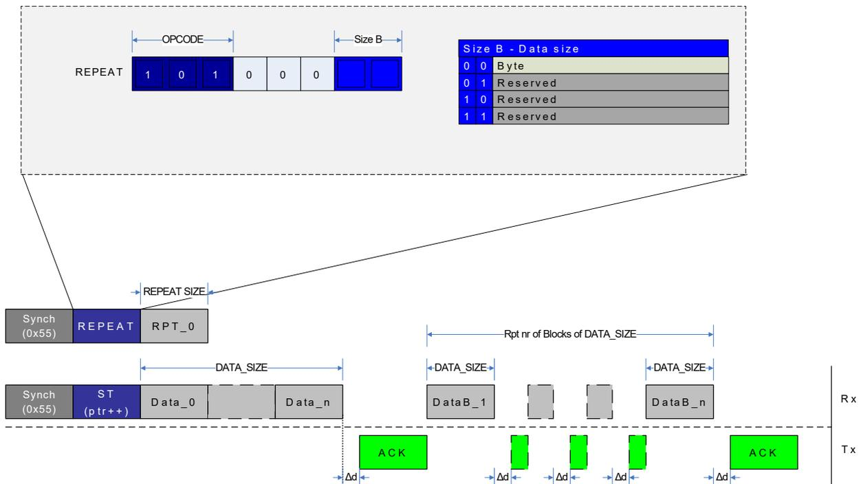
The Figure above gives an example of repeat operation with a `ST` instruction using pointer post increment operation. After the `REPEAT` instruction is sent with `RPT_0 = n`, the first `ST` instruction is issued with `SYNCH-` and Instruction frame, while the next `n` `ST`-instructions are executed by only sending in data bytes according to the `ST` operand `DATA_SIZE`, and maintaining the Acknowledge (ACK) handshake protocol.
