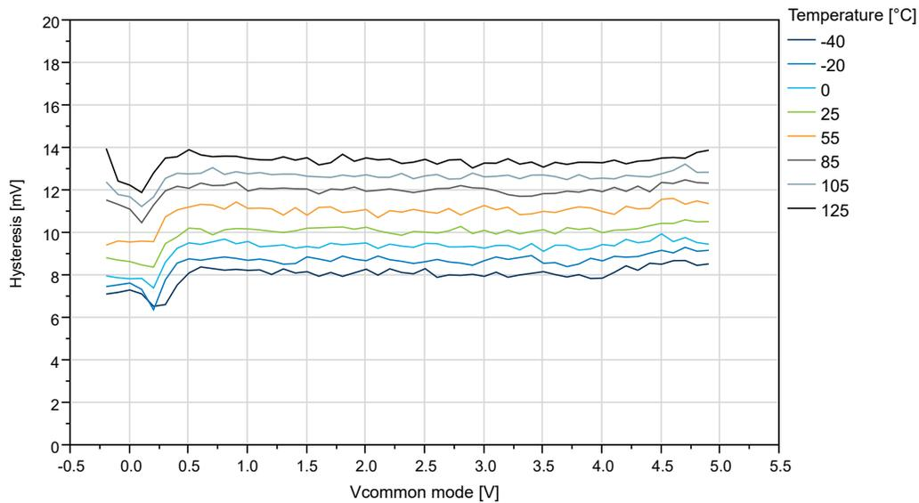
**Figure 34-53. Hysteresis vs.  $V_{CM}$  - 10mV to 50mV ( $V_{DD}=5V$ ,  $T=25^{\circ}C$ )**
