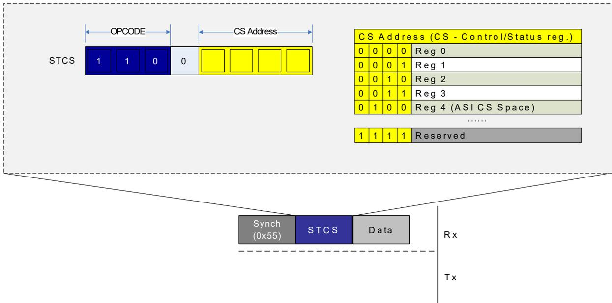
Figure 32-14 shows the data frame transmitted after the SYNCH and instruction frames. There is no response generated from the STCS instruction, as is the case for ST and STS.
