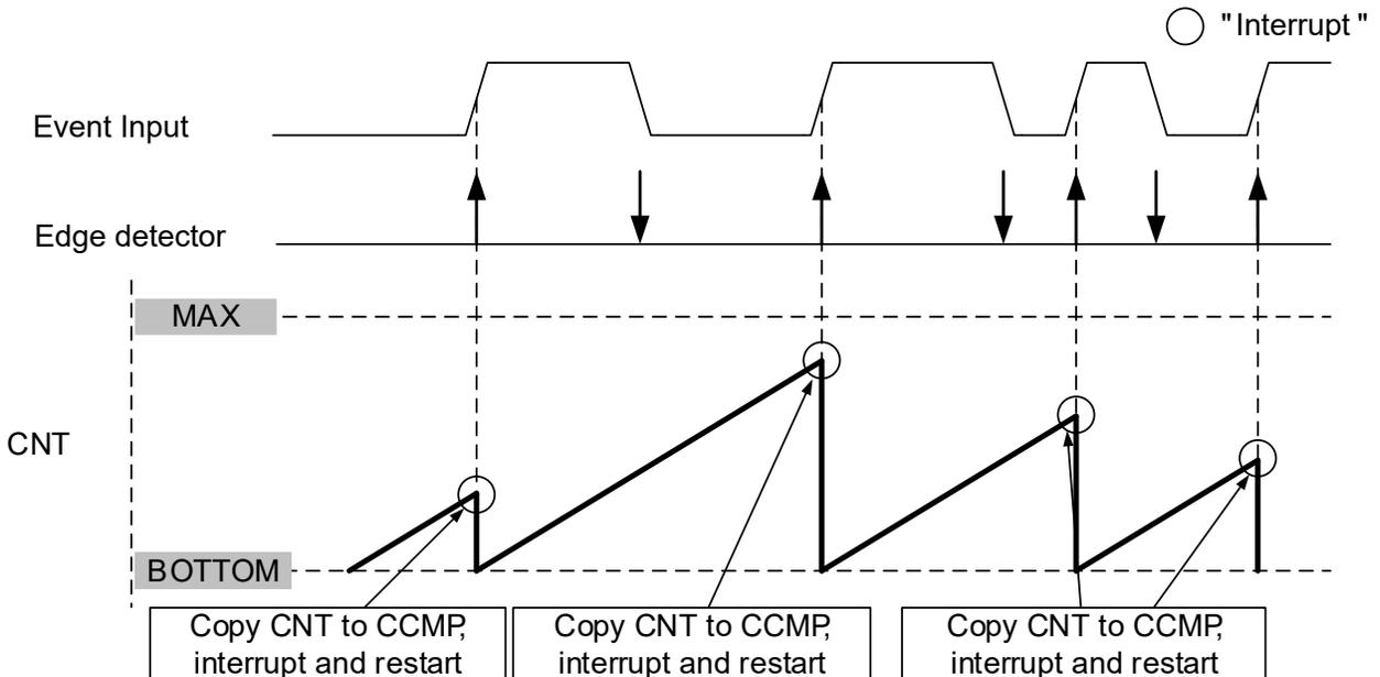
**21.3.3.1.5 Input Capture Pulse Width Measurement Mode**
