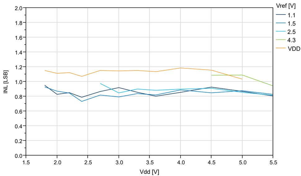
**Figure 34-49. INL vs.  $V_{ref}$  ( $V_{DD}=5.0V$ , 115ksps)**
