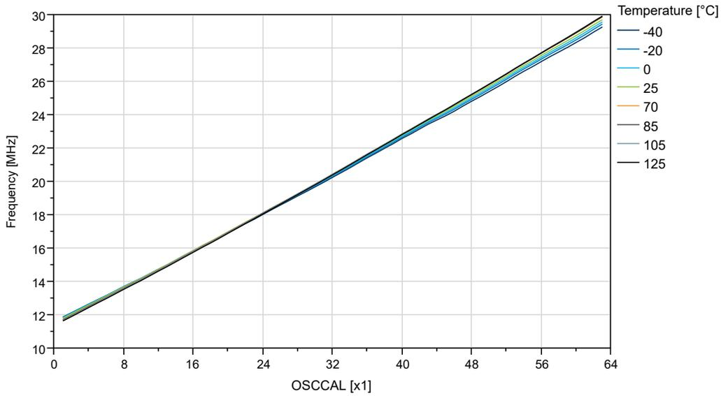
**Figure 34-58. OSC20M Internal Oscillator: Frequency vs. Temperature**
