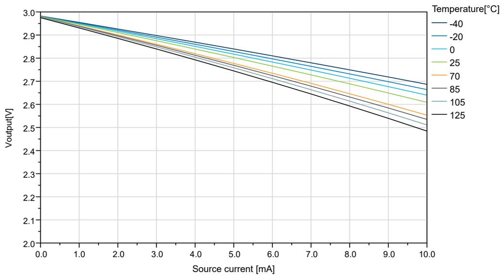
**Figure 34-27. IO Pin Output Voltage vs. Source Current ( $V_{DD}=5.0V$ )**
