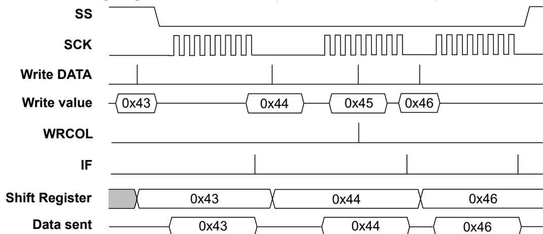
The figure shows three transfers and one write to the DATA register while the SPI is busy with a transfer. This write will be ignored and the Write Collision Flag (INTFLAGS.WRCOL) is set.
