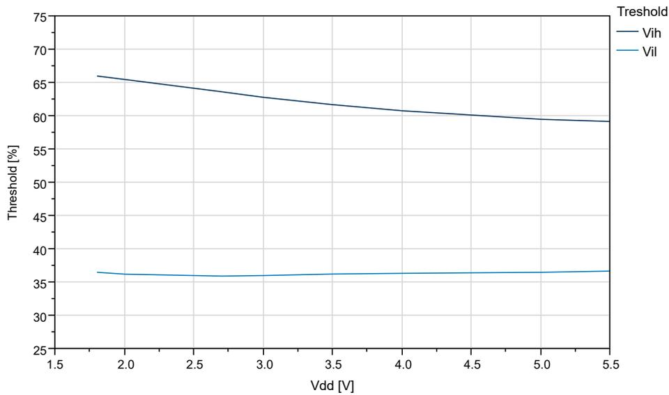
**Figure 34-19. IO Pin Input Threshold Voltage vs.  $V_{DD}$  ( $V_{IH}$ )**
