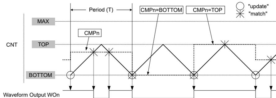
Using dual-slope PWM results in a lower maximum operation frequency compared to the single-slope PWM operation.
