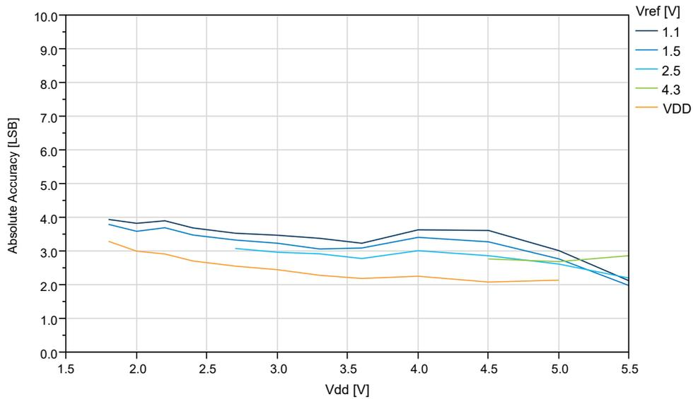
**Figure 34-43. Absolute Accuracy vs.  $V_{ref}$  ( $V_{DD}=5.0V$ , 115kps)**
