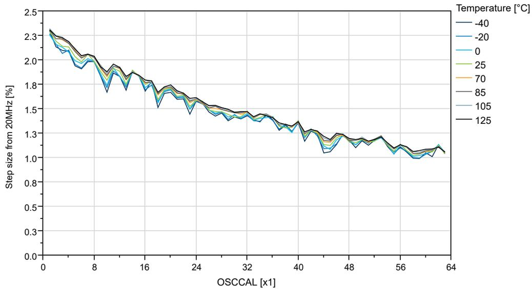
**Figure 34-57. OSC20M internal Oscillator: Frequency vs. Calibration Value ( $V_{DD}=3V$ )**
