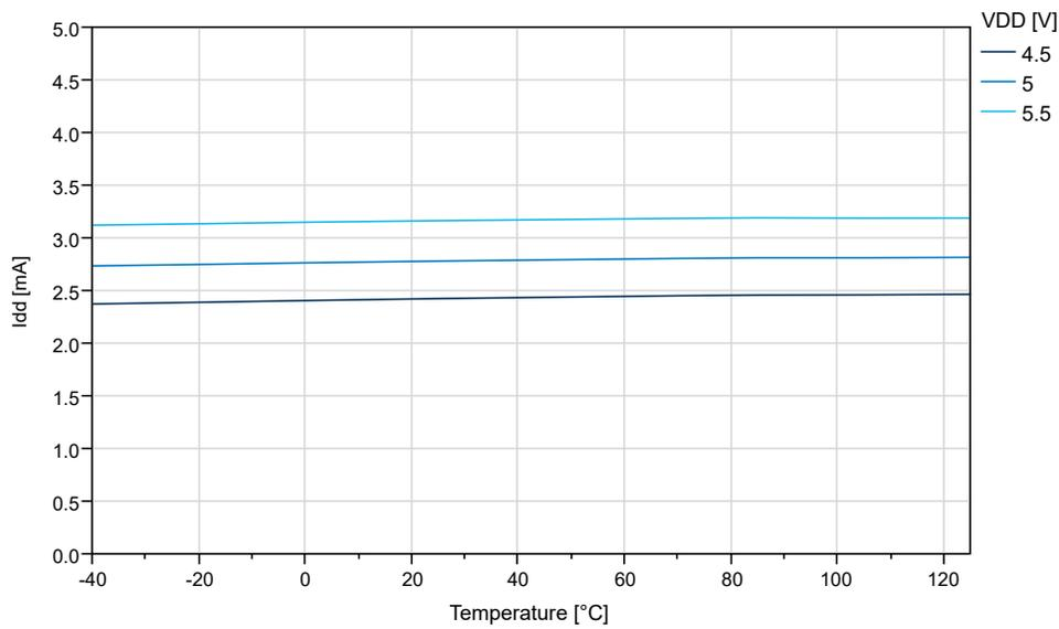
**Figure 34-9. Idle Supply Current vs.  $V_{DD}$  ( $f=32\text{KHz OSCULP32K}$ )**
