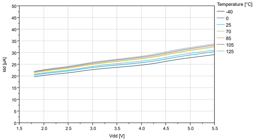
Figure 34-37. BOD Current vs.  $V_{DD}$  (Sampled BOD at 125Hz)
