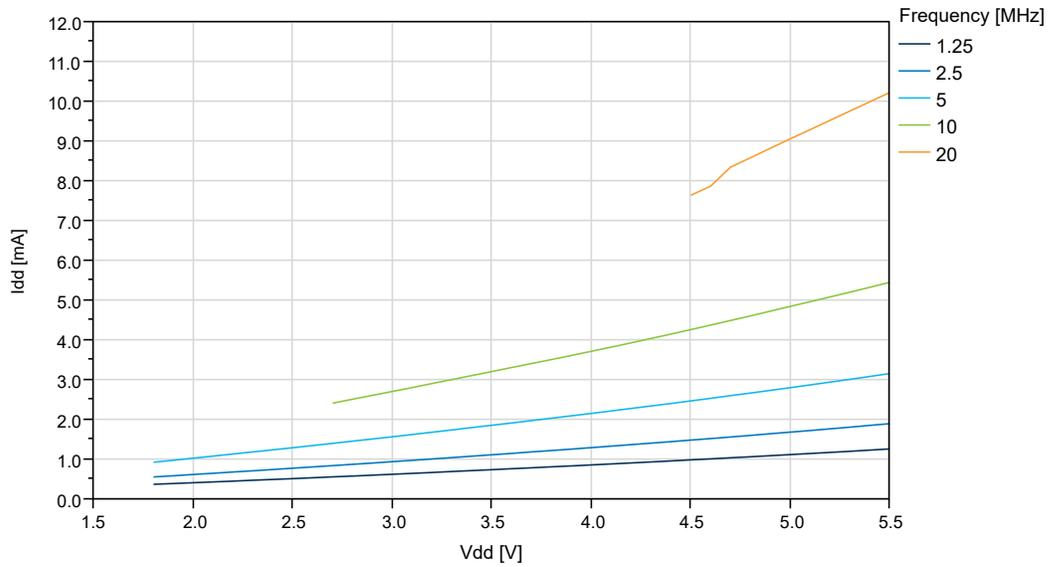
**Figure 34-5. Active Supply Current vs.  $V_{DD}$  ( $f=32\text{KHz OSCULP32K}$ )**
