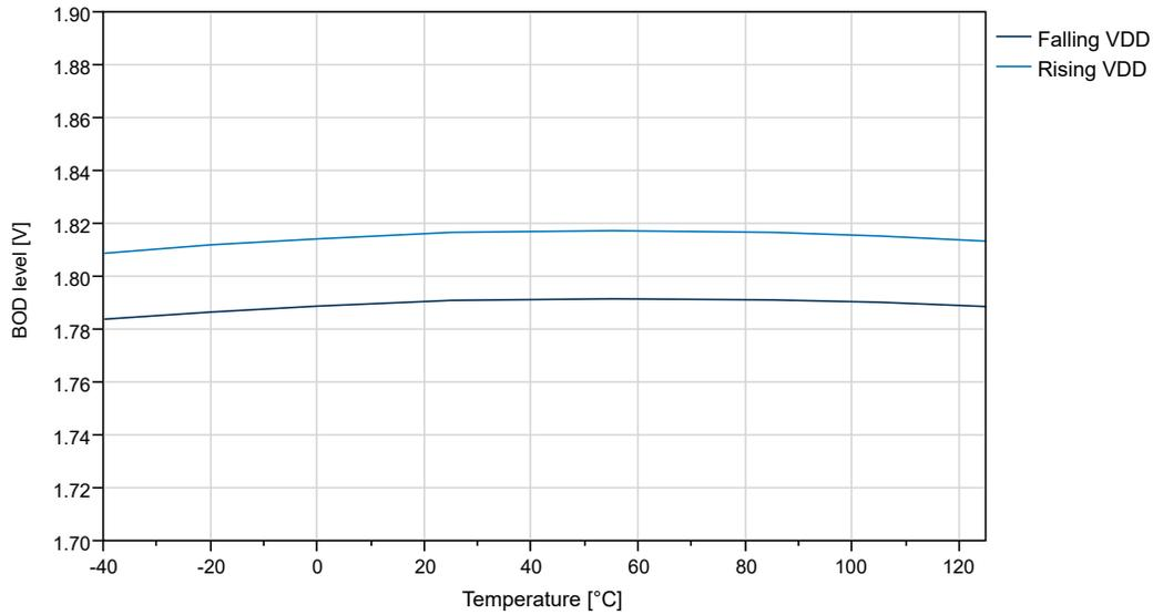
Figure 34-40. BOD Threshold vs. Temperature (Level 2.6V)
