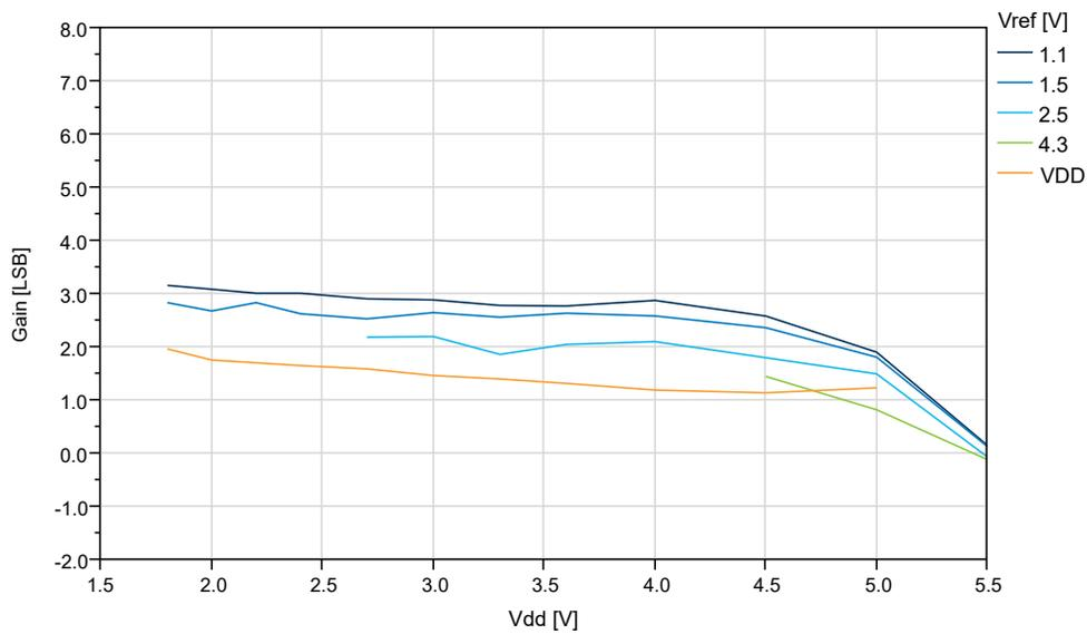
**Figure 34-47. Gain Error vs.  $V_{ref}$  ( $V_{DD}=5.0V$ , 115kps)**
