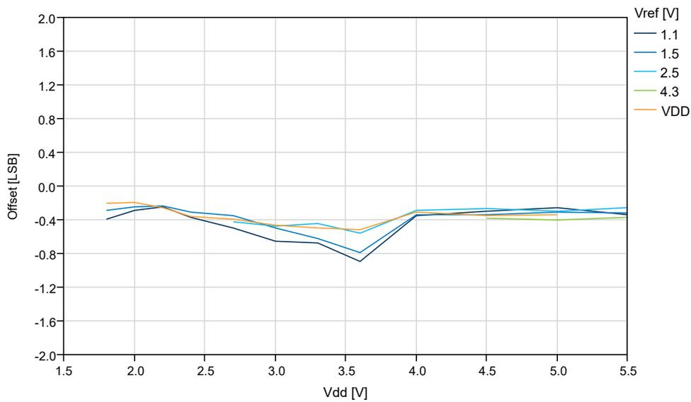
**Figure 34-51. Offset Error vs.  $V_{ref}$  ( $V_{DD}=5.0V$ , 115ksps)**
