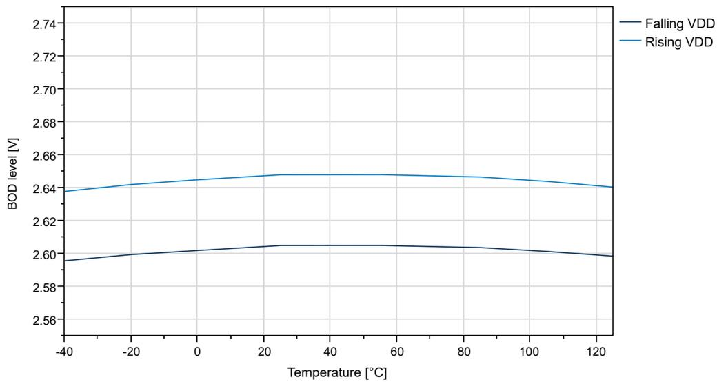
**Figure 34-41. BOD Threshold vs. Temperature (Level 4.3V)**
