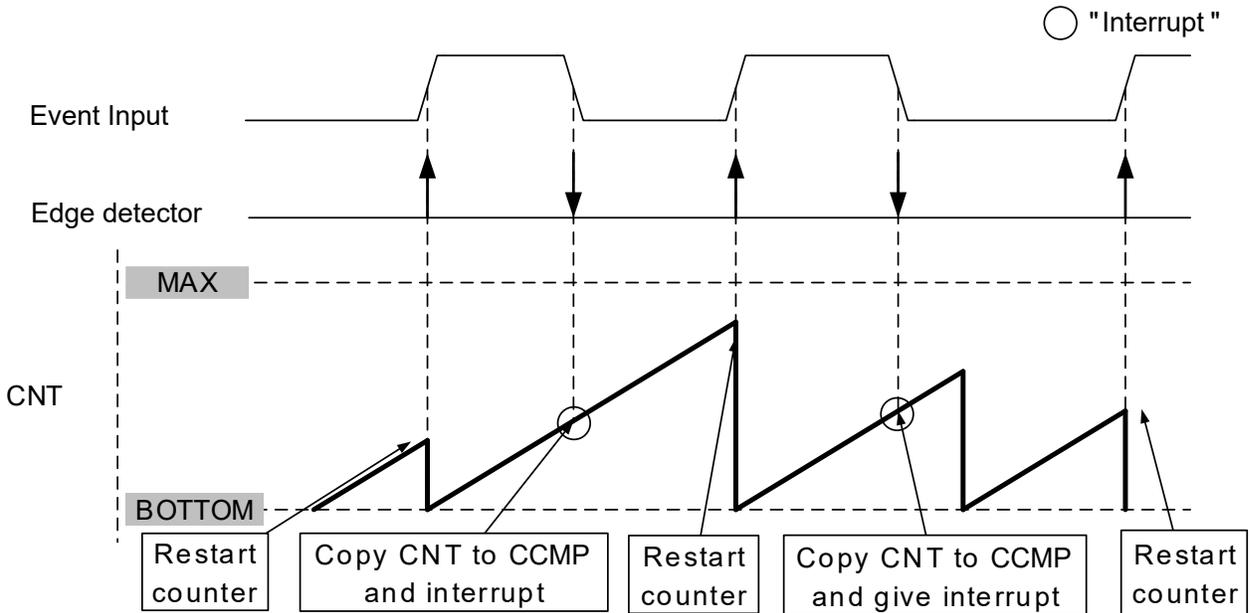
**21.3.3.1.6 Input Capture Frequency and Pulse Width Measurement Mode**
