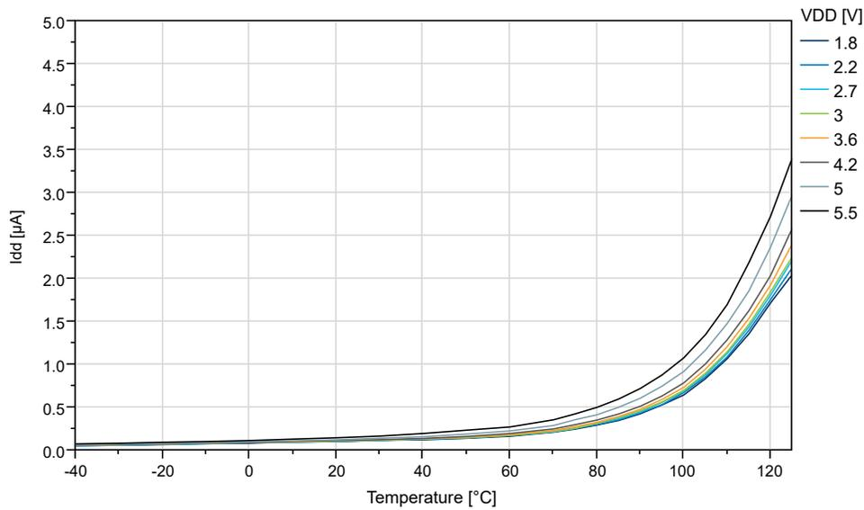
**Figure 34-11. Power Down Mode Supply Current vs.  $V_{DD}$  (all functions disabled)**
