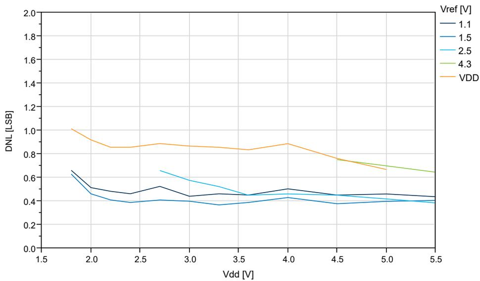
**Figure 34-45. DNL vs.  $V_{ref}$  ( $V_{DD}=5.0V$ , 115ksps)**
