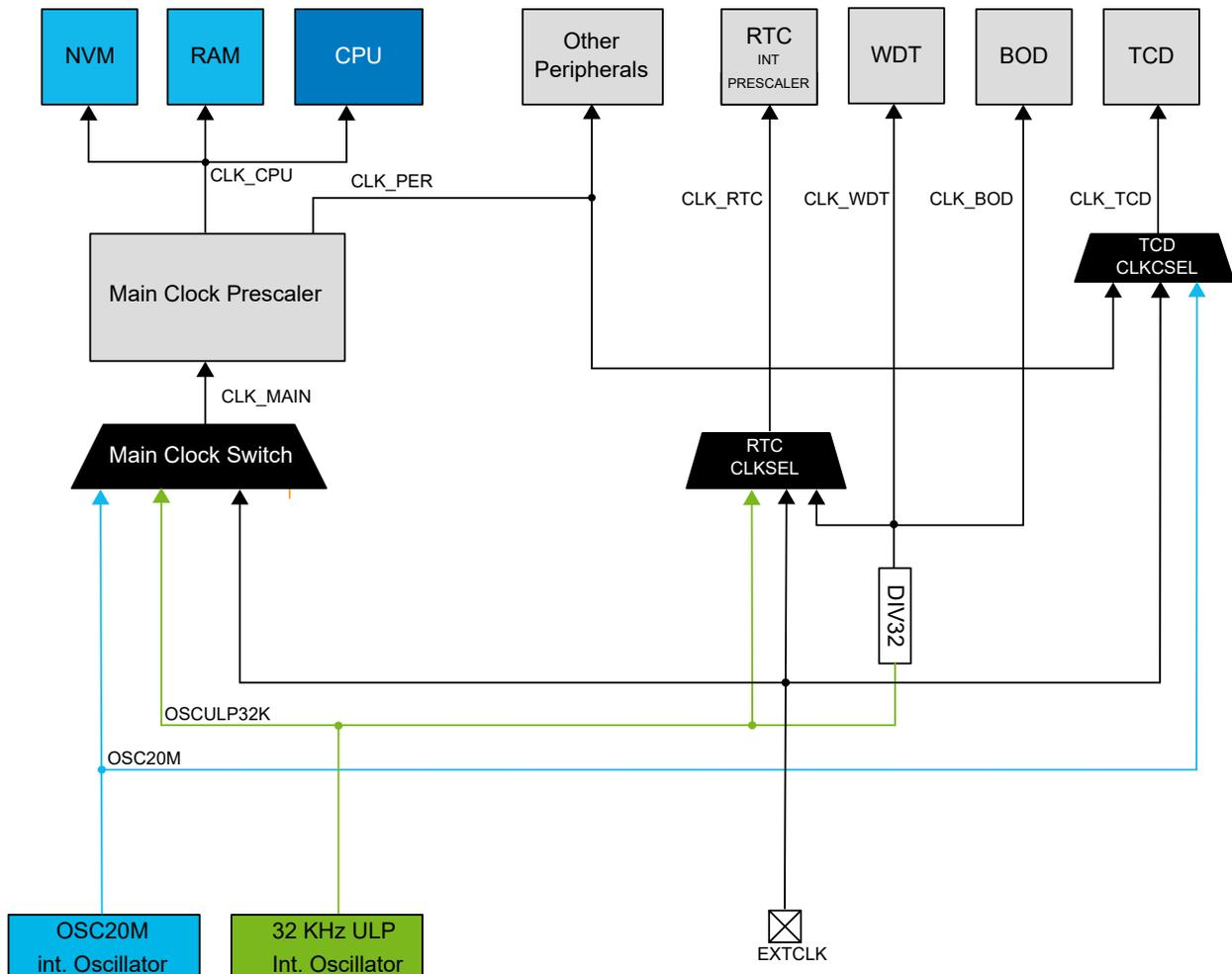
The clock system consists of the Main Clock and other asynchronous clocks:
