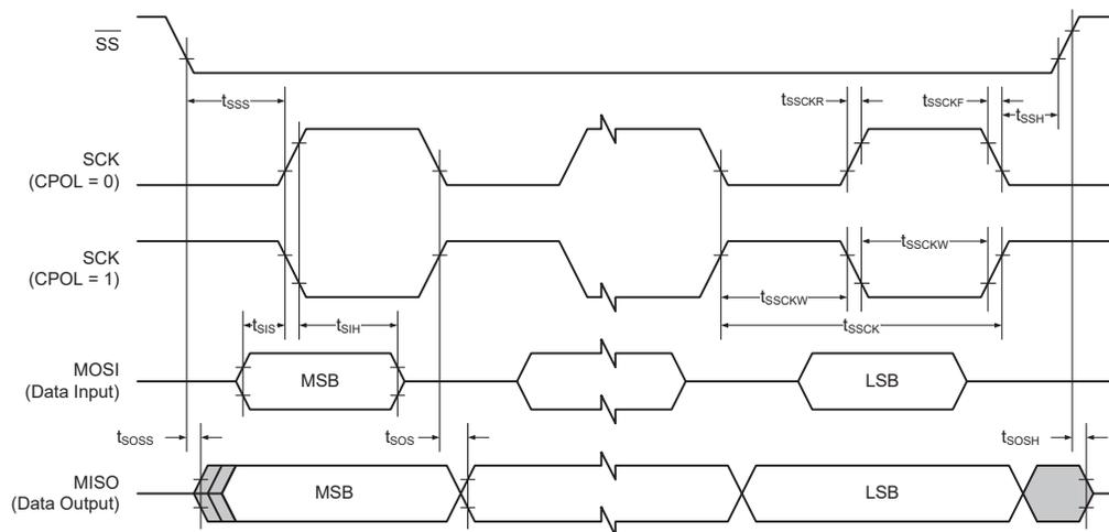
**Table 33-16. USART in SPI Mode - Timing Characteristics**
