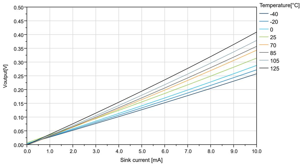
**Figure 34-23. IO Pin Output Voltage vs. Sink Current ( $V_{DD}=5.0V$ )**
