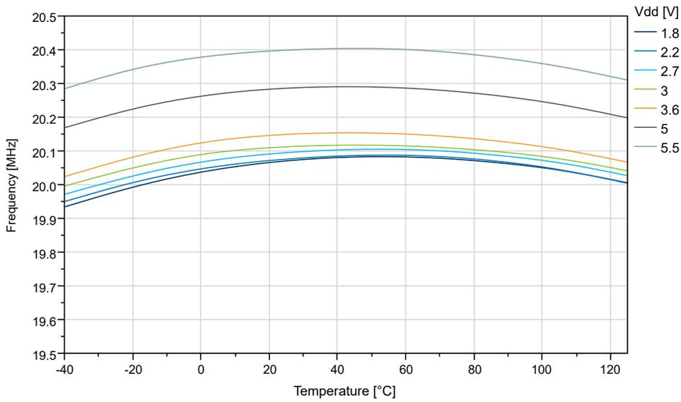
**Figure 34-59. OSC20M Internal Oscillator: Frequency vs.  $V_{DD}$**
