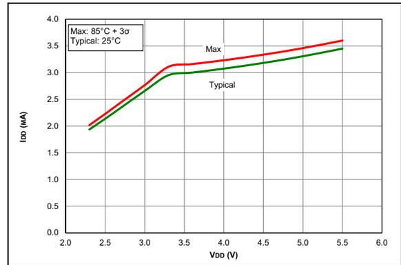
**FIGURE 38-4:**  $I_{DD}$ , HS Oscillator 32 MHz, PIC16F15324/44 Only.
