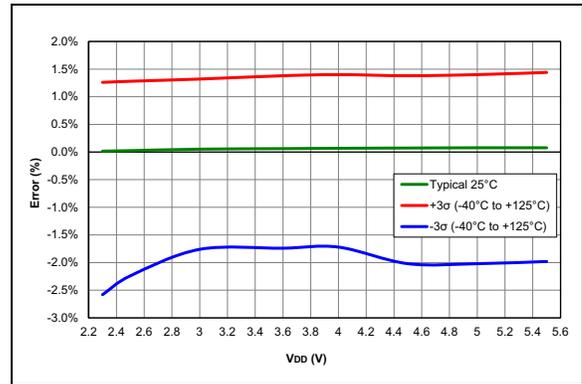
**FIGURE 38-28:** HFINTOSC Typical, Frequency Error, PIC16F15324/44 Only.
