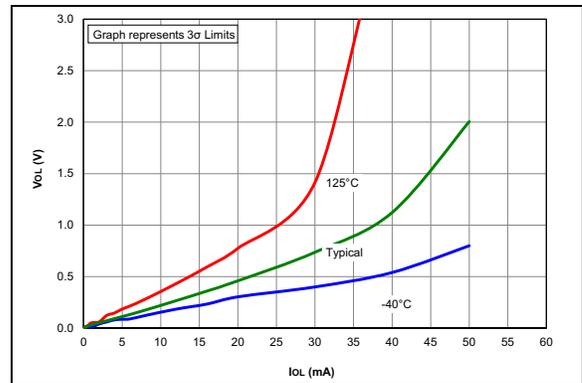
**FIGURE 38-35:**  $V_{OL}$  vs.  $I_{OL}$  Over Temperature,  $V_{DD} = 3.0V$ .
