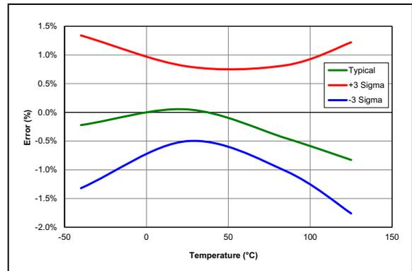
**FIGURE 38-29:** HFINTOSC Typical, Frequency Error,  $V_{DD} = 3.0V$ .
