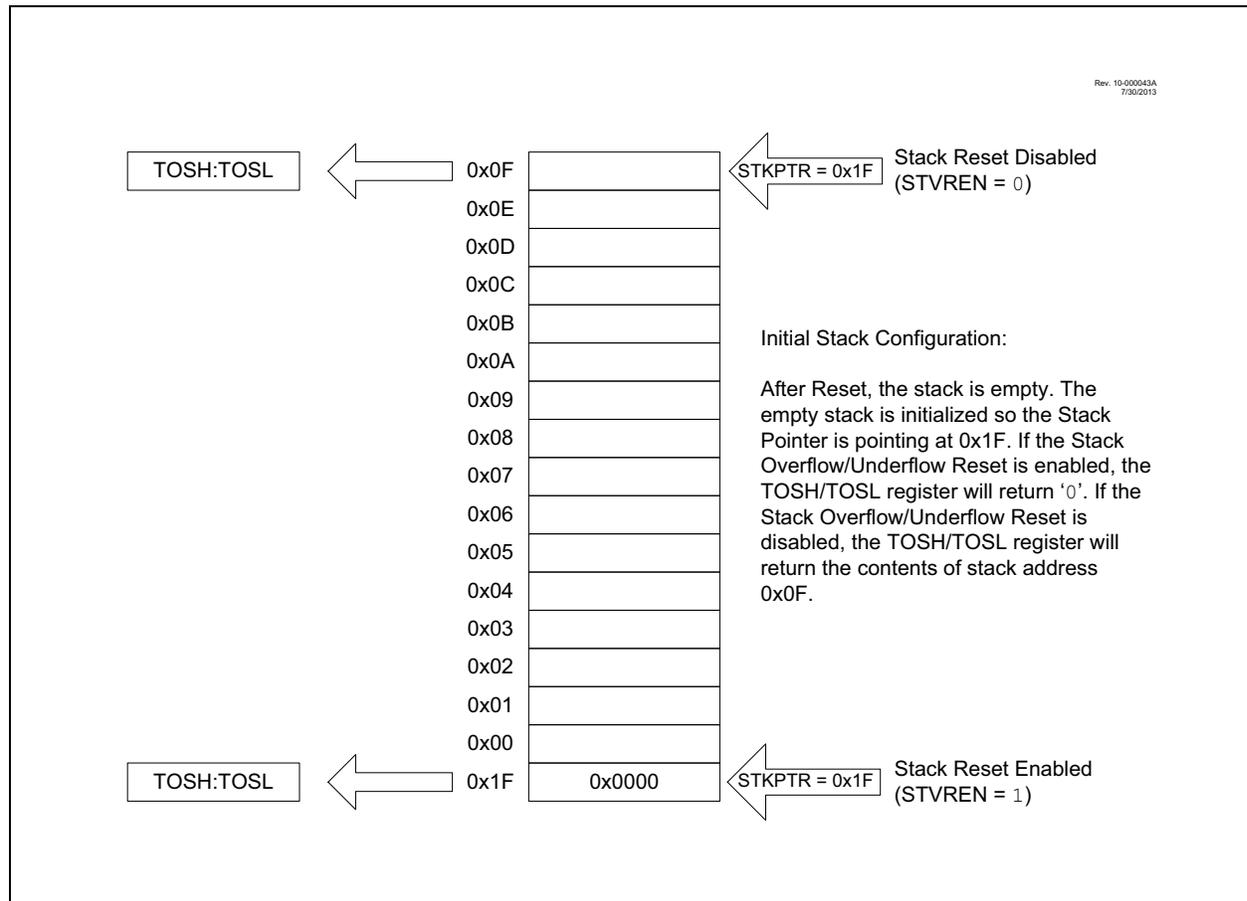
**FIGURE 4-5: ACCESSING THE STACK EXAMPLE 2**
