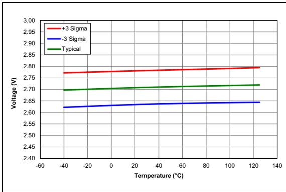
**FIGURE 38-38:** *Brown-Out Reset Voltage, Low Trip Point (BORV = 0).*
