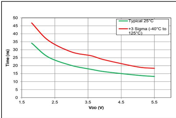
**FIGURE 38-101:** Rise Time, Slew Rate Control Enabled.
