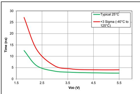
**FIGURE 38-103:** Rise Time, Slew Rate Control Disabled.
