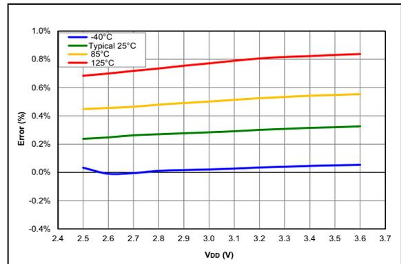
**FIGURE 38-95:** FVR Voltage Error 2x, PIC16LF15324/44 Only.
