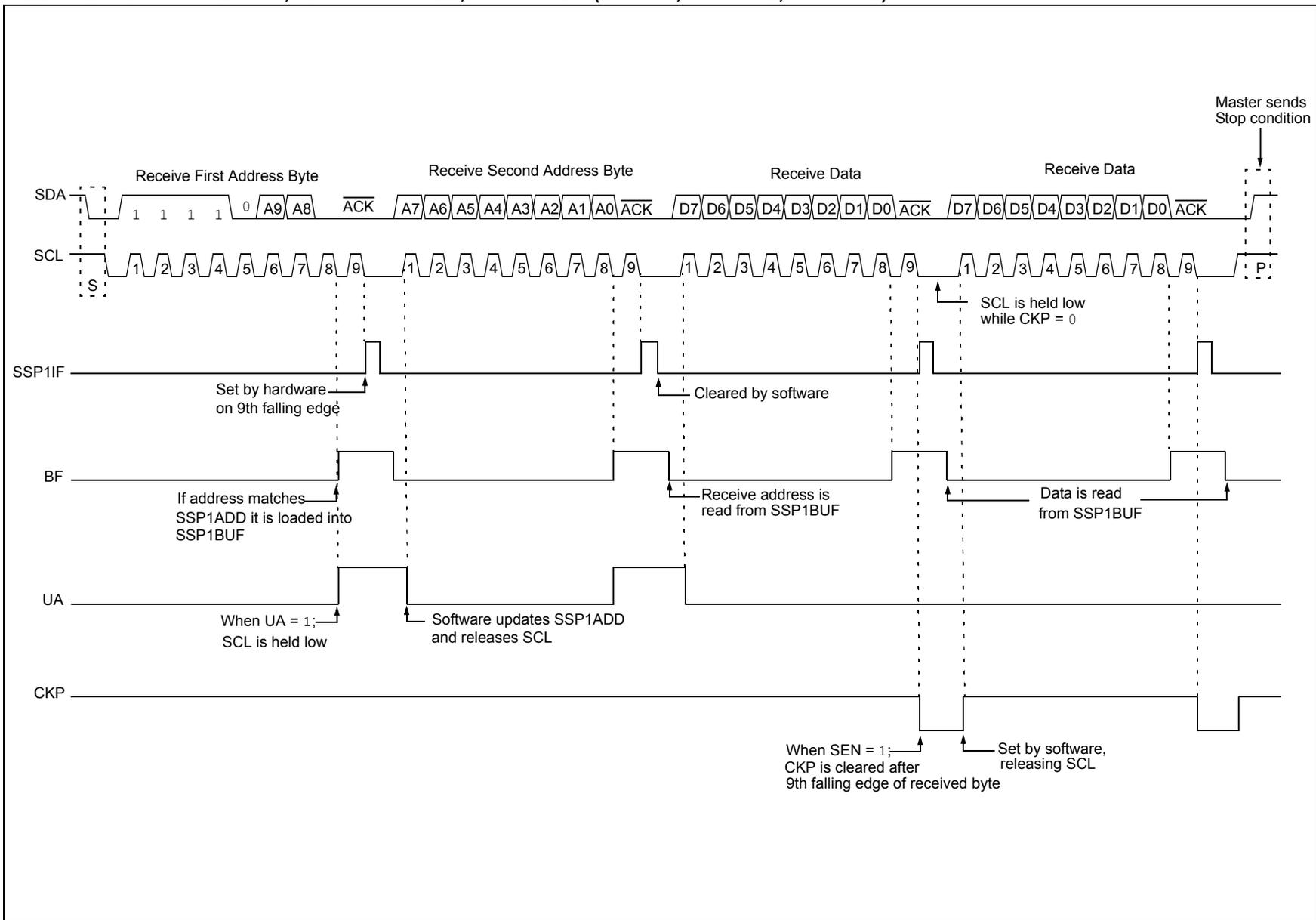
**FIGURE 32-21: I<sup>2</sup>C SLAVE, 10-BIT ADDRESS, RECEPTION (SEN = 0, AHEN = 1, DHEN = 0)**
