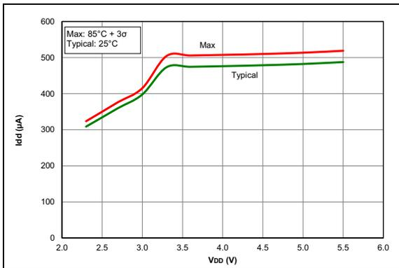
**FIGURE 38-2:**  $I_{DD}$ , XT Oscillator 4 MHz, PIC16F15324/44 Only.
