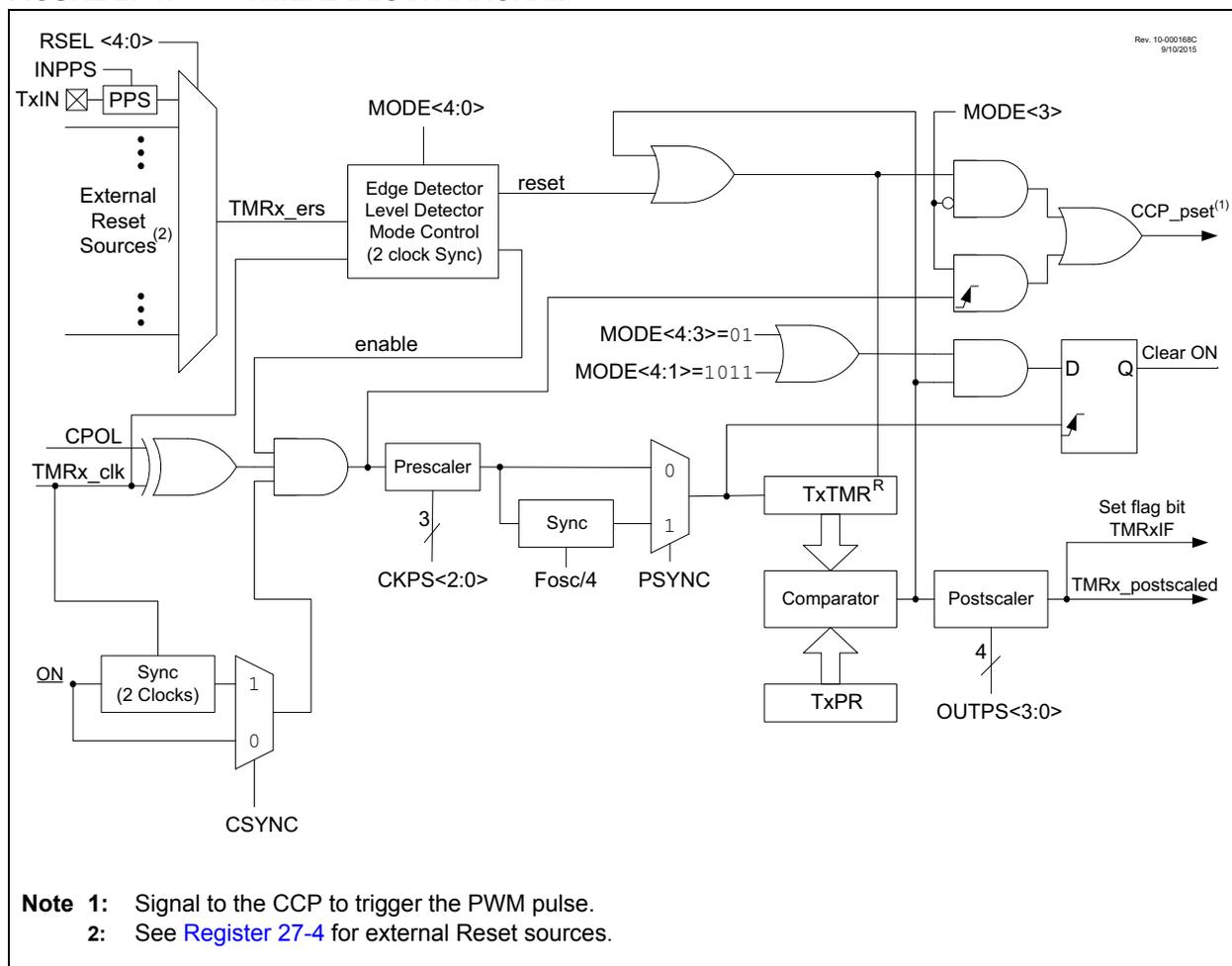
**FIGURE 27-2: TIMER2 CLOCK SOURCE BLOCK DIAGRAM**
