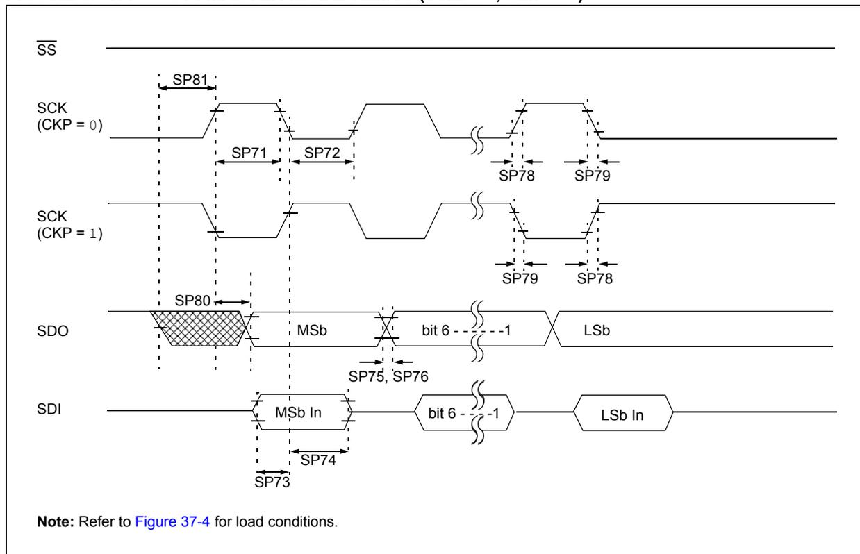
**FIGURE 37-18: SPI MASTER MODE TIMING (CKE = 1, SMP = 1)**
