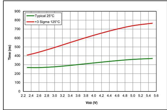
**FIGURE 38-88:** Comparator Response Time Rising Edge, PIC16F15324/44 Only.
