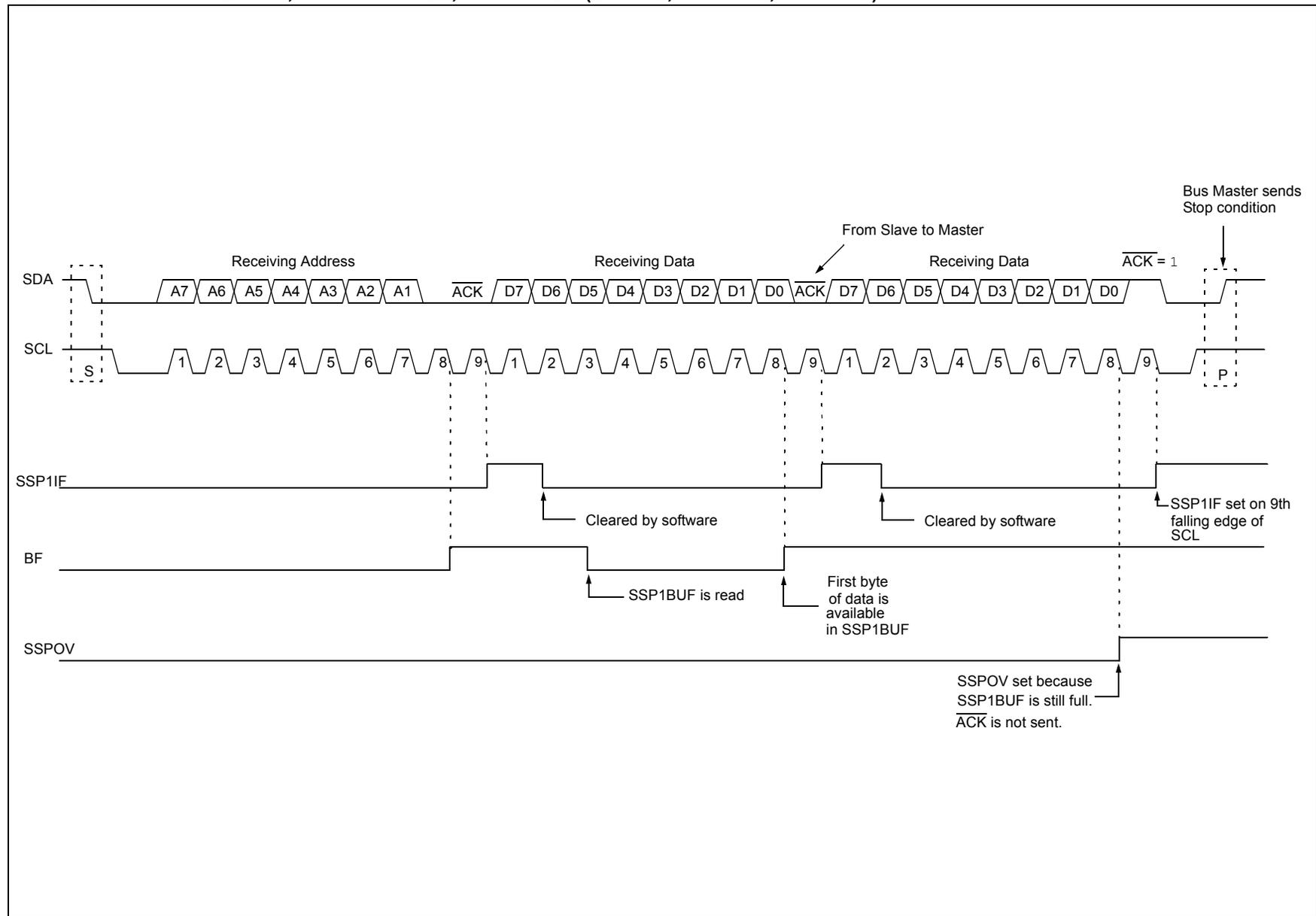
**FIGURE 32-15: I<sup>2</sup>C SLAVE, 7-BIT ADDRESS, RECEPTION (SEN = 1, AHEN = 0, DHEN = 0)**
