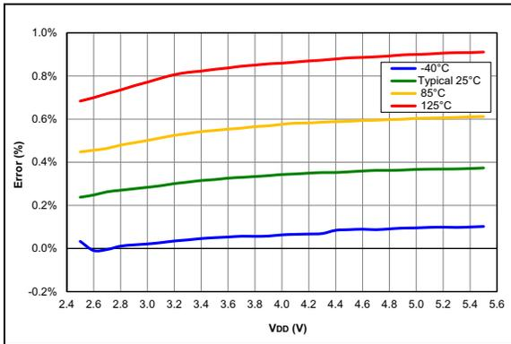
**FIGURE 38-96:** FVR Voltage Error 2x, PIC16F15324/44 Only.
