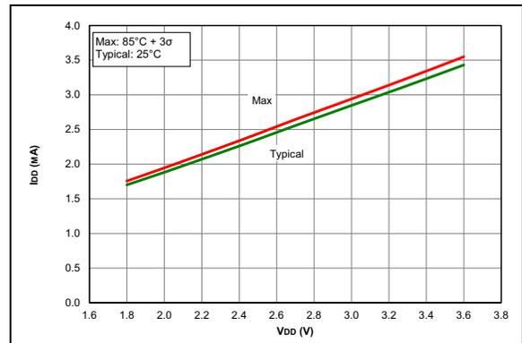
**FIGURE 38-5:**  $I_{DD}$ , HFINTOSC Mode, FOSC = 32 MHz, PIC16LF15324/44 Only.
