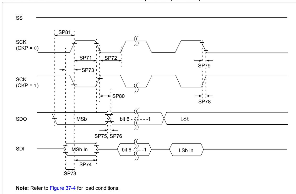
**FIGURE 37-19: SPI SLAVE MODE TIMING (CKE = 0)**
