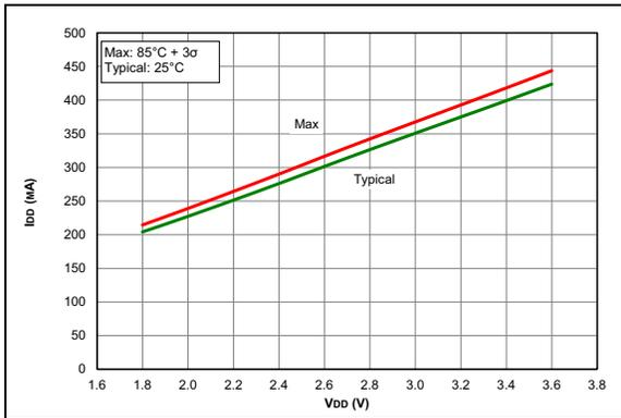
**FIGURE 38-1:**  $I_{DD}$ , XT Oscillator 4 MHz, PIC16LF15324/44 Only.
