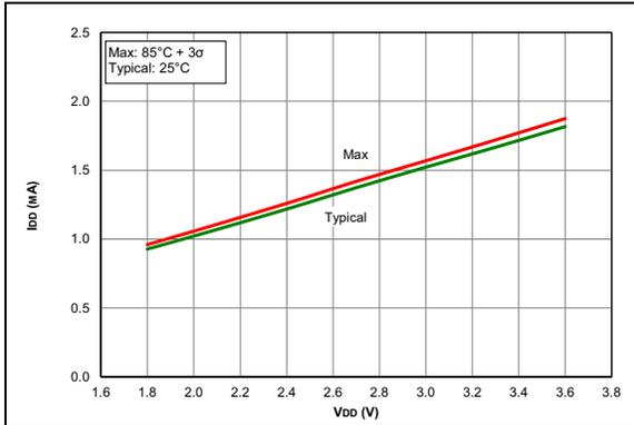
**FIGURE 38-7:**  $I_{DD}$ , HFINTOSC Mode,  $F_{osc} = 16$  MHz, PIC16LF15324/44 Only.
