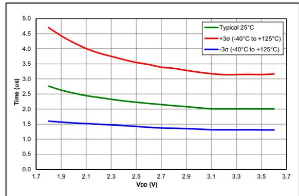
**FIGURE 38-66:** ADC RC Oscillator Period, PIC16LF15324/44 Only.
