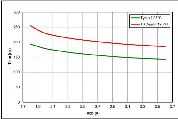
**FIGURE 38-85:** Comparator Response Time Falling Edge, PIC16LF15324/44 Only.
