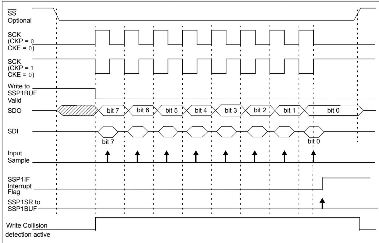
**FIGURE 32-10: SPI MODE WAVEFORM (SLAVE MODE WITH CKE = 1)**
