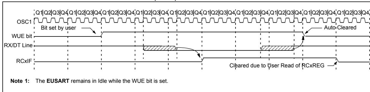
**FIGURE 33-8: AUTO-WAKE-UP BIT (WUE) TIMINGS DURING SLEEP**
