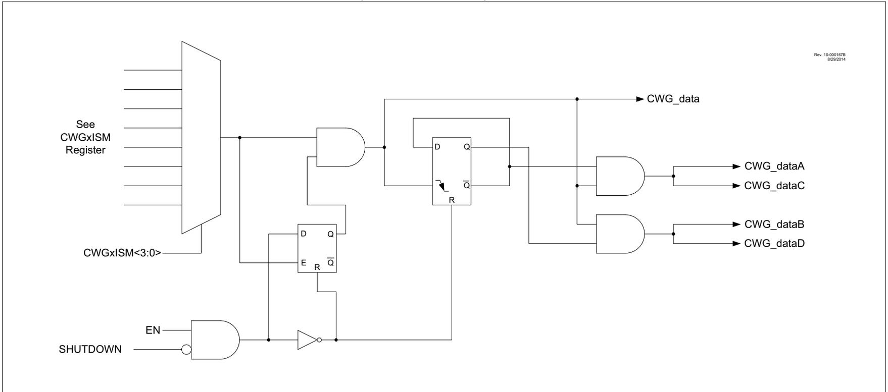
**FIGURE 30-3: SIMPLIFIED CWG BLOCK DIAGRAM (FORWARD AND REVERSE FULL-BRIDGE MODES)**
