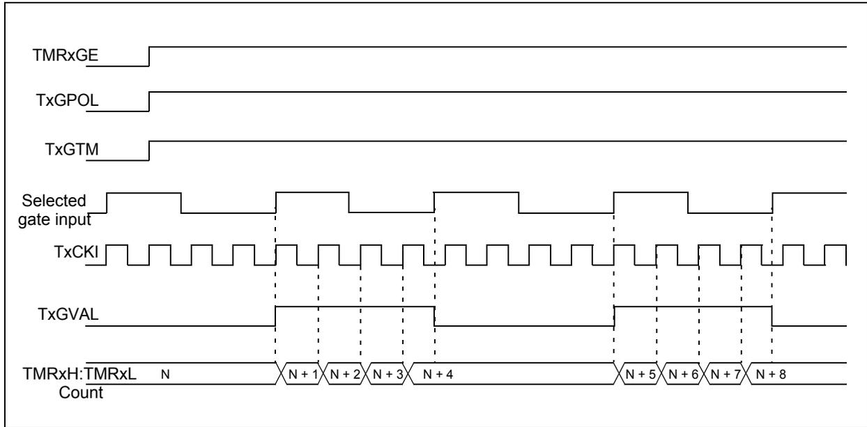
**FIGURE 26-5: TIMER1 GATE SINGLE-PULSE MODE**
