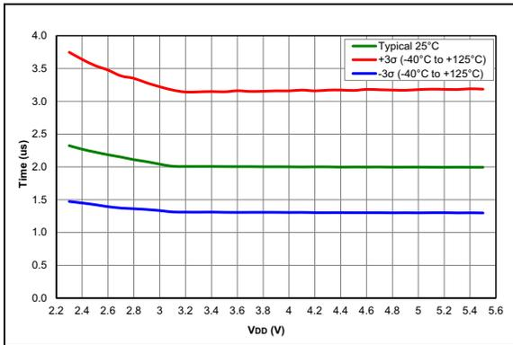
**FIGURE 38-67:** ADC RC Oscillator Period, PIC16F15324/44 Only.
