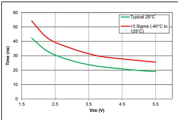
**FIGURE 38-102:** Fall Time, Slew Rate Control Enabled.
