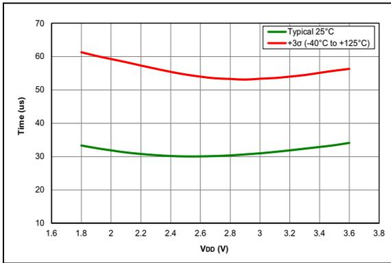
**FIGURE 38-91:** Band Gap Ready Time, PIC16LF15324/44 Only.
