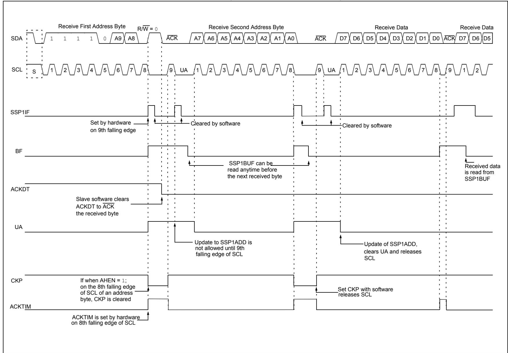
**FIGURE 32-22: I<sup>2</sup>C SLAVE, 10-BIT ADDRESS, TRANSMISSION (SEN = 0, AHEN = 0, DHEN = 0)**
