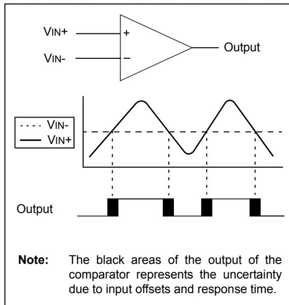
**FIGURE 23-2: COMPARATOR MODULE SIMPLIFIED BLOCK DIAGRAM**
