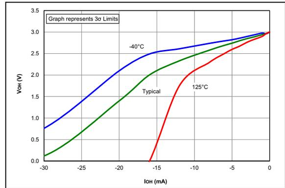
**FIGURE 38-34:**  $V_{OH}$  vs.  $I_{OH}$  Over Temperature,  $V_{DD} = 3.0V$ .
