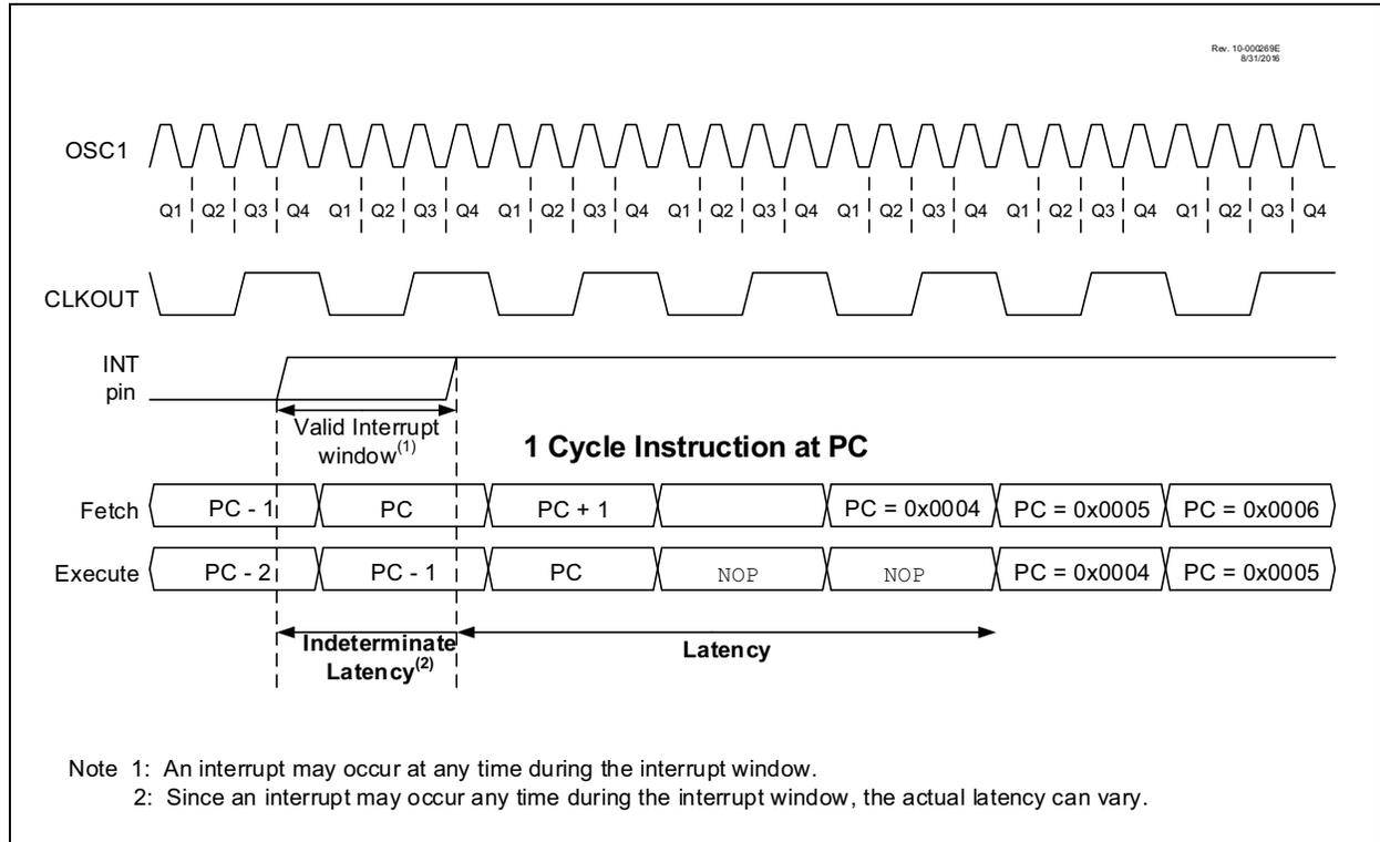
**FIGURE 10-3: INT PIN INTERRUPT TIMING**
