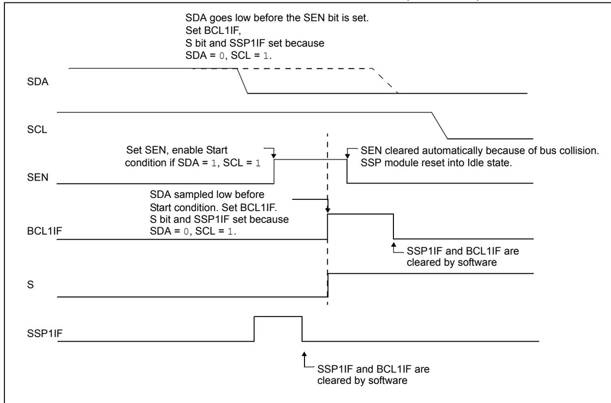
**FIGURE 32-34: BUS COLLISION DURING START CONDITION (SCL = 0)**
