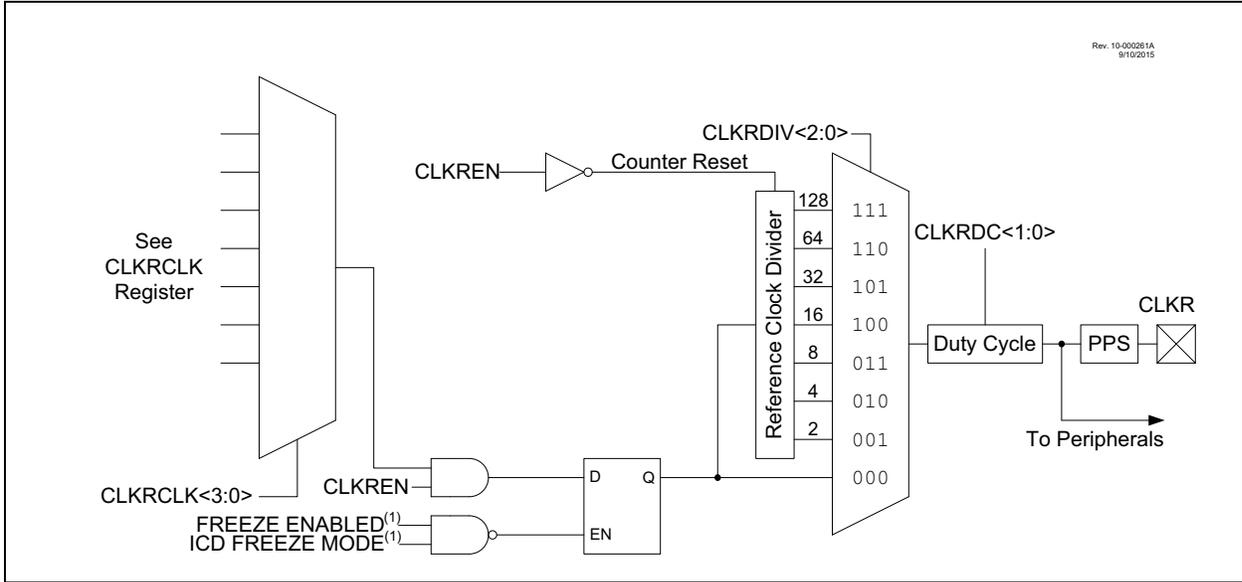
**FIGURE 34-2: CLOCK REFERENCE TIMING**
