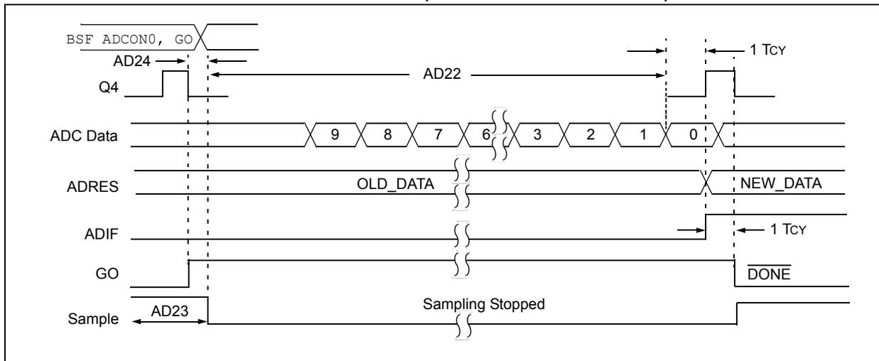
**FIGURE 37-11: ADC CONVERSION TIMING (ADC CLOCK FROM ADCRC)**
