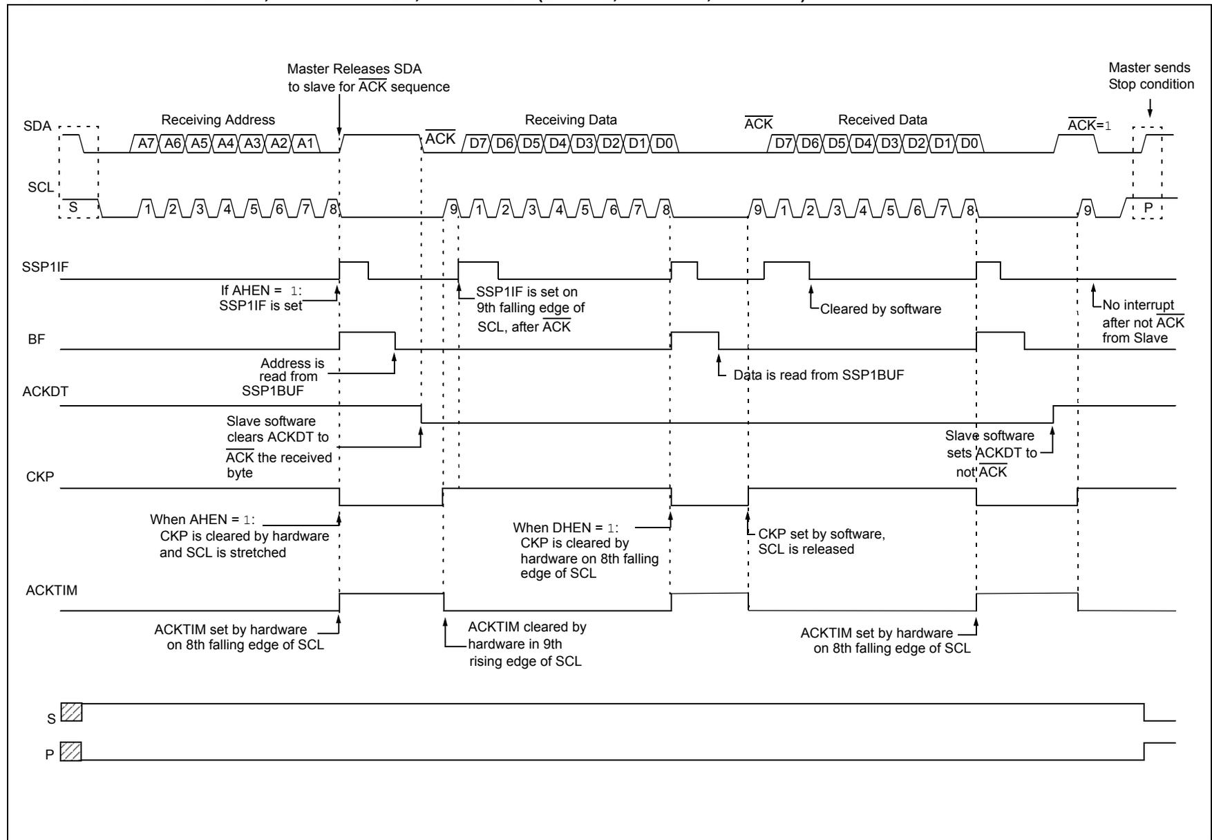
**FIGURE 32-17: I<sup>2</sup>C SLAVE, 7-BIT ADDRESS, RECEPTION (SEN = 1, AHEN = 1, DHEN = 1)**
