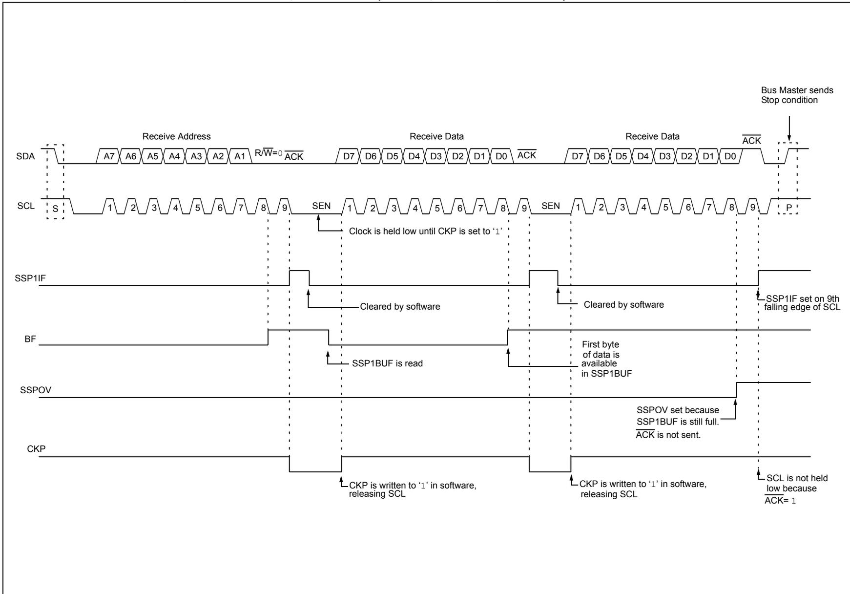
**FIGURE 32-16: I<sup>2</sup>C SLAVE, 7-BIT ADDRESS, RECEPTION (SEN = 0, AHEN = 1, DHEN = 1)**
