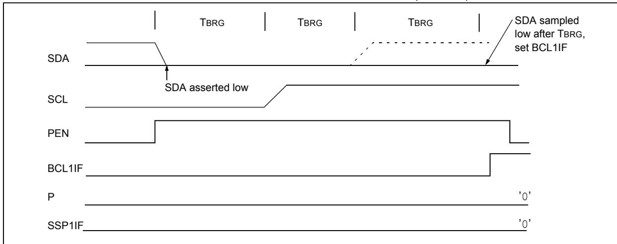
**FIGURE 32-39: BUS COLLISION DURING A STOP CONDITION (CASE 2)**
