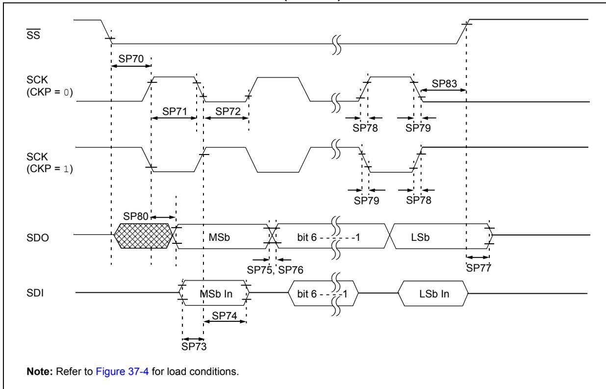
**FIGURE 37-20: SPI SLAVE MODE TIMING (CKE = 1)**
