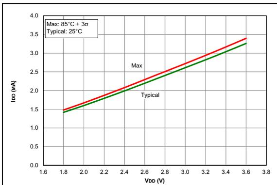
**FIGURE 38-3:**  $I_{DD}$ , HS Oscillator 32 MHz, PIC16LF15324/44 Only.
