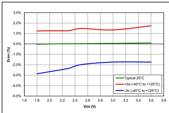
**FIGURE 38-27:** HFINTOSC Typical, Frequency Error, PIC16LF15324/44 Only.
