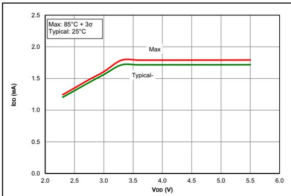
**FIGURE 38-8:**  $I_{DD}$ , HFINTOSC Mode,  $F_{osc} = 16$  MHz, PIC16F15324/44 Only.
