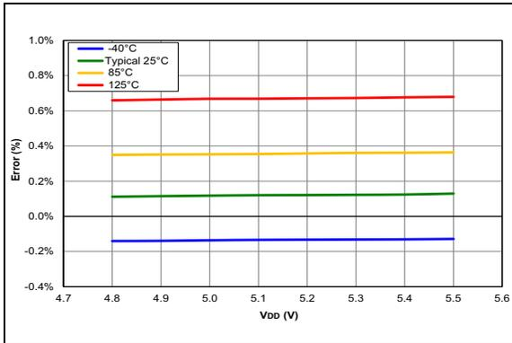
**FIGURE 38-97:** FVR Voltage Error 4x, PIC16F15324/44 Only.
