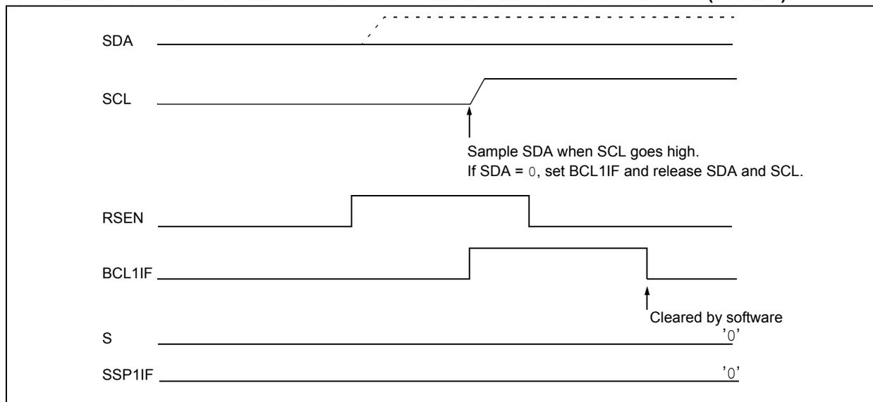
**FIGURE 32-37: BUS COLLISION DURING REPEATED START CONDITION (CASE 2)**
