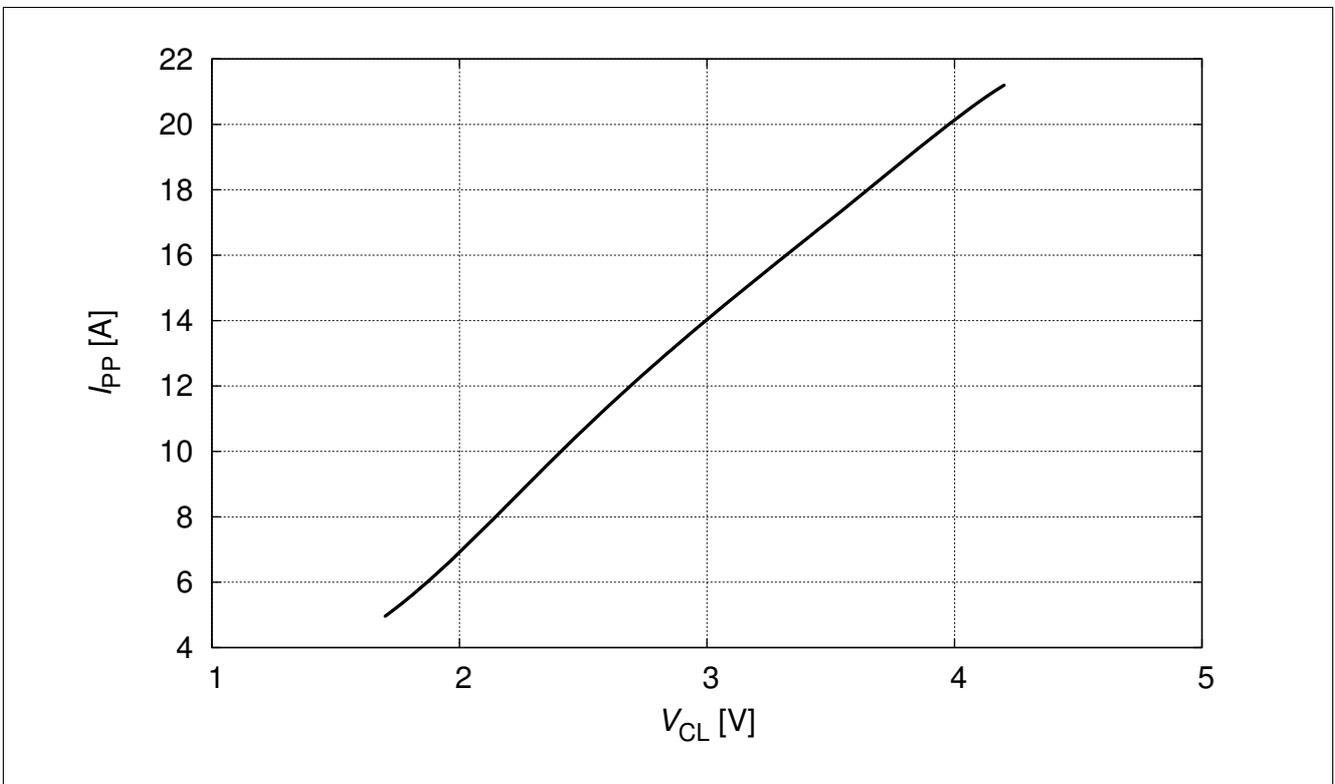
Figure 3-6 Pulse forward current (IEC61000-4-5) versus clamping voltage,  $I_{PP} = f(V_{CL})$
