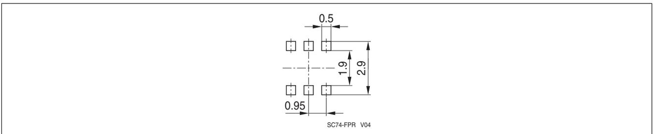
Figure 4-2 SC74 Footprint (Reflow Soldering)
