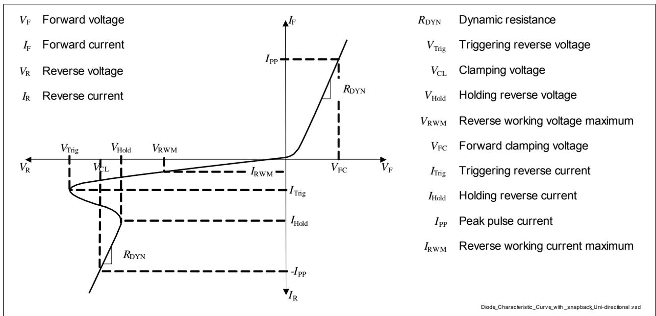
**Figure 2-1 Definitions of electrical characteristics**
