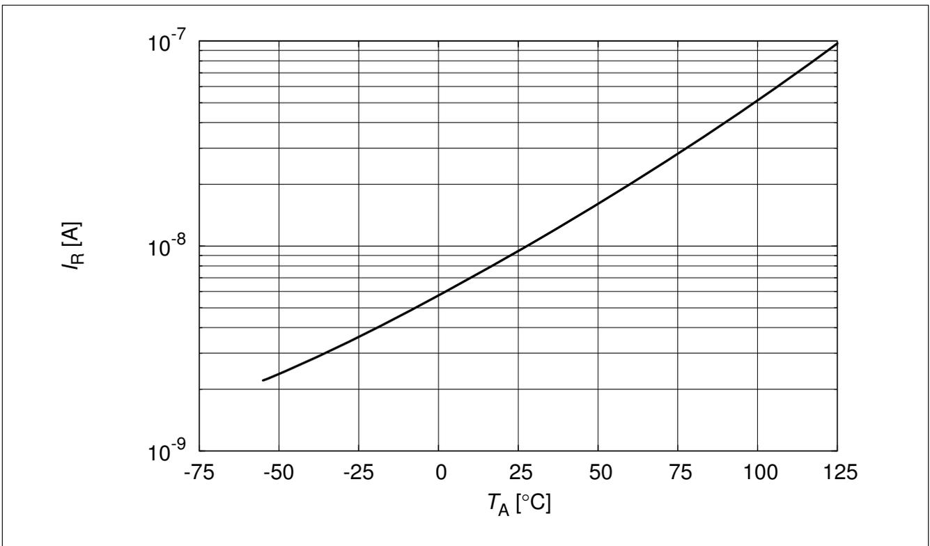
Figure 3-4 Reverse current  $I_R = f(T_A)$ ,  $V_R = 3.3$  V
