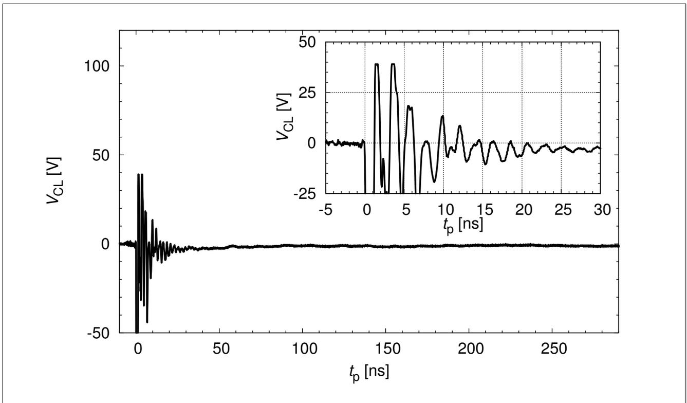
Figure 3-10 Clamping voltage at -8 kV contact discharge according IEC61000-4-2 ( $R = 330 \Omega$ ,  $C = 150 \text{ pF}$ )
