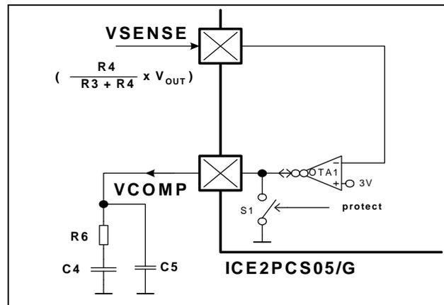
Figure 4 Startup Circuit
