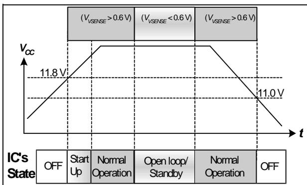
Figure 3 State of Operation respect to VCC
