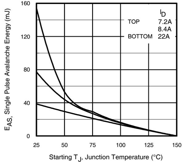
**Fig 13c.** Maximum Avalanche Energy Vs. Drain Current
