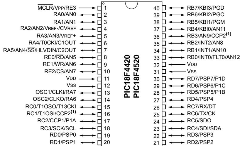
Note 1: RB3 is the alternate pin for CCP2 multiplexing.
