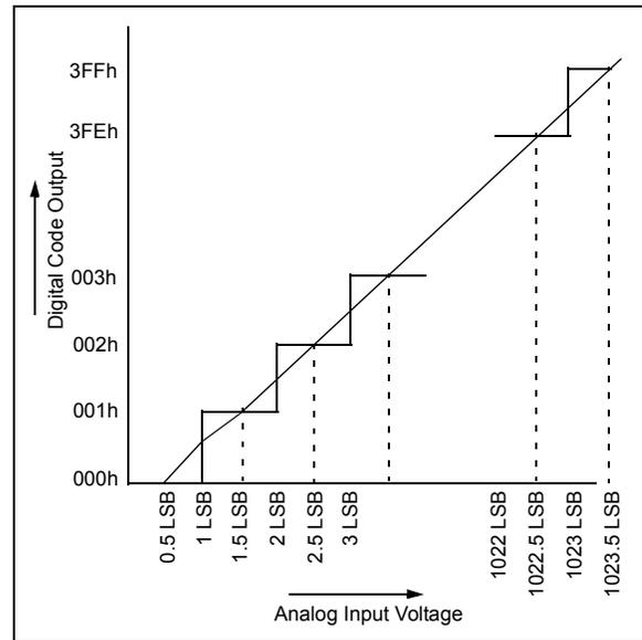
**FIGURE 19-3: ANALOG INPUT MODEL**
