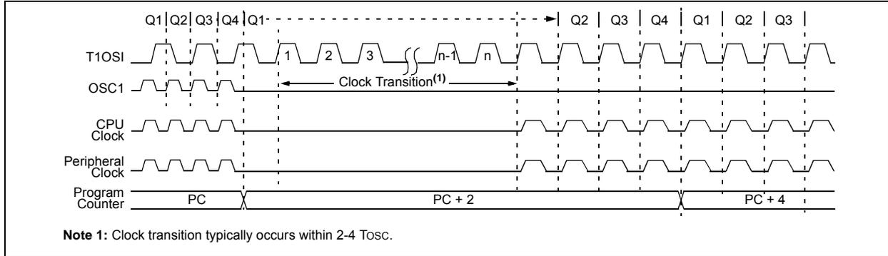
**FIGURE 3-2: TRANSITION TIMING FROM SEC\_RUN MODE TO PRI\_RUN MODE (HSPLL)**
