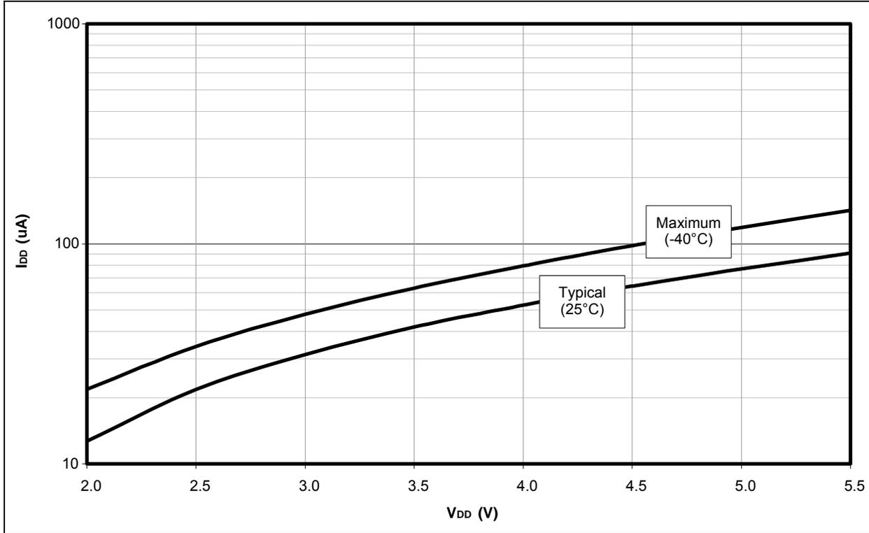
FIGURE 27-14: TYPICAL I<sub>DD</sub> ACROSS V<sub>DD</sub> (RC\_IDLE MODE, +25°C)
