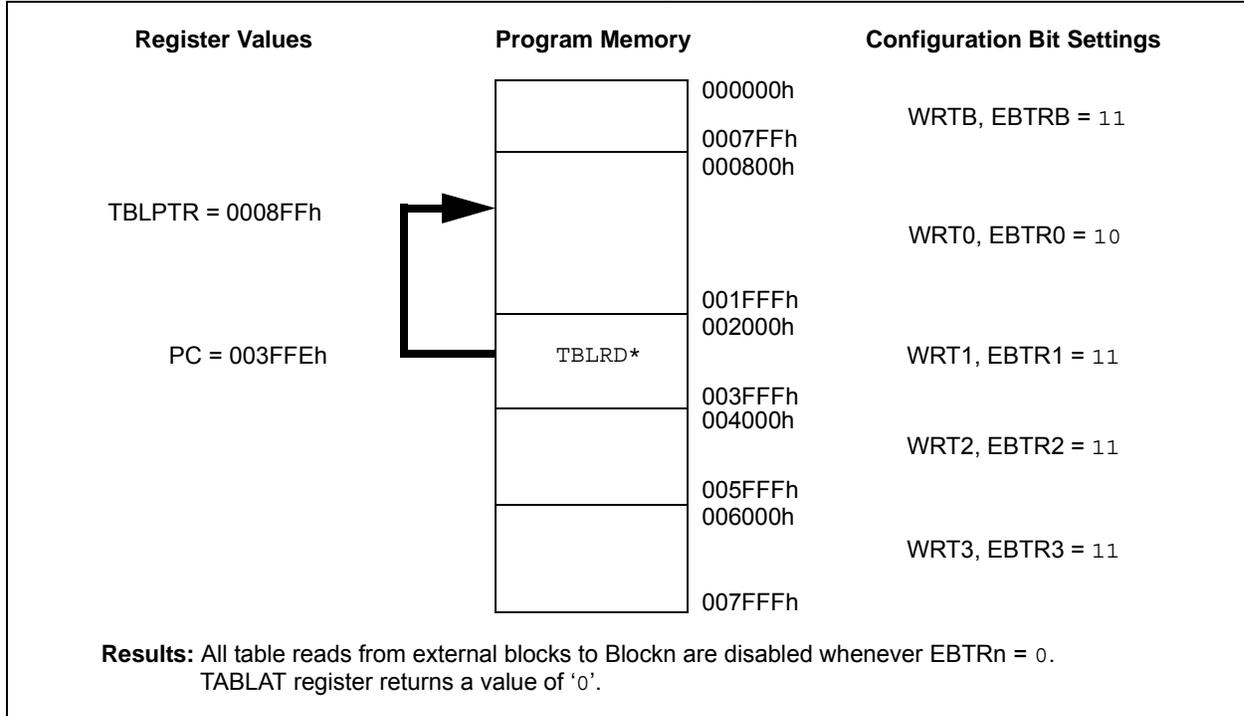
**FIGURE 23-8: EXTERNAL BLOCK TABLE READ (EBTRn) ALLOWED**
