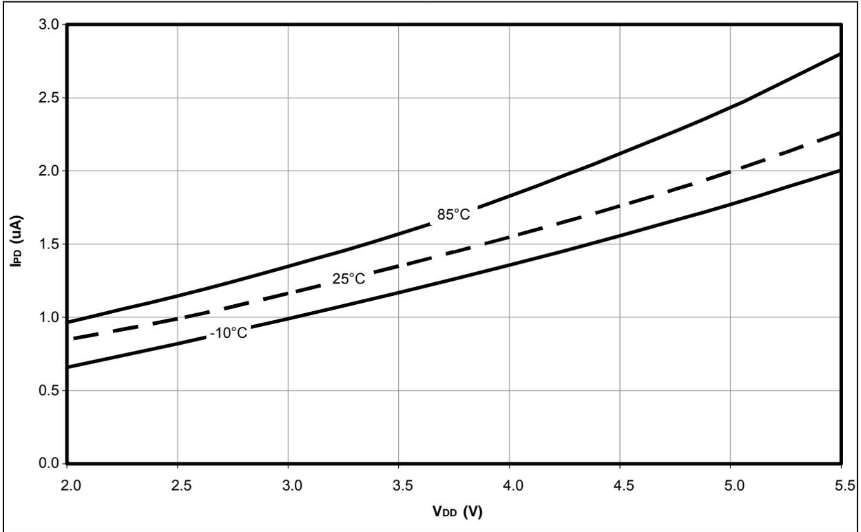
**FIGURE 27-5: MAXIMUM T1OSC DELTA CURRENT vs. V<sub>DD</sub> ACROSS TEMP. (DEVICE IN SLEEP, T1OSC IN LOW-POWER MODE)**
