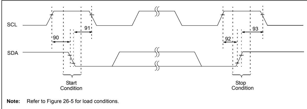
**TABLE 26-18: I<sup>2</sup>C™ BUS START/STOP BITS REQUIREMENTS (SLAVE MODE)**
