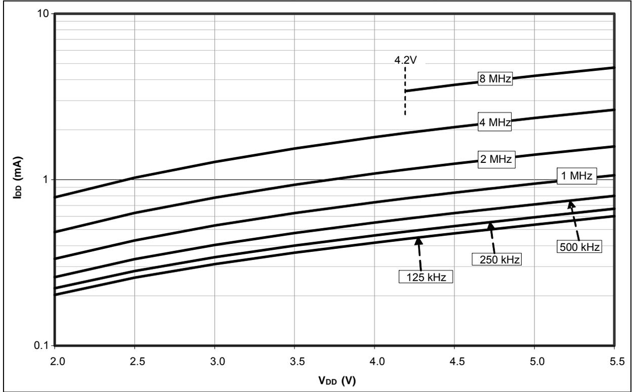
FIGURE 27-12: MAXIMUM  $I_{DD}$  ACROSS  $V_{DD}$  (RC\_RUN MODE, +85°C)
