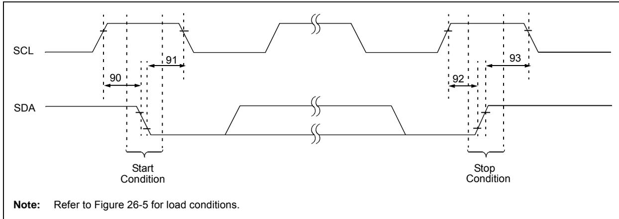
**TABLE 26-20: MASTER SSP I<sup>2</sup>C™ BUS START/STOP BITS REQUIREMENTS**
