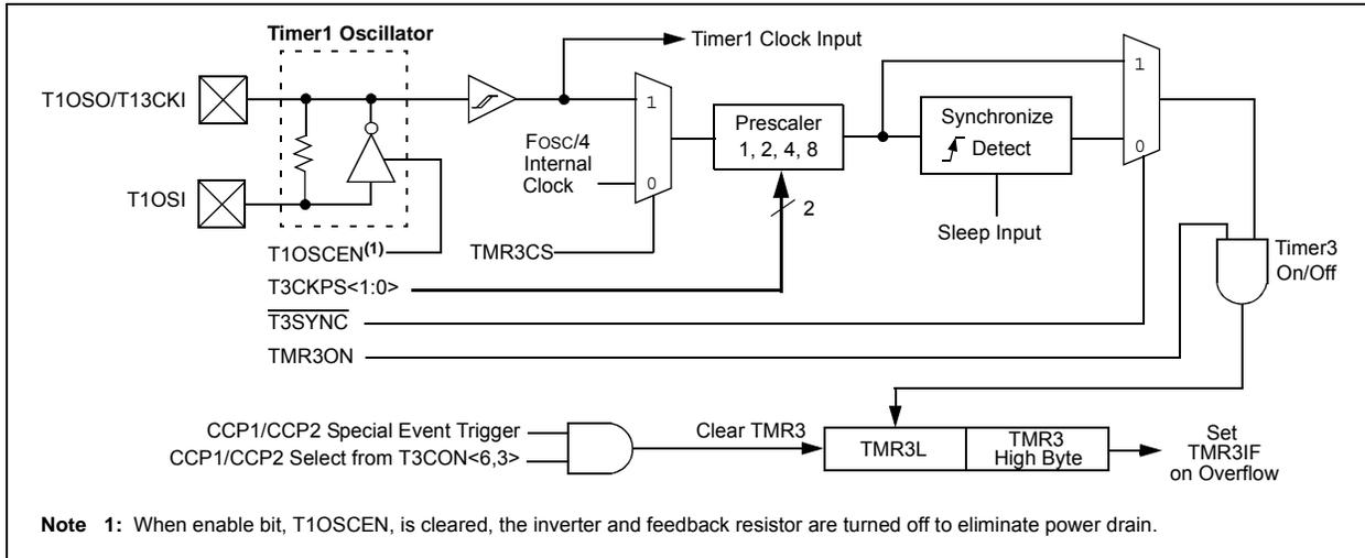
**FIGURE 14-2: TIMER3 BLOCK DIAGRAM (16-BIT READ/WRITE MODE)**
