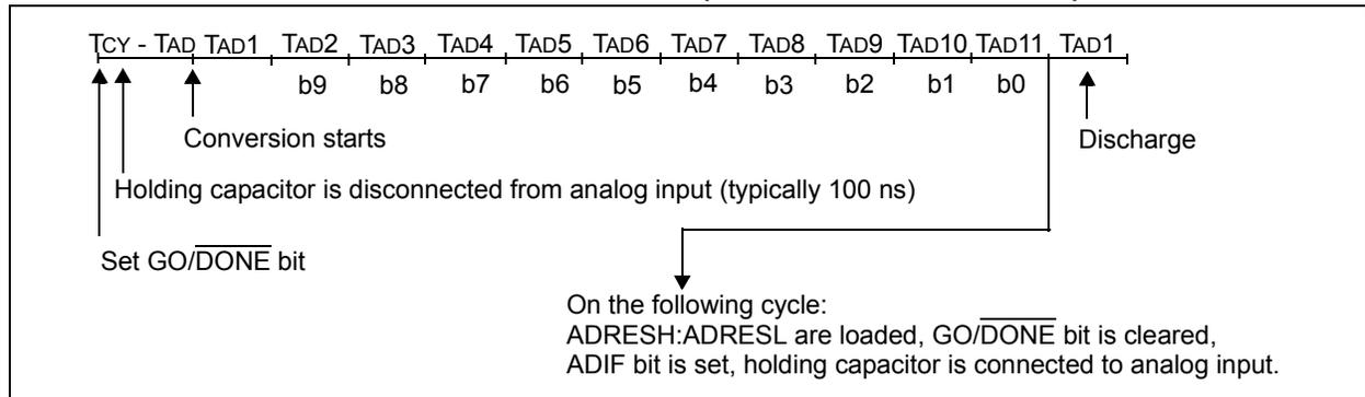
**FIGURE 19-5: A/D CONVERSION TAD CYCLES ( $\text{ACQT}<2:0> = 010, \text{TACQ} = 4 \text{TAD}$ )**
