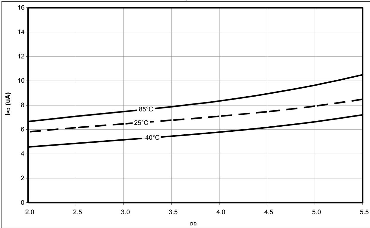
**FIGURE 27-7: MAXIMUM T1OSC DELTA CURRENT vs. V<sub>DD</sub> ACROSS TEMP. (DEVICE IN SLEEP, T1OSC IN HIGH-POWER MODE)**
