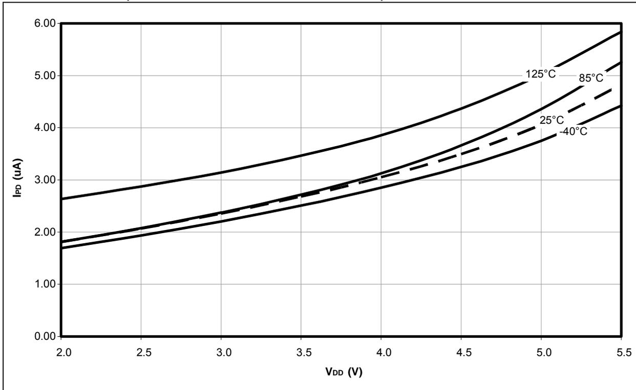
**FIGURE 27-10: MAXIMUM WDT CURRENT vs. V<sub>DD</sub> ACROSS TEMPERATURE (WDT DELTA CURRENT IN SLEEP MODE)**
