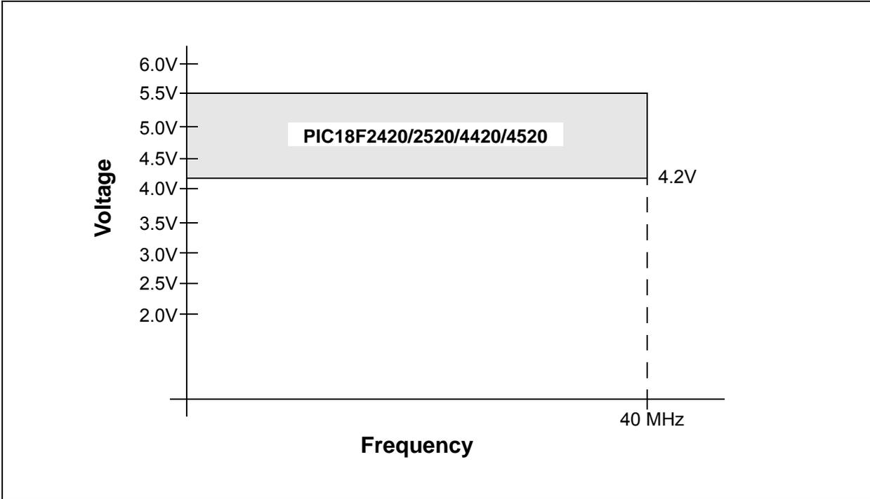
FIGURE 26-2: PIC18F2420/2520/4420/4520 VOLTAGE-FREQUENCY GRAPH (EXTENDED)
