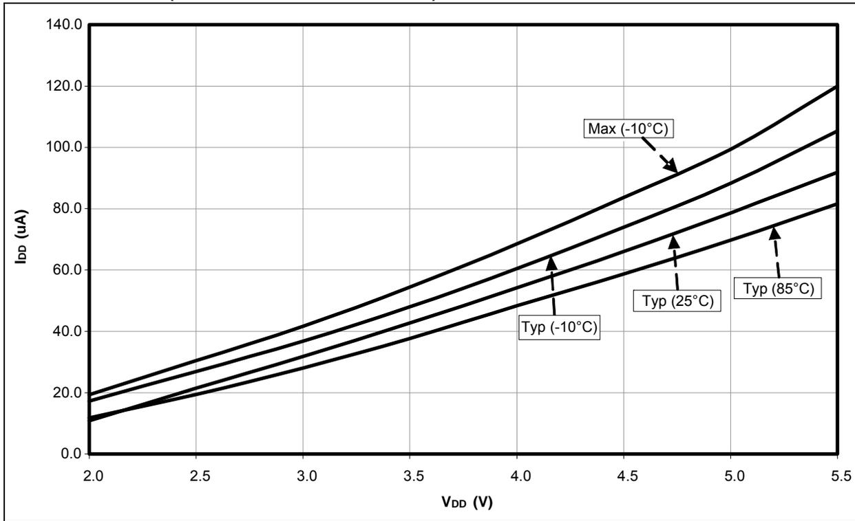
FIGURE 27-18: TYPICAL AND MAXIMUM SEC\_IDLE CURRENT vs. V<sub>DD</sub> ACROSS TEMPERATURE (T<sub>1OSC</sub> IN LOW-POWER MODE)
