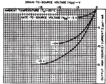
Fig. 7 - Minimum output high (source) current characteristics.
