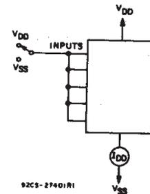
Fig. 11 - Quiescent device current test circuit.
