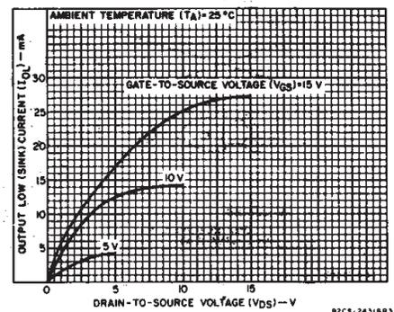
Fig. 2 - Typical output low (sink) current characteristics.
