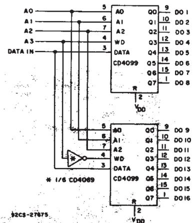
Fig. 14 - 1-of-16 decoder/demultiplexer.
