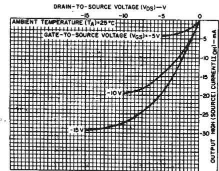
Fig. 6 - Typical output high (source) current characteristics.
