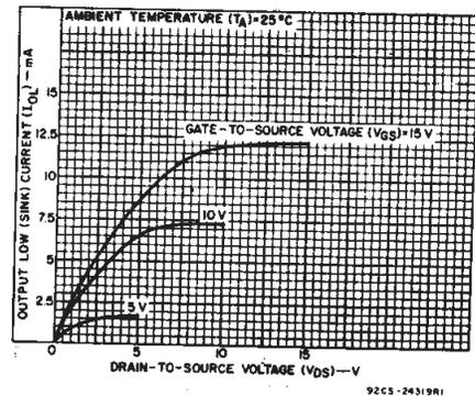
Fig. 4 - Minimum output low (sink) current characteristics.
