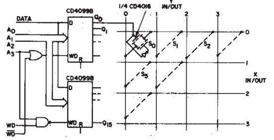
Fig. 16 - Multiple selection decoding - 4 x 4 crosspoint switch.
