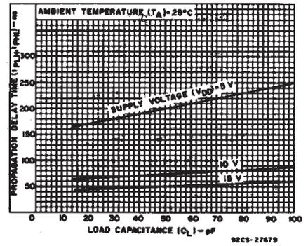
Fig. 8 - Typical propagation delay time (data to Q<sub>n</sub>) vs. load capacitance.
