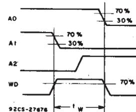
Fig. 3 - Definition of WRITE DISABLE ON time.
