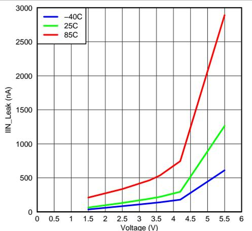
Figure 5. Input Current, Leak vs Input Voltage
