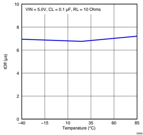
Figure 25. Turn-off Time vs Temperature
