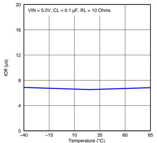
**Figure 34. Turn-off Time vs Temperature**
