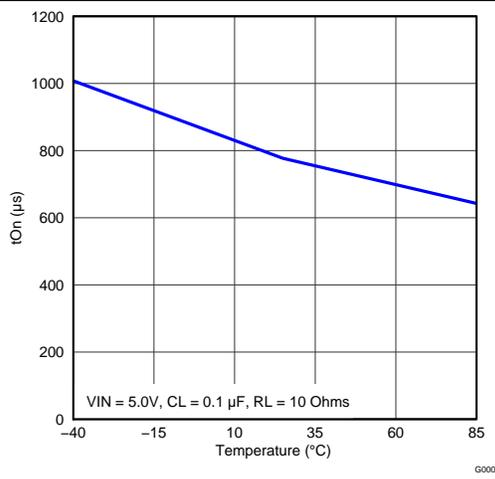
**Figure 42. Turn-on Time vs Temperature**
