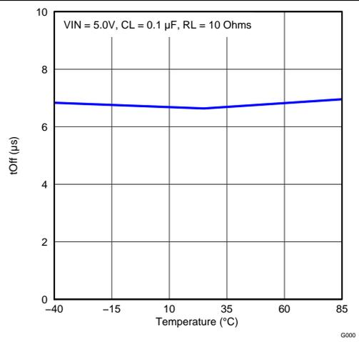
**Figure 43. Turn-Off Time vs Temperature**
