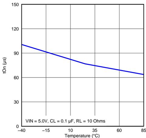
**Figure 33. Turn-on Time vs Temperature**
