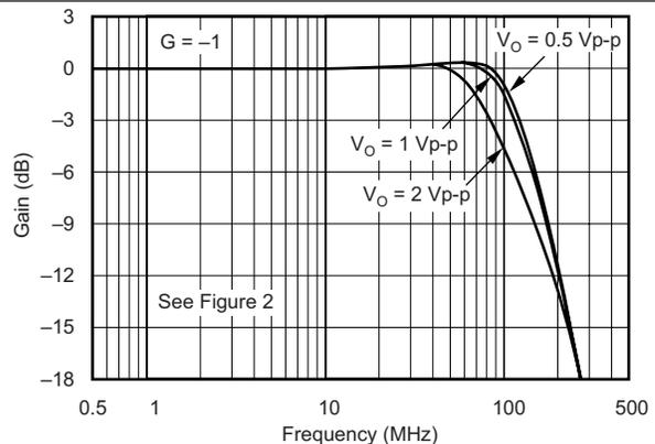
Figure 4. Inverting Large-Signal Frequency Response
