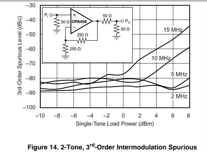
**Figure 14. 2-Tone, 3<sup>rd</sup>-Order Intermodulation Spurious**
