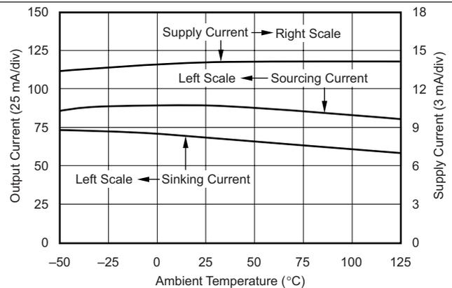
Figure 22. Supply and Output Current vs Temperature
