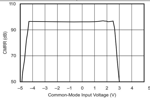
**Figure 27. Common-Mode Rejection Ratio vs Common-Mode Input Voltage**
