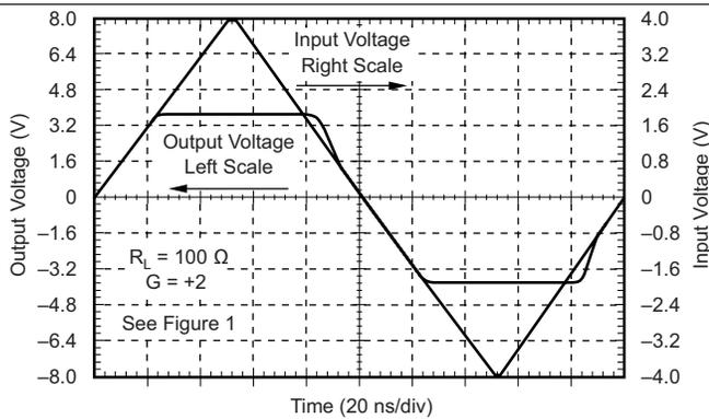
Figure 23. Noninverting Input Overdrive Recovery
