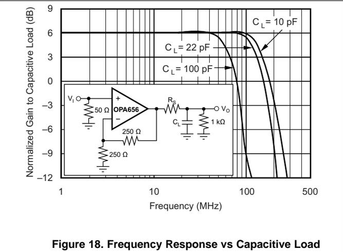
**Figure 18. Frequency Response vs Capacitive Load**
