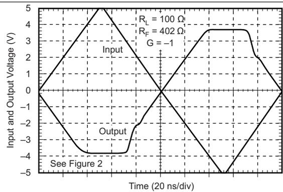
Figure 24. Inverting Overdrive Recovery
