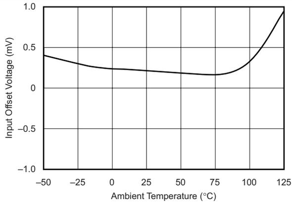
Figure 19. Typical Input Offset Voltage Over Temperature
