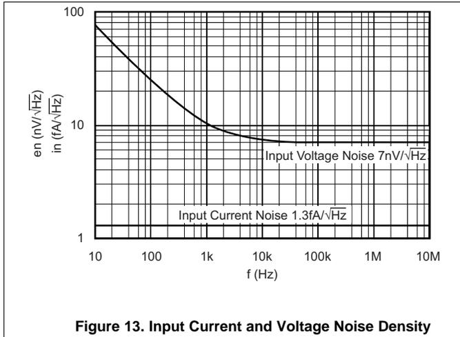
**Figure 13. Input Current and Voltage Noise Density**
