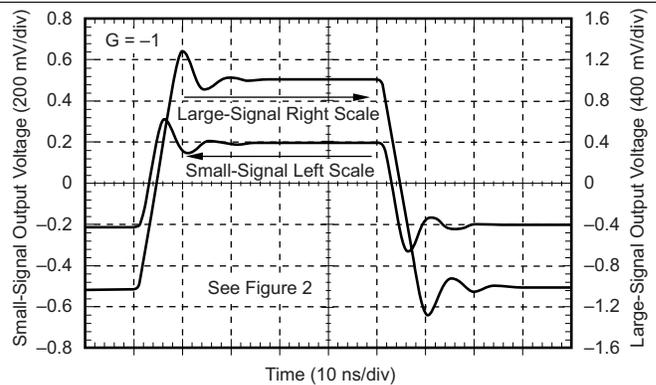
Figure 6. Inverting Pulse Response
