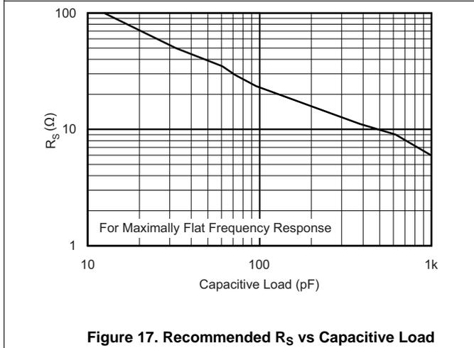
**Figure 17. Recommended  $R_S$  vs Capacitive Load**
