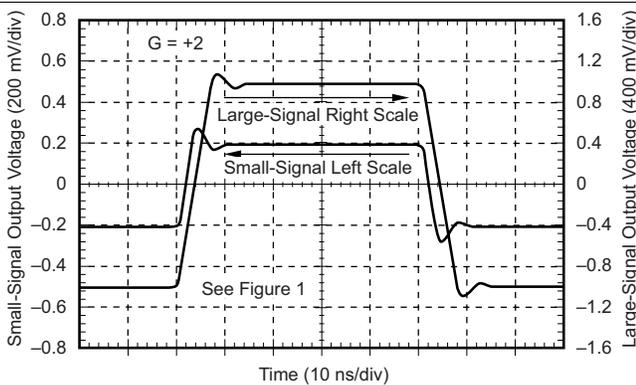
Figure 5. Noninverting Pulse Response
