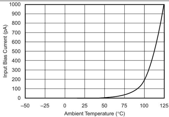
Figure 21. Typical Input Bias Current Over Temperature
