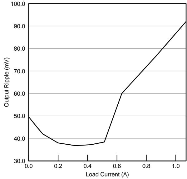
Figure 11. Output Ripple vs. I<sub>LOAD</sub> (C<sub>OUT</sub> = 1µF)
