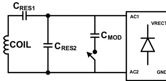
Figure 34. Capacitive Modulation
