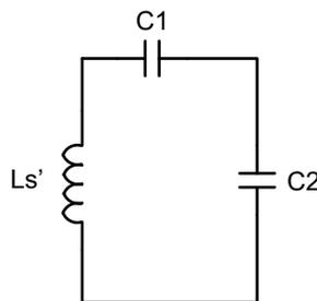
**Figure 45. Dual Resonant Circuit with the Receiver Coil**
