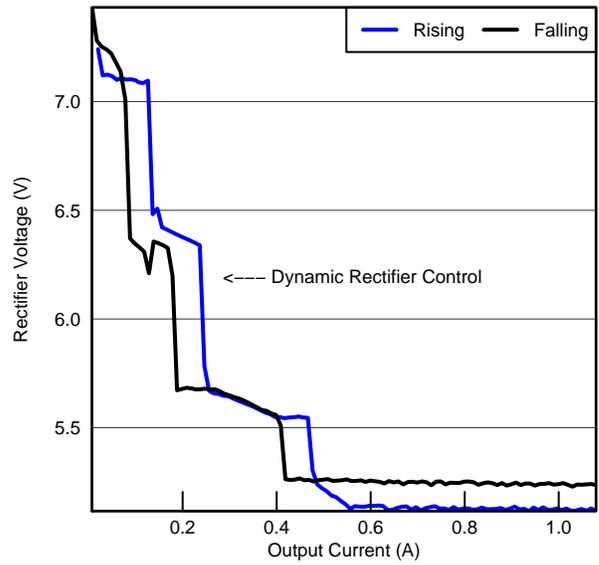
Figure 7.  $V_{RECT}$  vs.  $I_{LOAD}$  at  $R_{ILIM} = 220\Omega$
