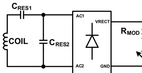
**Figure 33. Resistive Modulation**
