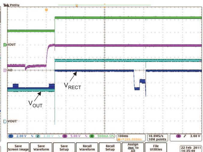
Figure 19. Adapter Insertion ( $V_{AD} = 10\text{V}$ )
