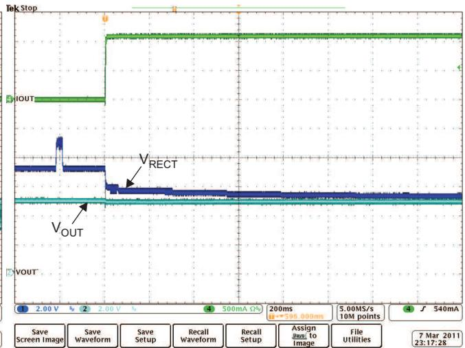
Figure 15. 1A Load Step Full System Response
