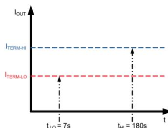
**Figure 32. Termination Deglitch Timings for the CS100 Packet**
