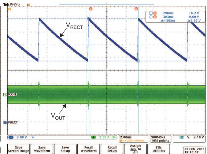
Figure 17. Rectifier Overvoltage Clamp ( $f_{op} = 110\text{kHz}$ )
