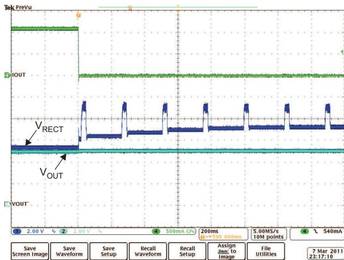
Figure 16. 1A Load Dump Full System Response
