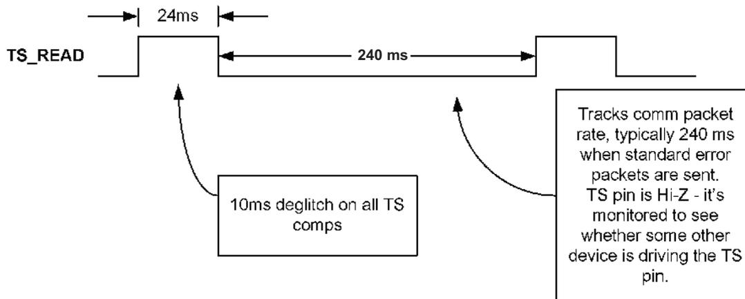
**Figure 43. Timing Diagram for TS Detection Circuit**
