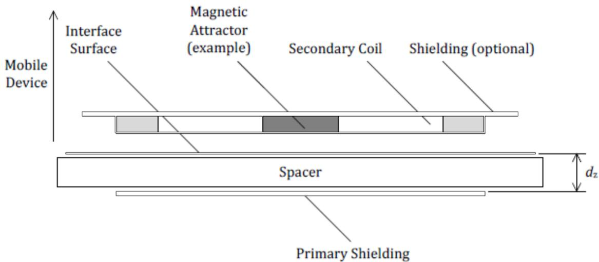
**Figure 46. WPC v1.0 Receiver Coil Test Fixture for the Inductance Measurement  $L_s'$  (copied from System Description Wireless Power Transfer, volume 1: Low Power, Part 1 Interface Definition, Version 1.0.1, Figure 4-4)**
