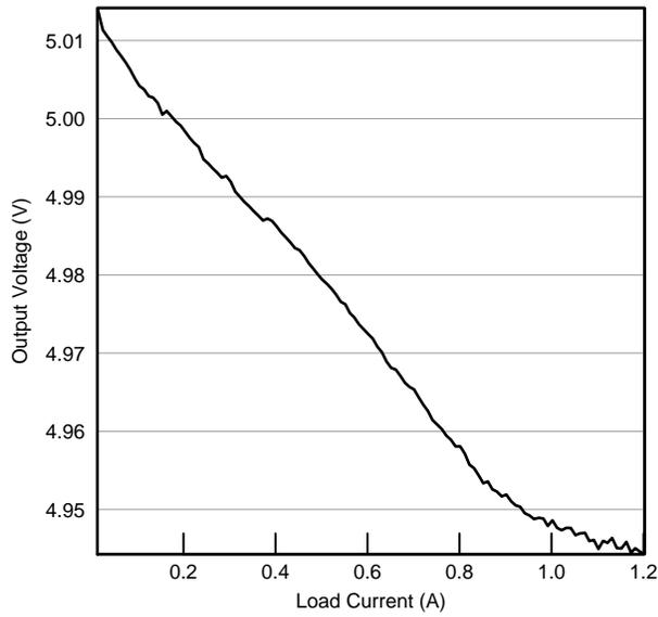
Figure 10. I<sub>LOAD</sub> Sweep (I-V Curve)
