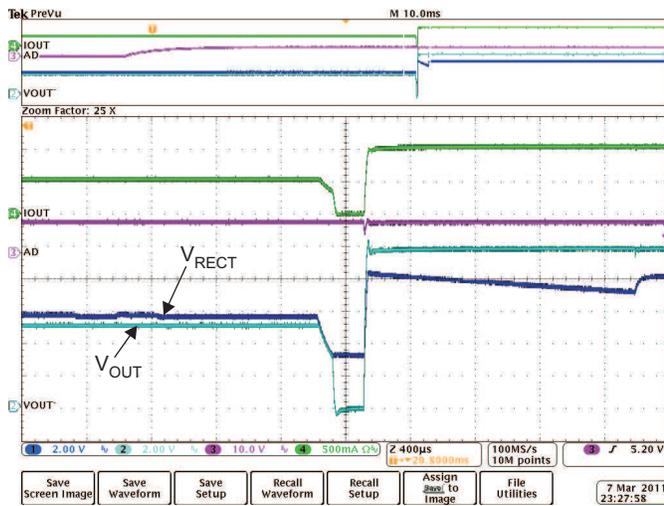
Figure 20. Adapter Insertion ( $V_{AD} = 10V$ ) Illustrating Break-Before-Make Operation
