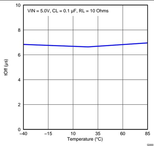
Figure 43. Turn-Off Time vs Temperature
