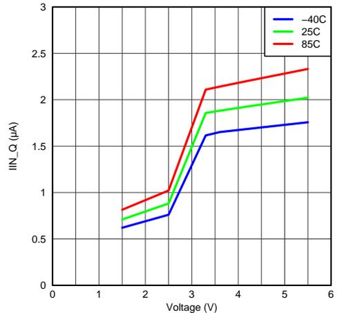
Figure 4. Input Current, Quiescent vs Input Voltage
