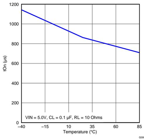
Figure 24. Turn-on Time vs Temperature
