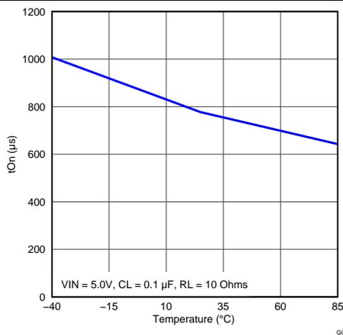
Figure 42. Turn-on Time vs Temperature
