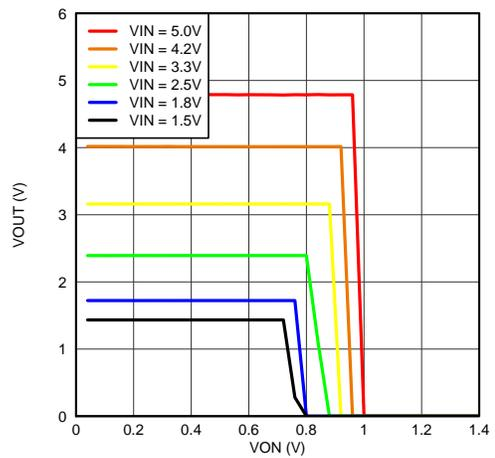
Figure 2. TPS22910A On Input Threshold (Active Low)
