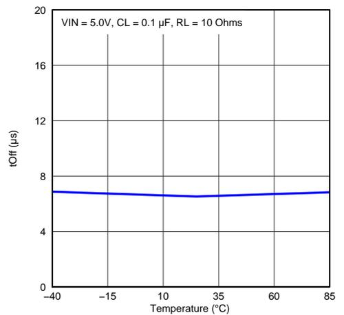
**Figure 34. Turn-off Time vs Temperature**
