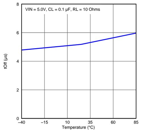
Figure 16. Turn-off Time vs Temperature
