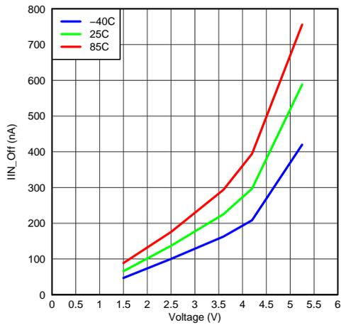
Figure 7. Input Current, Off vs Input Voltage
