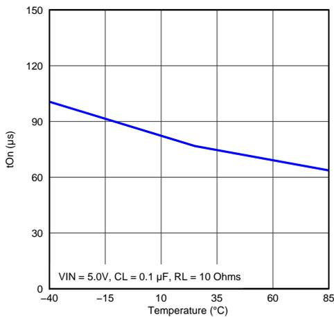
**Figure 33. Turn-on Time vs Temperature**
