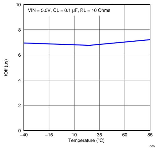
Figure 25. Turn-off Time vs Temperature
