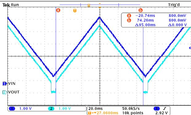
Figure 9. Under Voltage Lockout Response (IOUT = -100mA)
