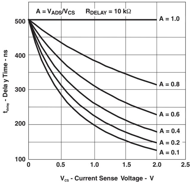
Figure 5. Delay Time Under Varying ADS Voltages
