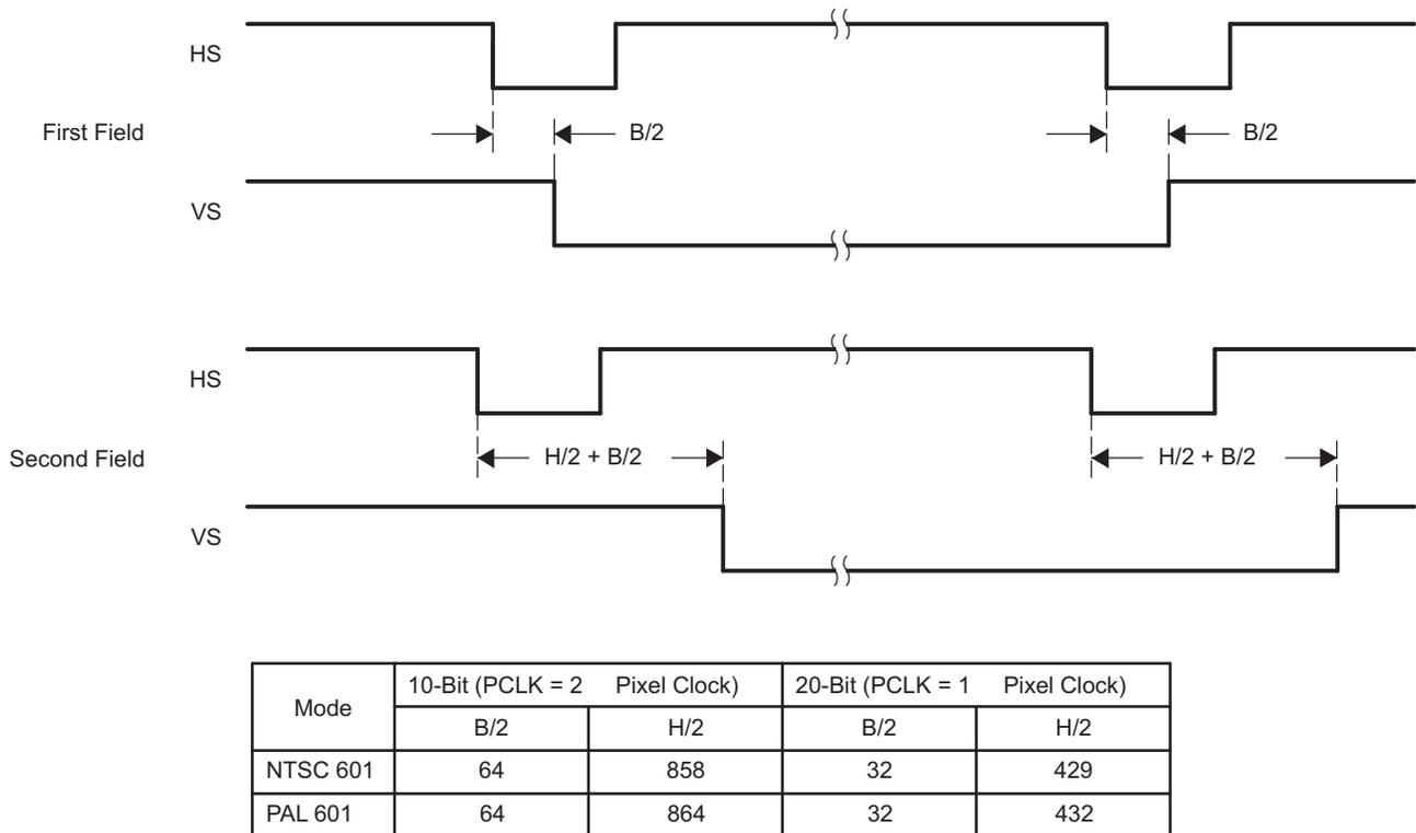
Figure 2-18. VSYNC Position With Respect to HSYNC
