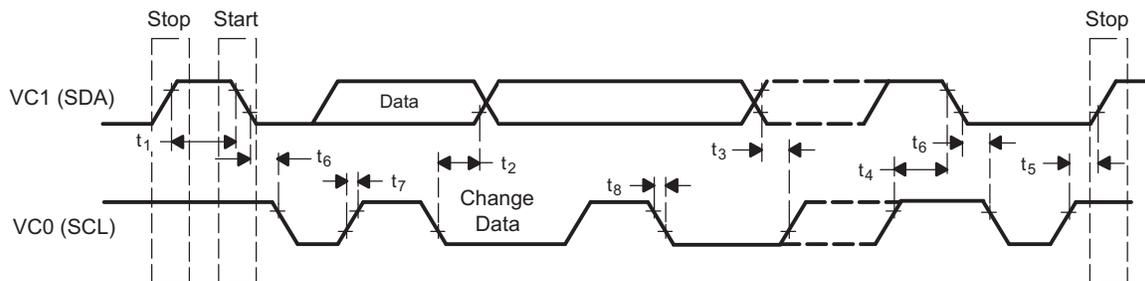
Figure 3-2. I<sup>2</sup>C Host Port Timing
