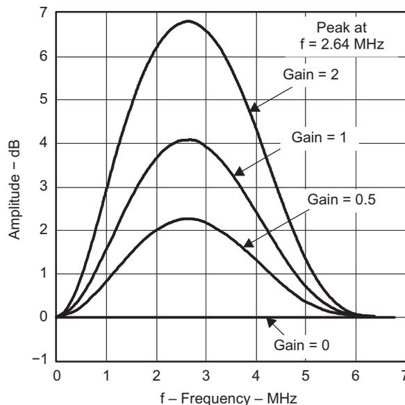
Figure 2-9. Peaking Filter Response, NTSC/PAL ITU-R BT.601 Sampling
