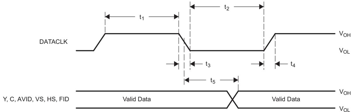
Figure 3-1. Clocks, Video Data, and Sync Timing
