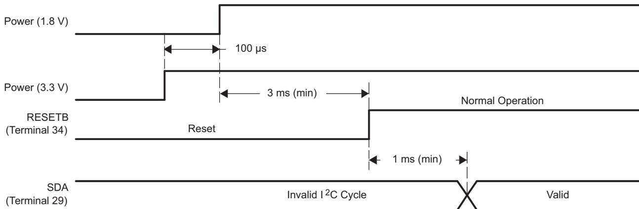
NOTE: All times shown are minimum values. Maximum time between 1.8 V and 3.3 V should be no longer than 1 second.
