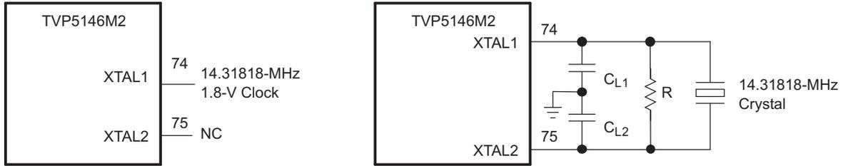
NOTE: The resistor (R) in parallel with the crystal is recommended to support a wide range of crystal types. A 100-kΩ resistor may be used for most crystal types.
