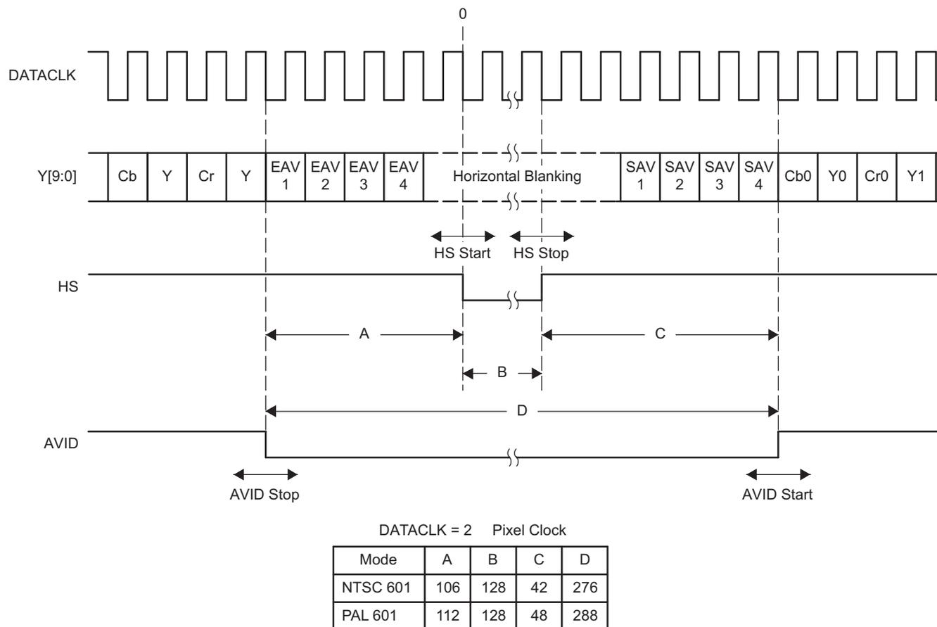
NOTE: ITU-R BT.656 10-bit 4:2:2 timing with 2x pixel clock reference
