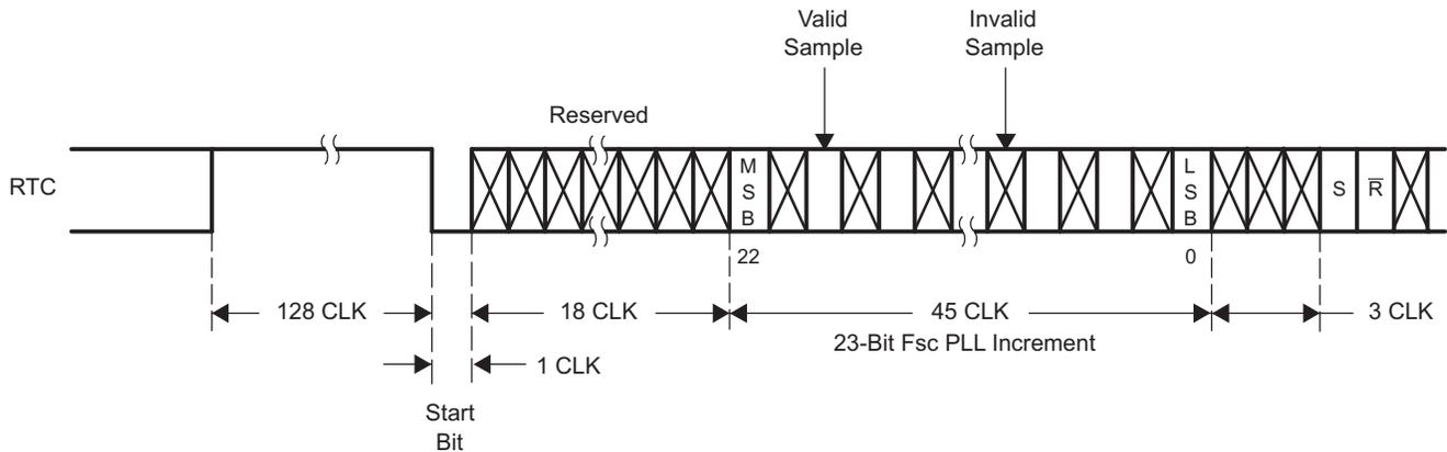
NOTE: RTC reset bit ( $\bar{R}$ ) is active-low, Sequence bit (S) PAL: 1 = (R-Y) line normal, 0 = (R-Y) line inverted, NTSC: 1 = no change
