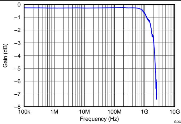
**Figure 3. Gain vs Frequency for MHL/USB Switch**
