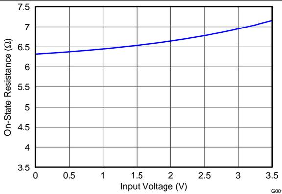
**Figure 1. ON Resistance vs  $V_I$  for MHL/USB Switch**
