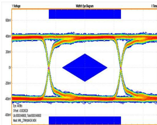
Figure 16. MHL Eye Pattern: 480p 60 fps (No Switch)
