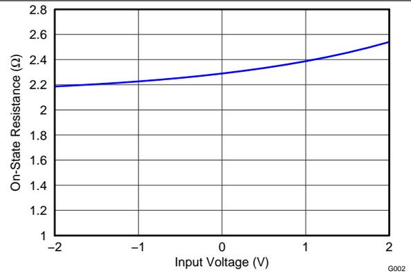
**Figure 2. ON Resistance vs  $V_I$  for USB/Audio Switch**
