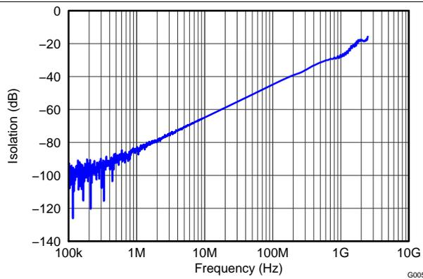
**Figure 5. Off Isolation vs Frequency for MHL/USB Switch**
