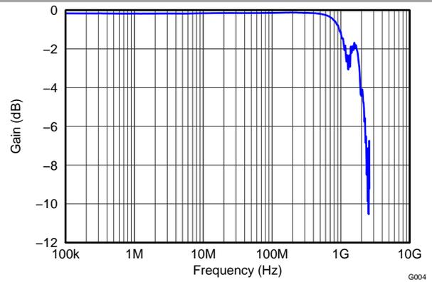
**Figure 4. Gain vs Frequency for USB/Audio Switch**
