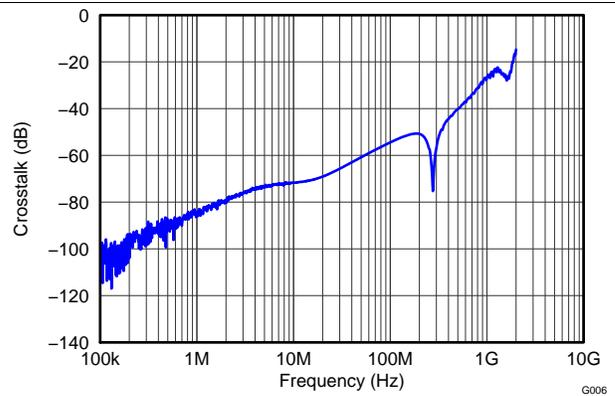
**Figure 6. Cross Talk vs Frequency for MHL/USB Switch**
