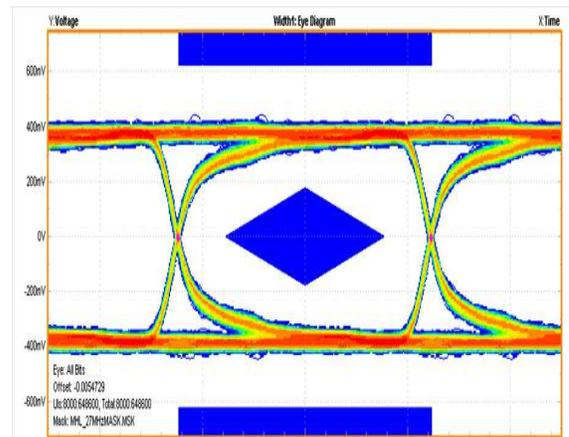
Figure 17. MHL Eye Pattern: 480p 60 fps (With Switch)
