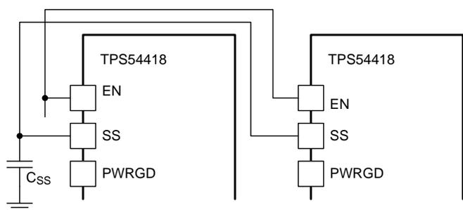
Figure 27. Ratiometric Start-Up Schematic
