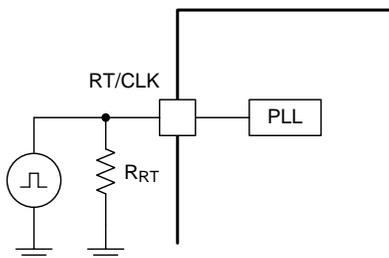
**Figure 29. Synchronizing to a System Clock**
