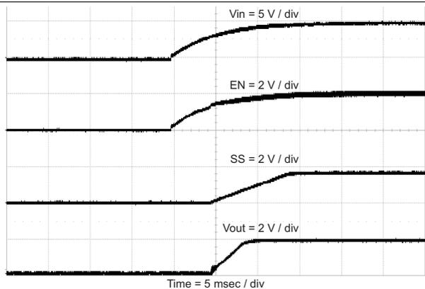
Figure 42. Power Up  $V_{OUT}$ ,  $V_{IN}$
