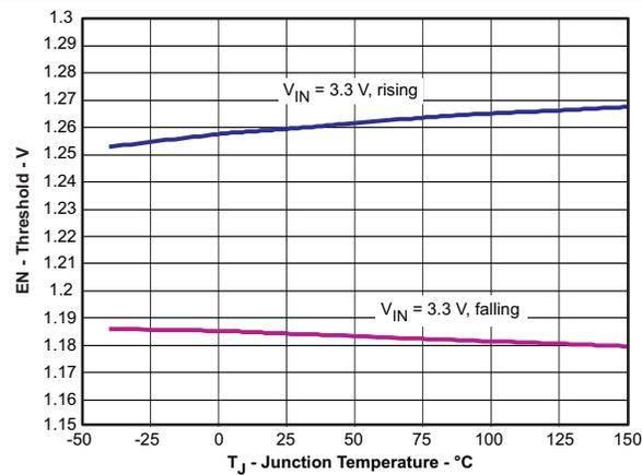
Figure 10. Enable Pin Voltage vs Junction Temperature
