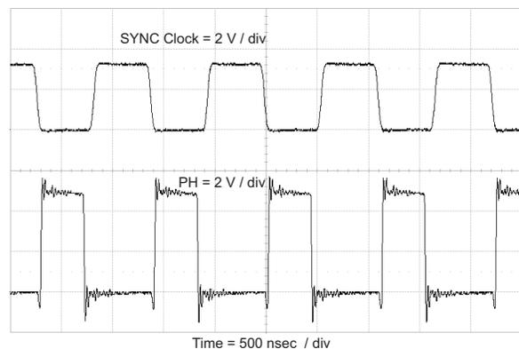
**Figure 30. Plot of Synchronizing to System Clock**
