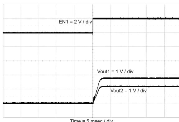
Figure 28. Ratiometric Start-Up Using Coupled SS Pins
