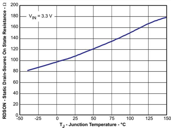
Figure 21. PWRGD On Resistance vs Junction Temperature
