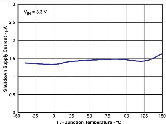
Figure 16. Shutdown Supply Current vs Junction Temperature
