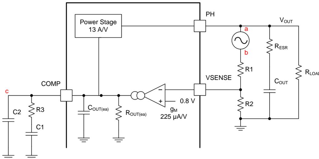
Figure 31. Small Signal Model for Loop Response
