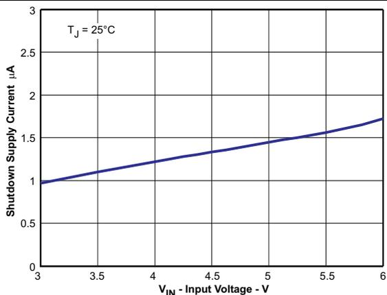
Figure 17. Shutdown Supply Current vs Input Voltage
