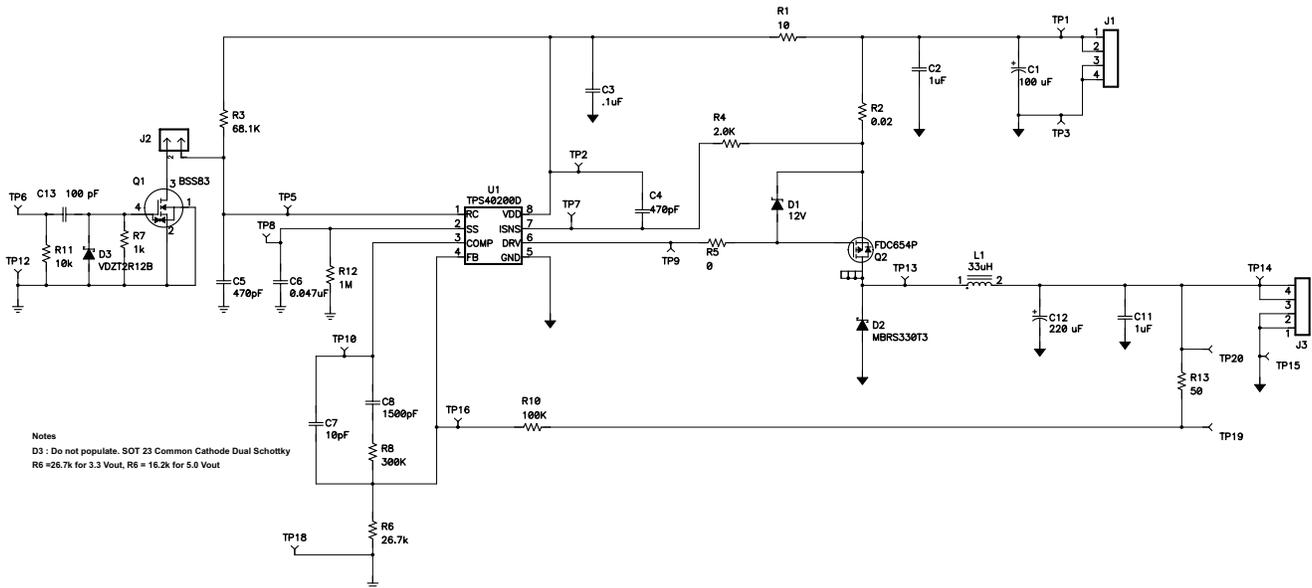
Figure 32. 8-V to 16-V  $V_{IN}$  Step-Down Buck Converter
