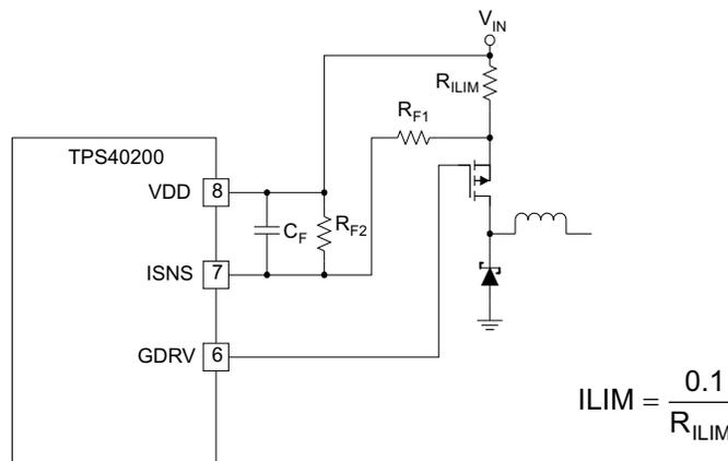
Figure 35. Overcurrent Trip Circuit for  $R_{F2}$  Open
