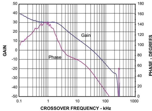
**Figure 40. Overall System Gain and Phase Response**
