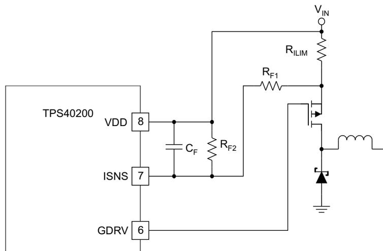
NOTE: The current-limit resistor and its associated circuitry can be eliminated and pins 7 and 8 shorted. However, the result of this may result in damage to the part or PC board in the event of an overcurrent event.
