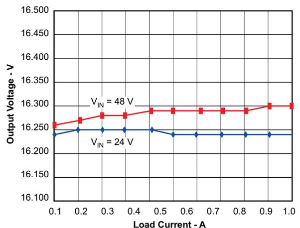
Figure 46. Load Regulation, Two Input Voltage Extremes
