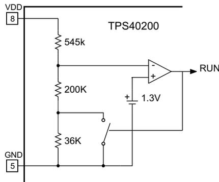
**Figure 29. Undervoltage Lockout**
