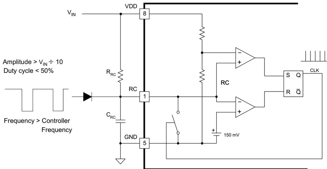
Figure 25. Diode-Connected Synchronization
