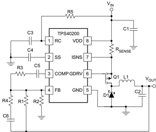
Figure 1. 12-V to 5-V Buck Converter With 94% Efficiency
