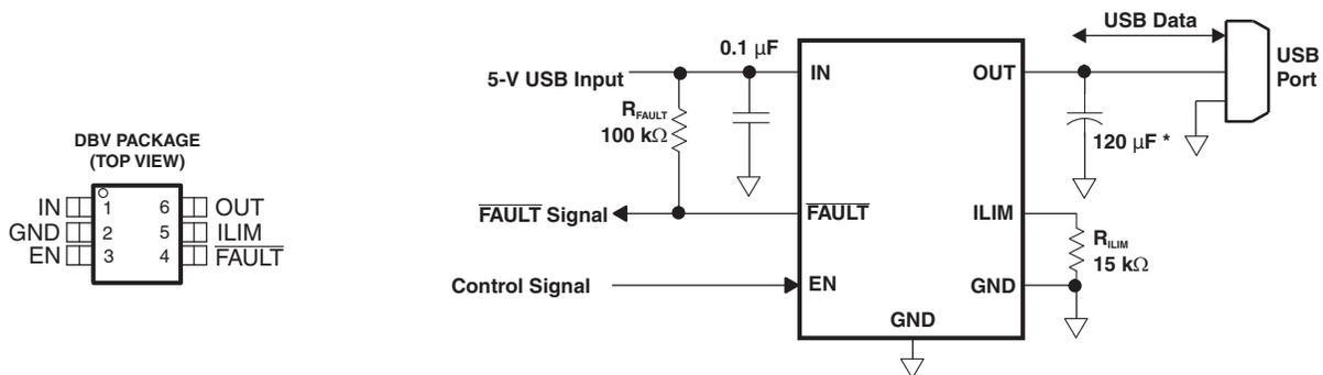
\* USB requirement that downstream-facing ports are bypassed with at least 120  $\mu$ F per hub
