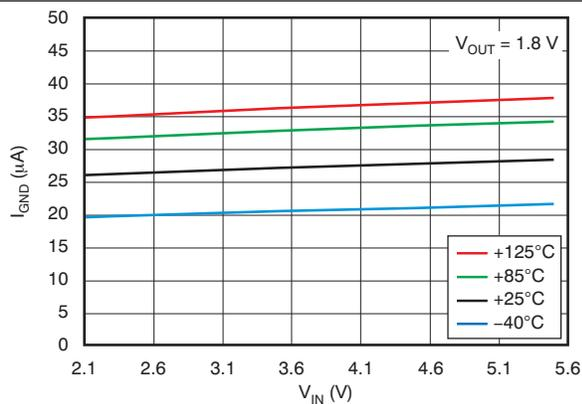
Figure 5. Ground Pin Current vs Input Voltage
