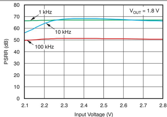
Figure 11. Power-Supply Ripple Rejection vs Input Voltage
