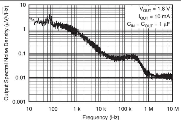
Figure 12. Output Spectral Noise Density vs Frequency
