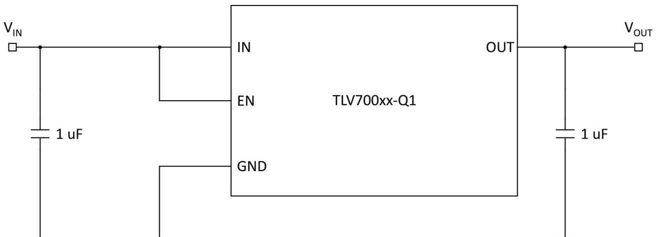
Figure 21. Simplified Schematic
