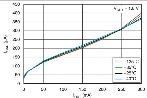
Figure 6. Ground Pin Current vs Load
