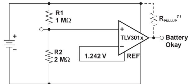
When the battery voltage drops below 1.9 V, the Battery Okay output goes low.
