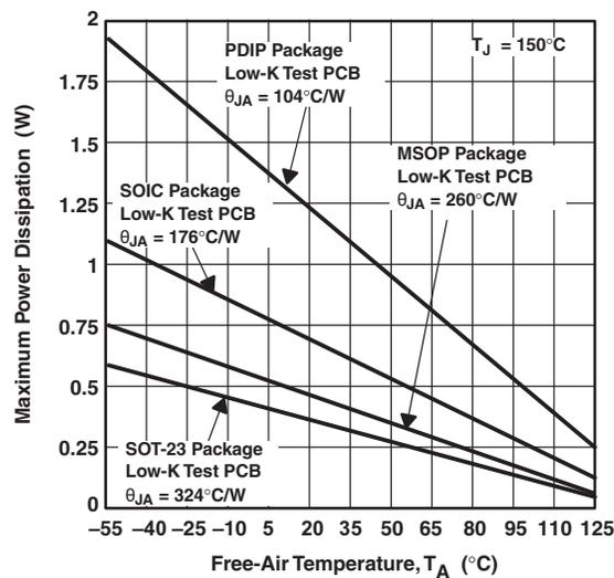
Figure 53. Maximum Power Dissipation vs Free-Air Temperature
