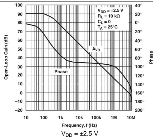
Figure 12. Open-Loop Gain and Phase vs Frequency
