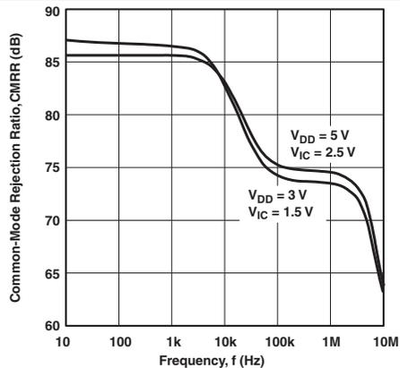
Figure 17. Common-Mode Rejection Ratio vs Frequency
