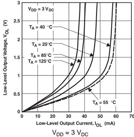
Figure 7. Low-Level Output Voltage vs Low-Level Output Current
