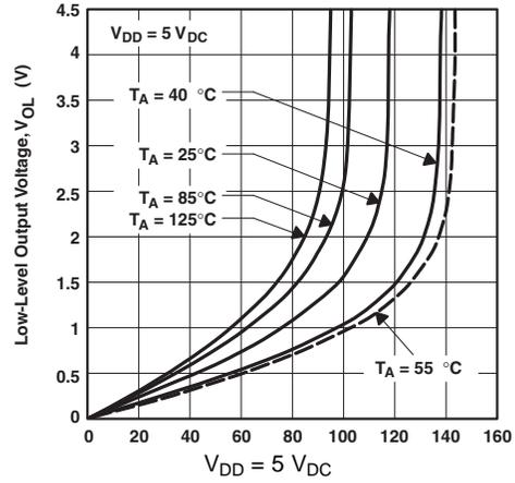
Figure 8. Low-level Output Voltage vs Low-Level Output Current
