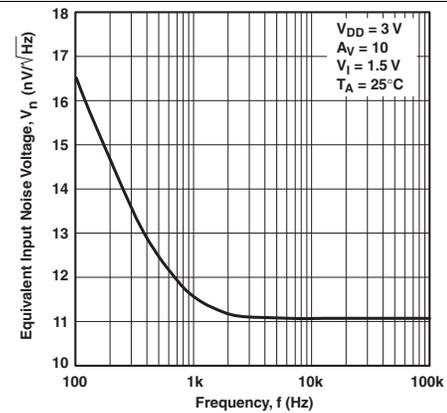
Figure 28. Equivalent Input Noise Voltage vs Frequency
