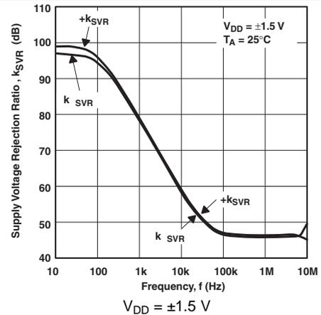
Figure 18. Supply-Voltage Rejection Ratio vs Frequency
