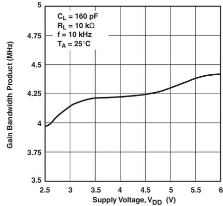
Figure 38. Gain Bandwidth Product vs Supply Voltage
