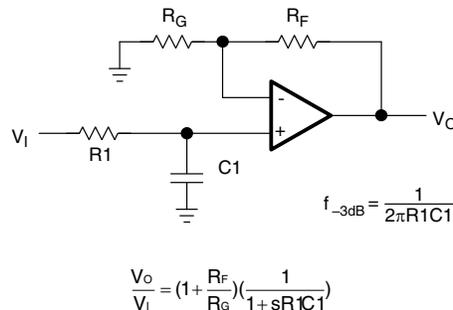
Figure 51. Single-Pole Low-Pass Filter
