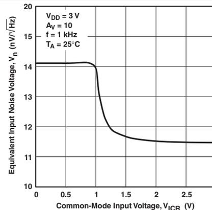
Figure 30. Equivalent Input Noise Voltage vs Common-Mode Input Voltage
