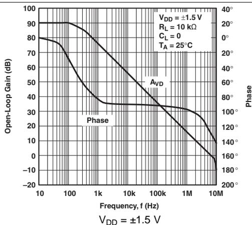
Figure 11. Open-Loop Gain and Phase vs Frequency
