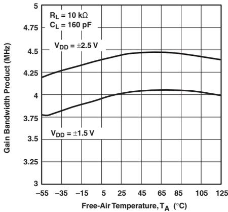
Figure 39. Gain Bandwidth Product vs Free-Air Temperature
