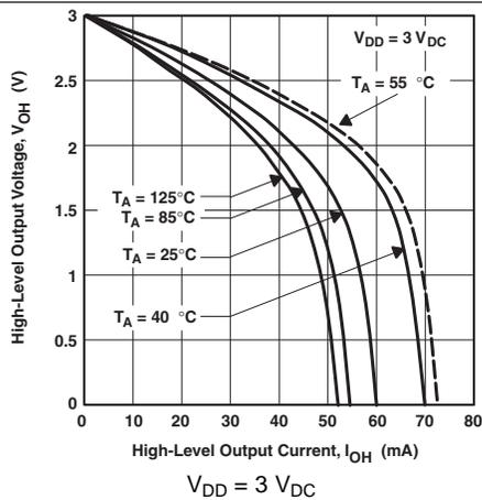
Figure 5. High-Level Output Voltage vs High-Level Output Current
