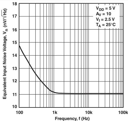
Figure 29. Equivalent Input Noise Voltage vs Frequency
