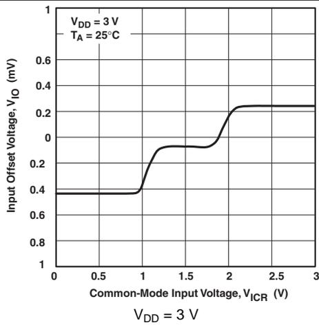
Figure 1. Input Offset Voltage vs Common-Mode Input Voltage
