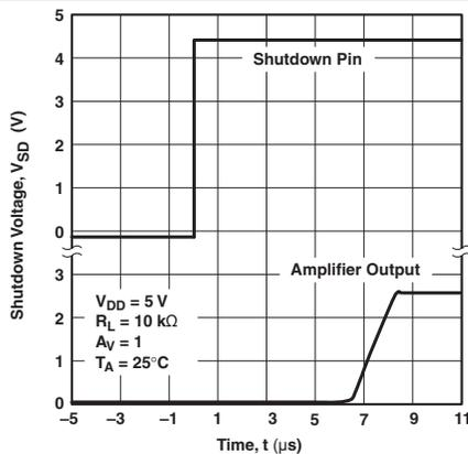
Figure 23. Amplifier With a Shutdown Pulse Turnoff Characteristics
