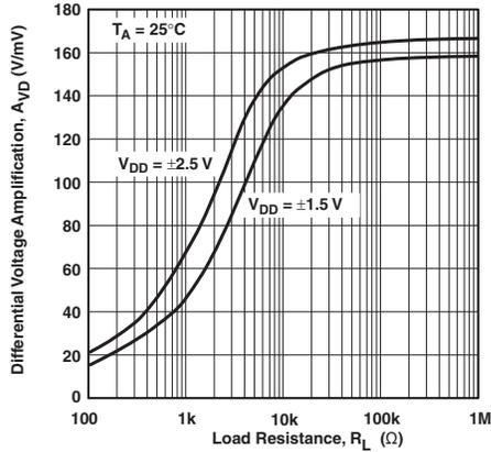
Figure 13. Differential Voltage Amplification vs Load Resistance
