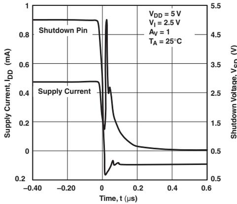
Figure 25. Turnoff Supply Current With a Shutdown Pulse
