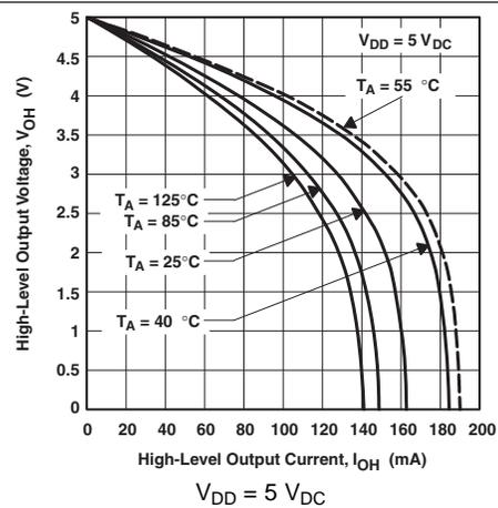
Figure 6. High-Level Output Voltage vs High-Level Output Current
