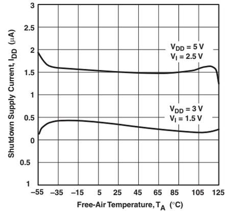
Figure 26. Shutdown Supply Current vs Free-Air Temperature
