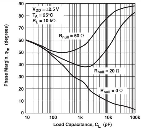
Figure 36. Phase Margin vs Load Capacitance
