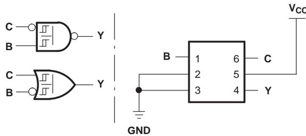
Figure 6. 2-Input NAND Gate With One Inverted Input
