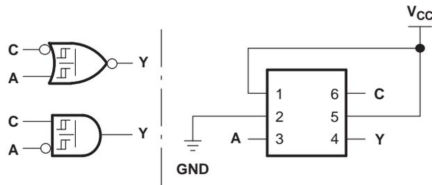
Figure 5. 2-Input NOR Gate With One Inverted Input
