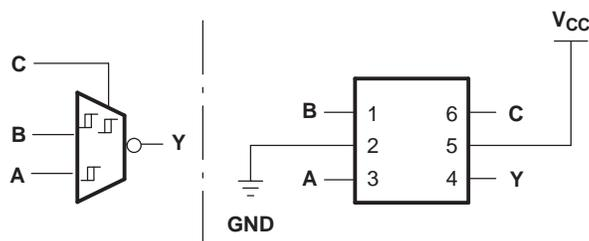
**Figure 3. 2-to-1 Data Selector With Inverted Output**
