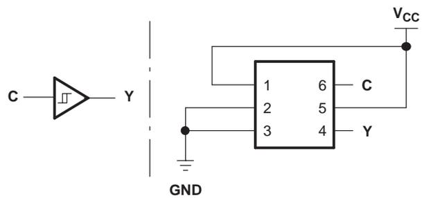
Figure 8. Noninverted Buffer
