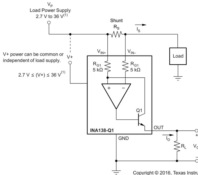
(1) Maximum V<sub>p</sub> and V<sub>+</sub> voltage is 60 V with INA168-Q1.
