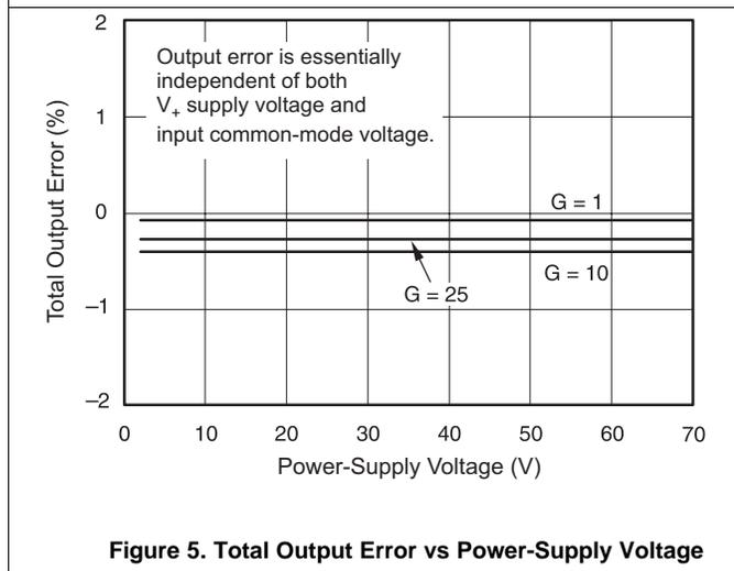
**Figure 5. Total Output Error vs Power-Supply Voltage**
