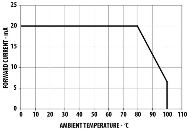
Figure 3. Ambient Temperature vs. Maximum DC Forward Current.
