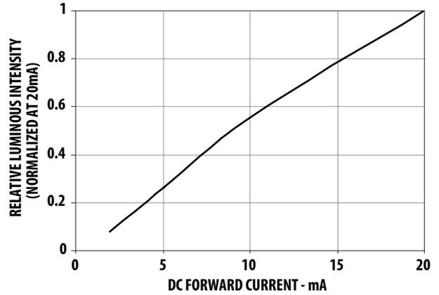
Figure 2. Relative Luminous Intensity vs. Forward Current.
