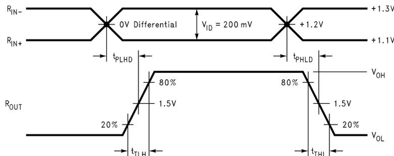
Figure 2. Receiver Propagation Delay and Transition Time Waveforms
