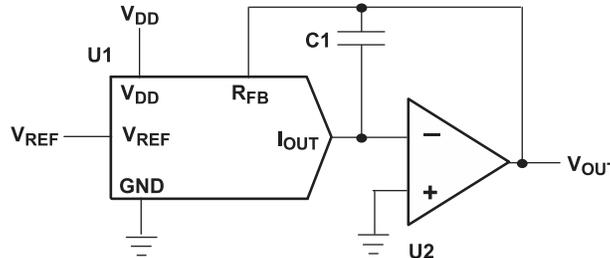
Figure 20. Gain Peaking Prevention Circuit With Compensation Capacitor
