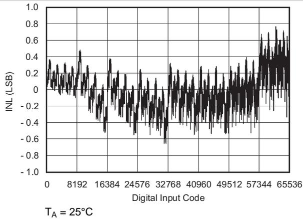
Figure 2. Linearity Error vs Digital Input Code
