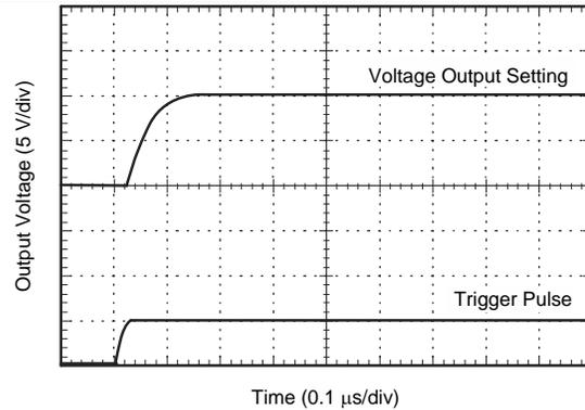
Figure 11. DAC Settling Time
