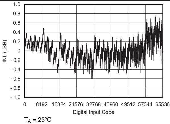
Figure 12. Linearity Error vs Digital Input Code
