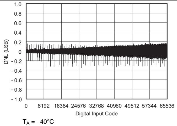
**Figure 5. Differential Linearity Error vs Digital Input Code**
