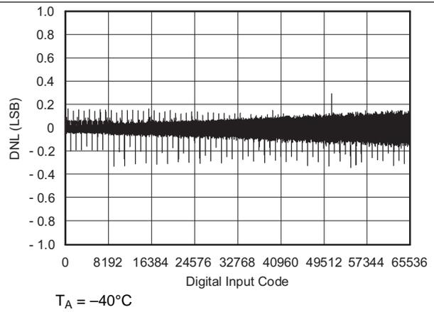
Figure 15. Differential Linearity Error vs Digital Input Code
