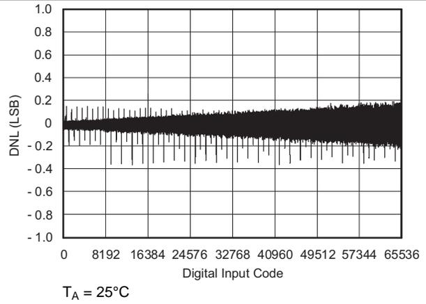
**Figure 3. Differential Linearity Error vs Digital Input Code**
