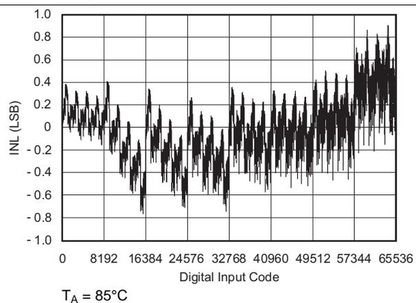
**Figure 6. Linearity Error vs Digital Input Code**
