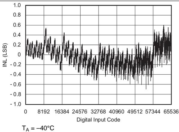
Figure 14. Linearity Error vs Digital Input Code
