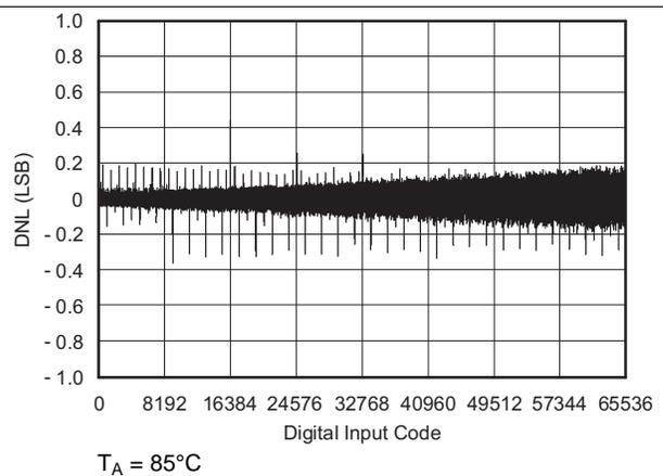
Figure 17. Differential Linearity Error vs Digital Input Code
