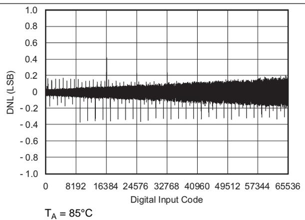
**Figure 7. Differential Linearity Error vs Digital Input Code**
