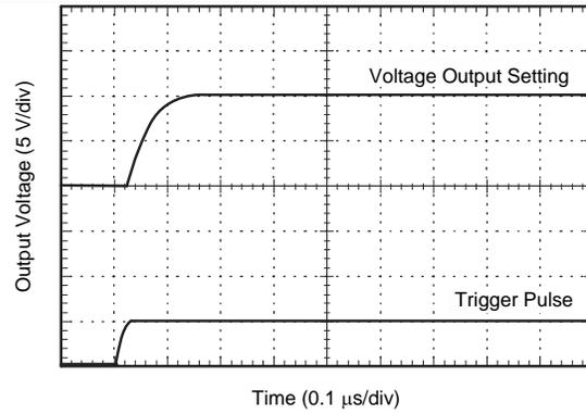
Figure 11. DAC Settling Time
