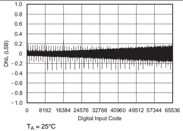
Figure 13. Differential Linearity Error vs Digital Input Code
