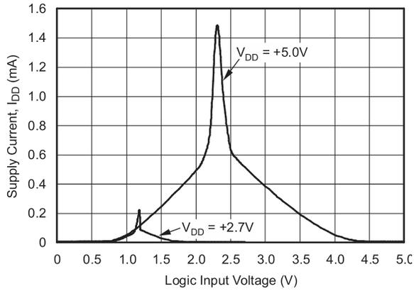
Figure 8. Supply Current vs Logic Input Voltage
