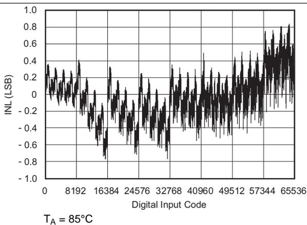
Figure 16. Linearity Error vs Digital Input Code
