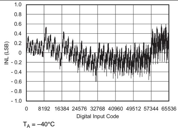
**Figure 4. Linearity Error vs Digital Input Code**
