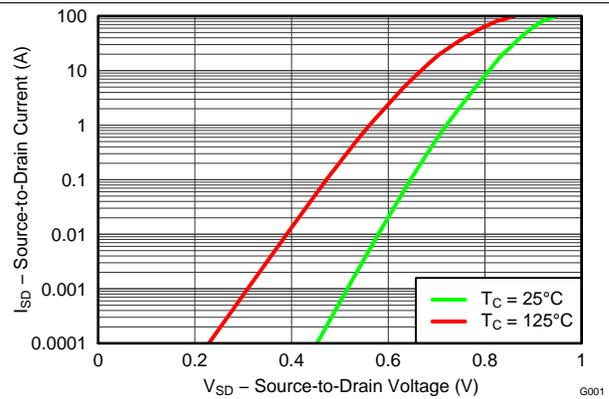
Figure 24. Sync MOSFET Body Diode
