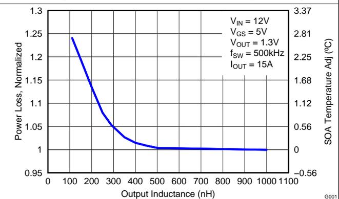
Figure 8. Normalized Power Loss vs Output Inductance
