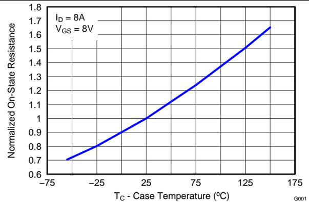
Figure 22. Sync MOSFET Normalized R<sub>DS(on)</sub>
