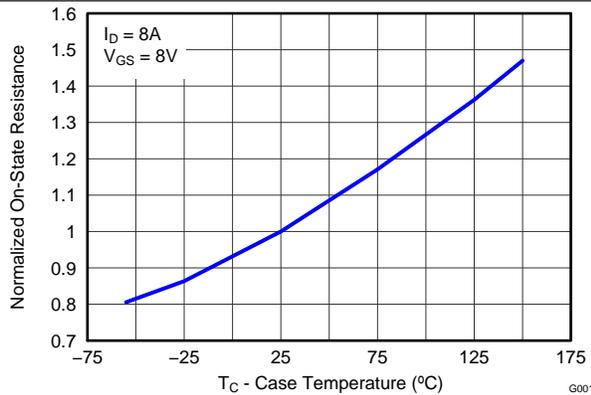
Figure 21. Control MOSFET Normalized R<sub>DS(on)</sub>
