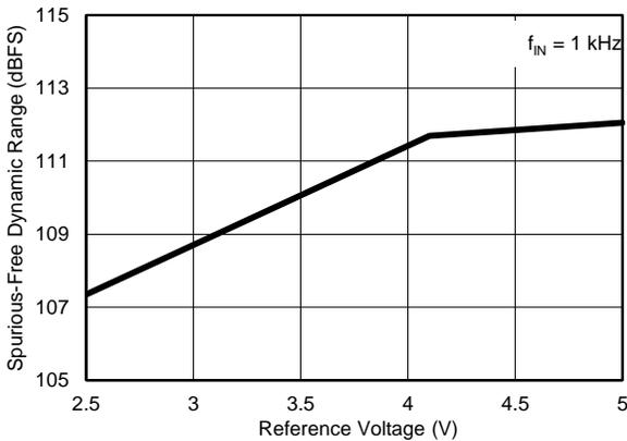
**Figure 22. SFDR vs REFERENCE VOLTAGE**
