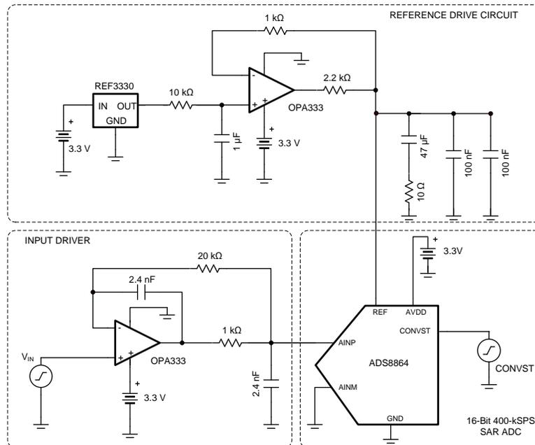
Figure 70. Ultralow-Power DAQ Circuit at 10 kSPS
