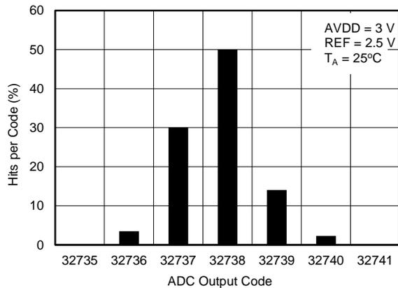
**Figure 14. DC INPUT HISTOGRAM ( $V_{REF} = 2.5\text{ V}$ )**
