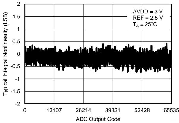
Figure 6. TYPICAL INL ( $V_{REF} = 2.5\text{ V}$ )
