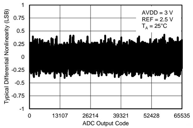
Figure 7. TYPICAL DNL ( $V_{REF} = 2.5\text{ V}$ )
