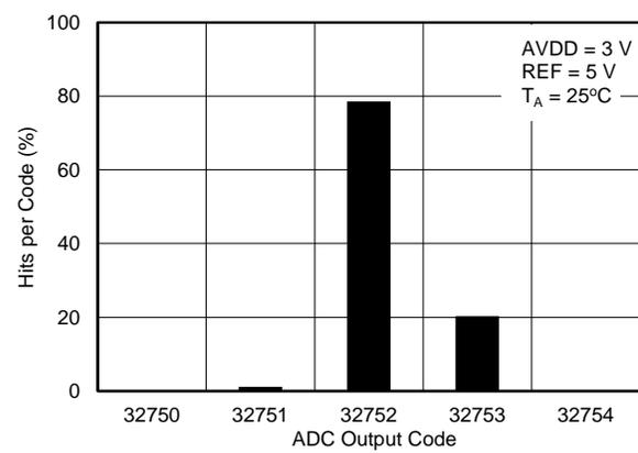
**Figure 15. DC INPUT HISTOGRAM ( $V_{REF} = 5\text{ V}$ )**
