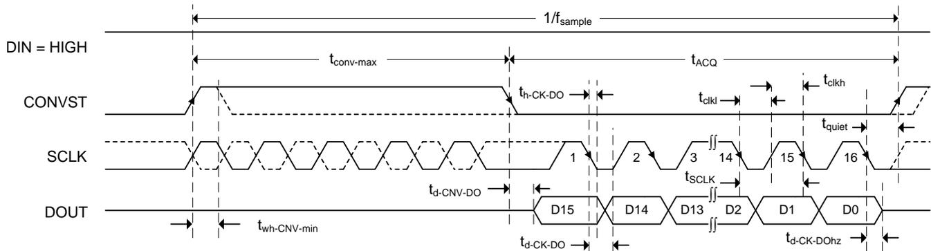
Figure 1. 3-Wire Operation: CONVST Functions as Chip Select
