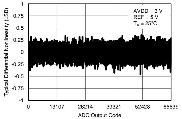
Figure 9. TYPICAL DNL ( $V_{REF} = 5\text{ V}$ )
