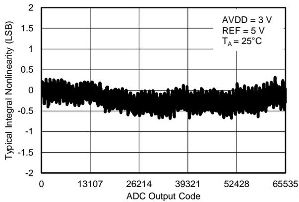
Figure 8. TYPICAL INL ( $V_{REF} = 5\text{ V}$ )
