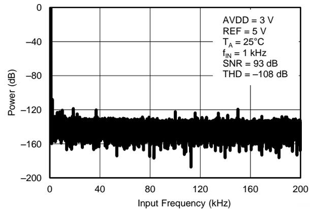
**Figure 17. TYPICAL FFT ( $V_{REF} = 5\text{ V}$ )**
