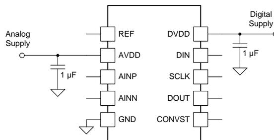
Figure 62. Supply Decoupling
