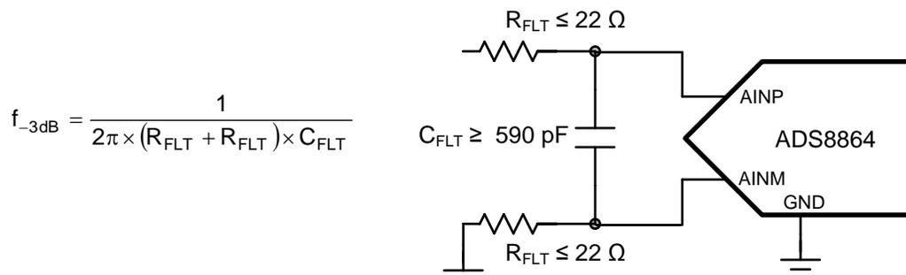
**Figure 67. Antialiasing Filter**
