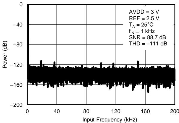
**Figure 16. TYPICAL FFT ( $V_{REF} = 2.5\text{ V}$ )**
