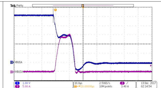
**图 9-6. VBUS Short with Schottky Diode**
