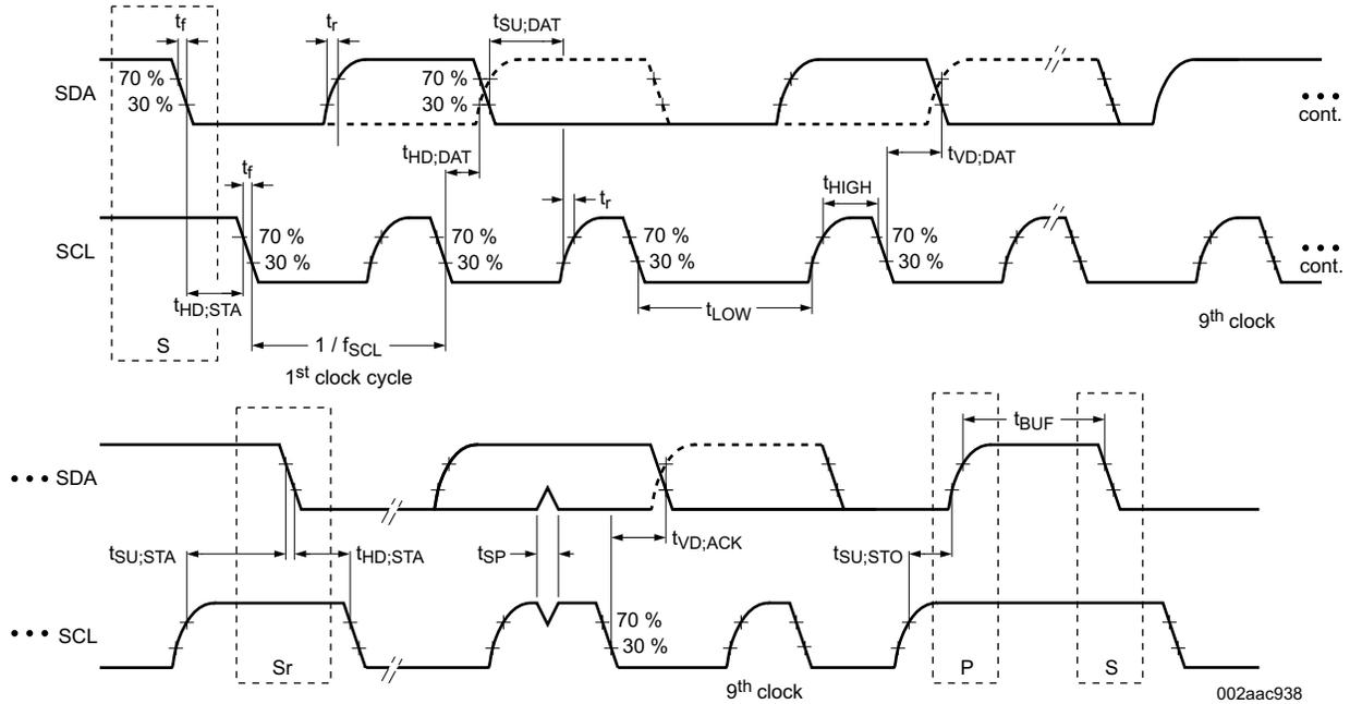
图 7-1. I<sup>2</sup>C Slave Interface Timing
