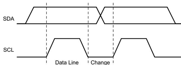
图 8-24. I<sup>2</sup>C Bit Transfer
