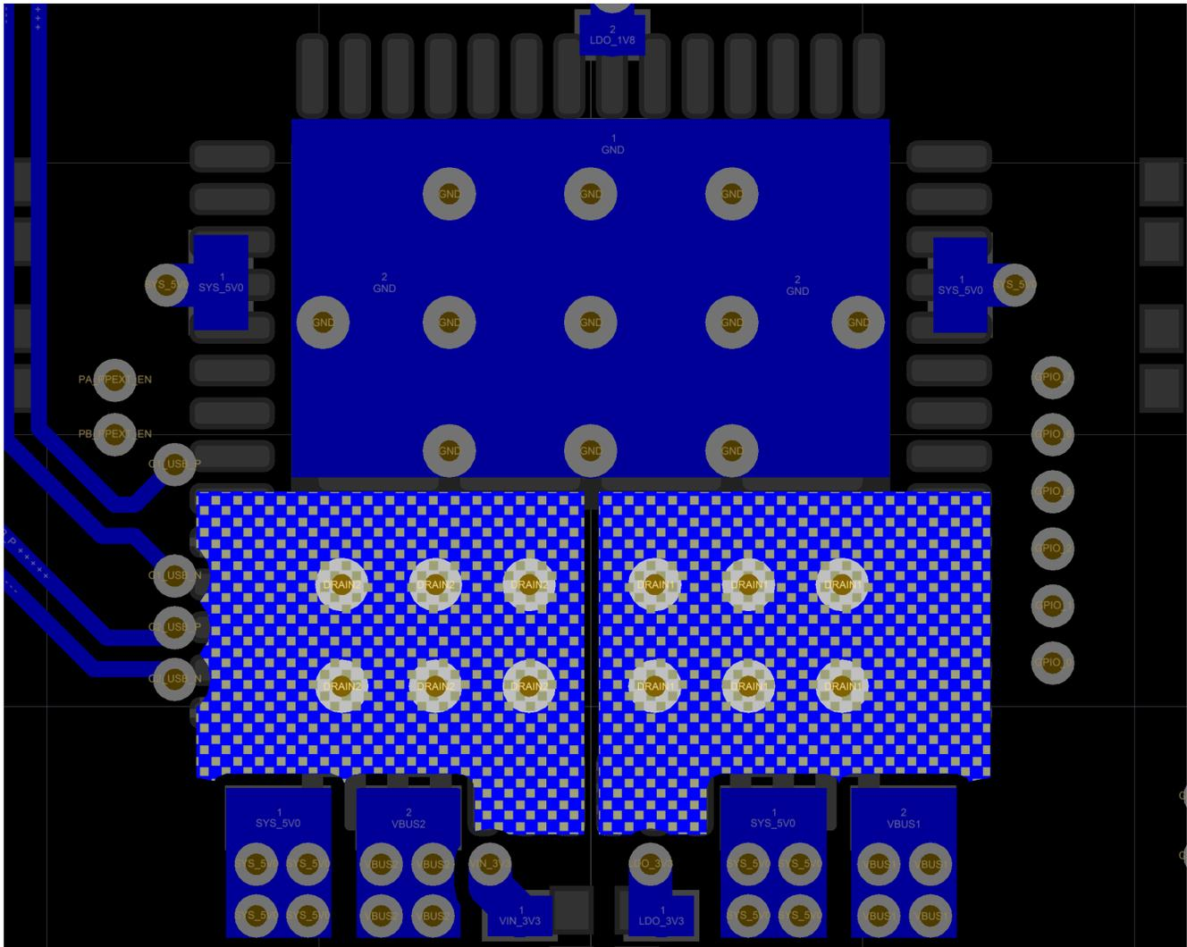
图 11-16. Figure 13. DRAIN1 and DRAIN2 Bottom Layer
