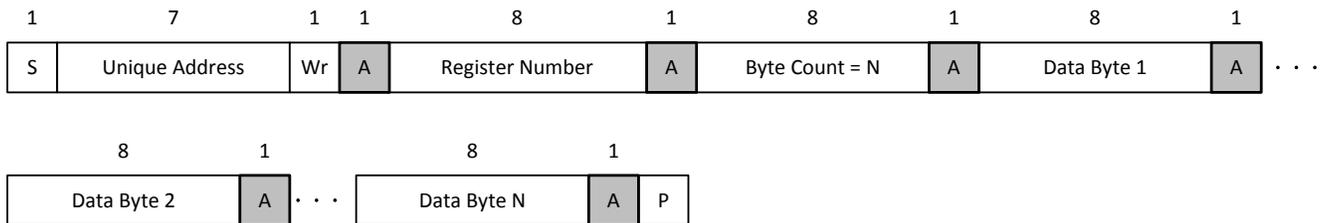
图 8-26. I<sup>2</sup>C Unique Address Write Register Protocol
