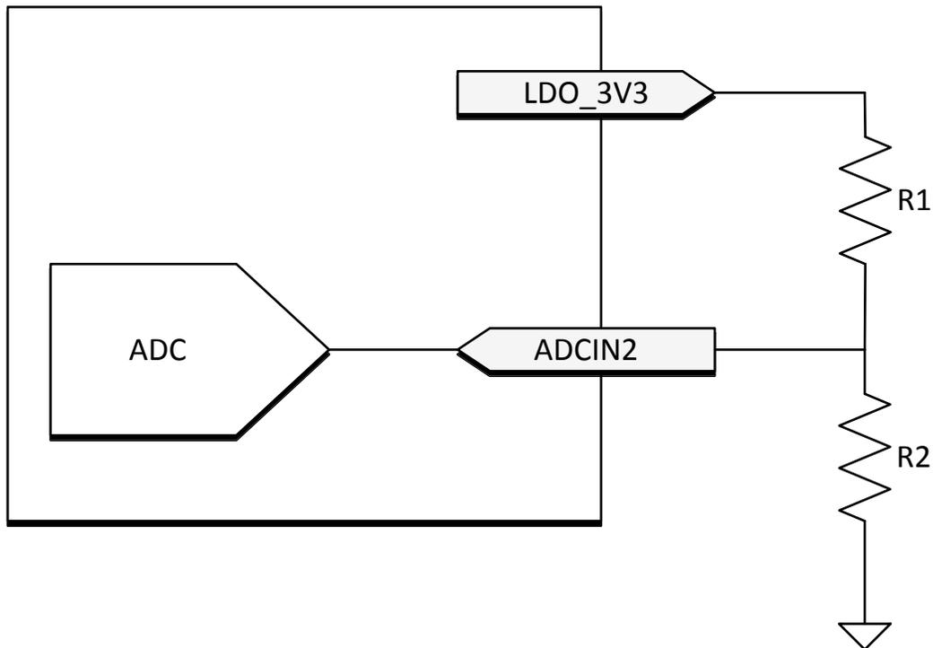
**图 8-29. I<sup>2</sup>C Address Divider**
