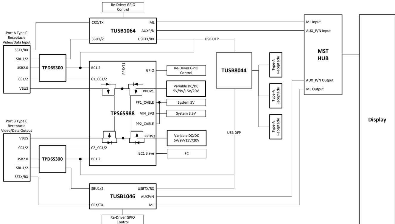
图 9-11. USB and DisplayPort Dock Block Diagram
