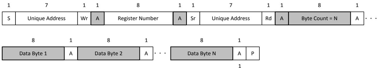
图 8-27. I<sup>2</sup>C Unique Address Read Register Protocol
