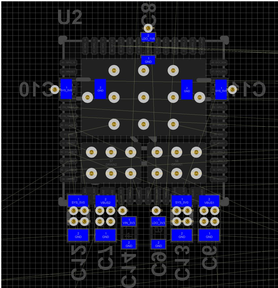
图 11-11. System Capacitors Placement Bottom Layer
