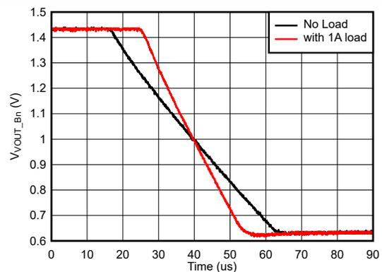
$V_{PVIN\_Bn} = 3.3\text{ V}$  Buck VSET = 1.4 V to 0.6 V Slew Rate = 33.3 V/ms
