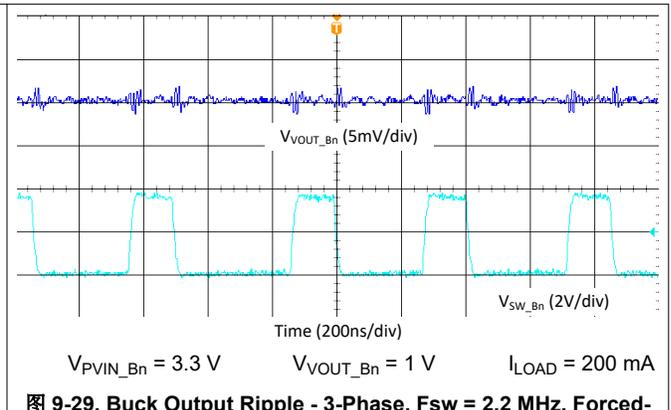
图 9-29. Buck Output Ripple - 3-Phase, Fsw = 2.2 MHz, Forced-PWM Mode
