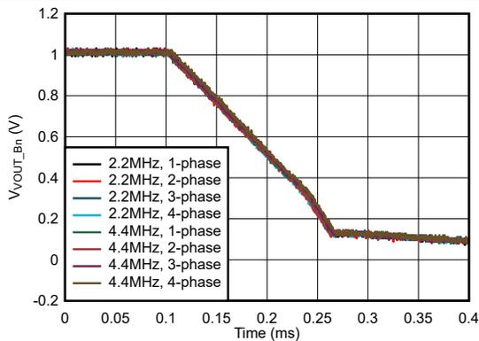
$V_{PVIN\_Bn} = 3.3\text{ V}$  Buck VSET = 1 V Slew Rate = 5 V/ms
