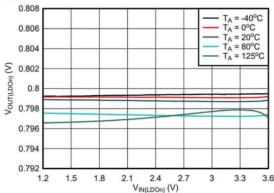
$V_{OUT(LDO_n)} = 0.8\text{ V}$   $I_{OUT(LDO_n)} = 500\text{ mA}$
