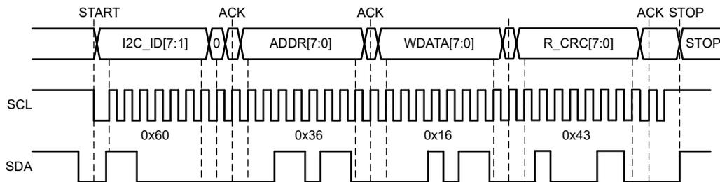
The I<sup>2</sup>C controller device (the MCU) provides R\_CRC[7:0], which is calculated from the I2C\_ID, R/W, ADDR, and the WDATA bits (24 bits). See CRC Calculation for I2C and SPI Interface Protocols.
