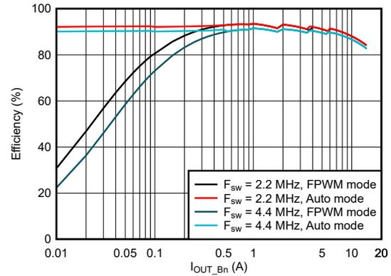
$V_{PVIN\_Bn} = 3.3\text{ V}$   $V_{VOUT\_Bn} = 1.8\text{ V}$  4-Phase
