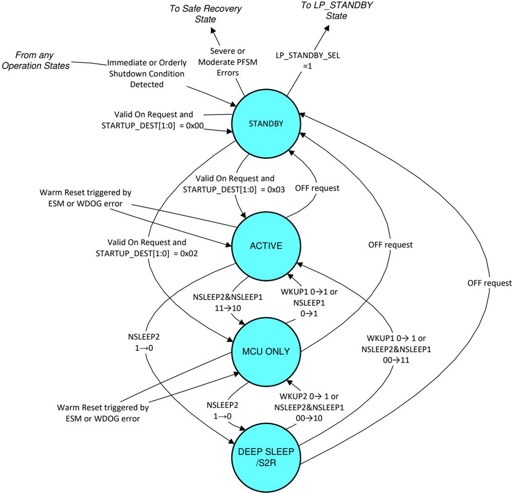
) defines the ON or OFF state and the sequencing timing of the external regulators and GPIO outputs. This example defines four power states: STANDBY, ACTIVE, MCU ONLY, and DEEP\_SLEEP/S2R three power states: STANDBY, ACTIVE and RETENTION states. The priority order of these states is as follows:
