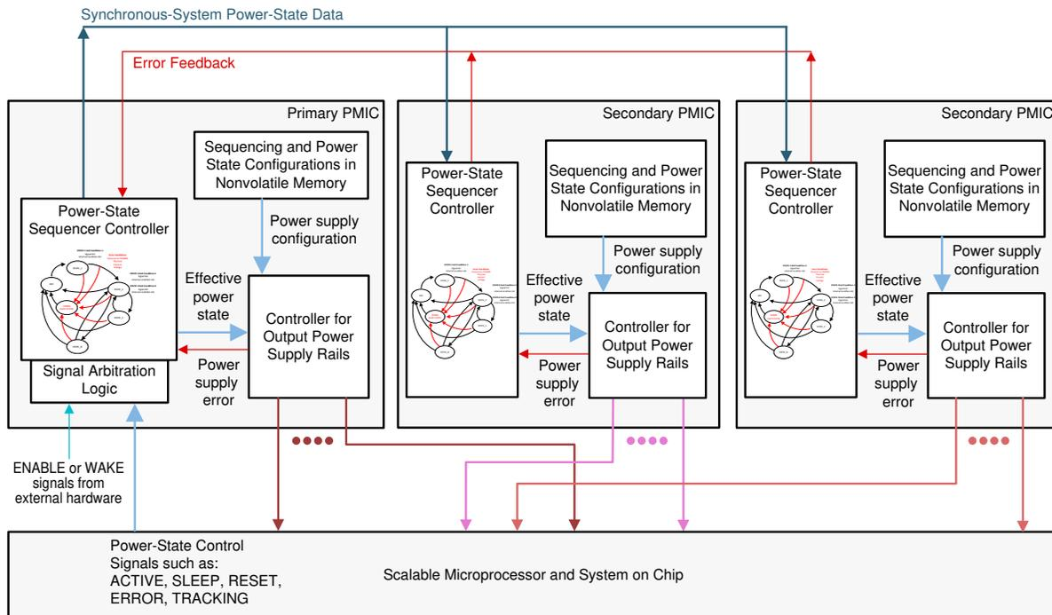
图 8-43. Multi-PMIC Power State Synchronization Block Diagram
