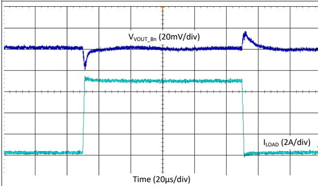
图 9-38. Buck Load Step Transient - 4-Phase, 2.2 MHz, Auto Mode
