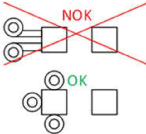
**图 9-69. Ground connection of capacitor at VOUT\_LDOVINT pin**
