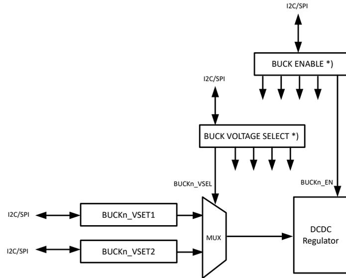
\*) BUCK ENABLE and BUCK VOLTAGE SELECT bits are located in BUCKx\_CTRL register
