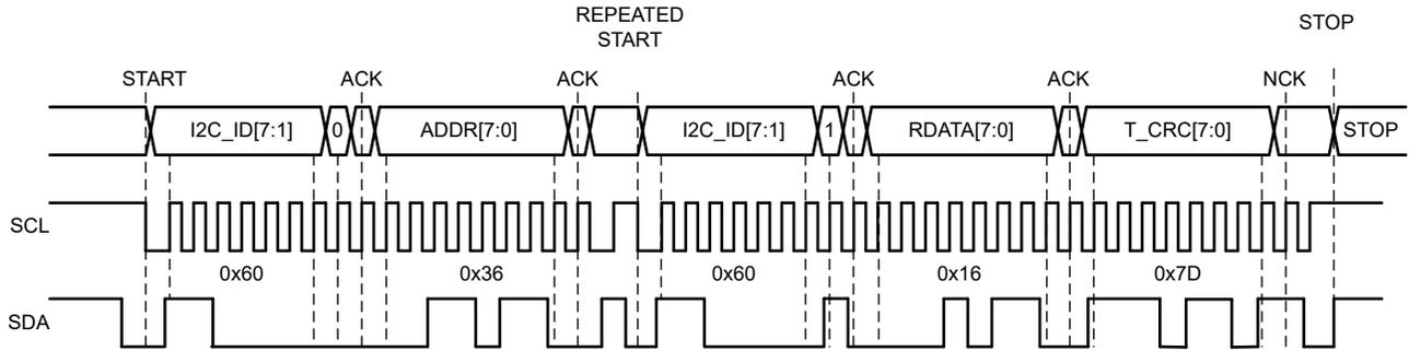
The I<sup>2</sup>C target device (the TPS6593-Q1) provides T\_CRC[7:0], which is calculated from the I2C\_ID, R/W, ADDR, I2C\_ID, R/W, and the RDATA bits (32 bits). See CRC Calculation for I2C and SPI Interface Protocols.
