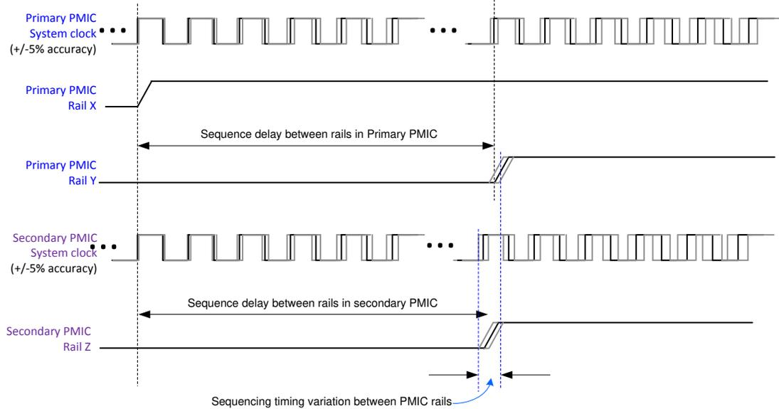
**图 8-45. Multi-PMIC Rail Sequencing Timing Variation**
