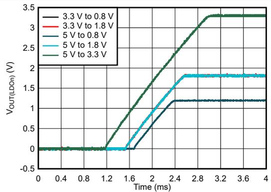
$V_{IN(LDOn)} = 3.3\text{ V or }5\text{ V}$   $TA = 25^\circ\text{C}$
