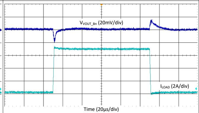
图 9-39. Buck Load Step Transient - 4-Phase, 4.4 MHz, Auto Mode
