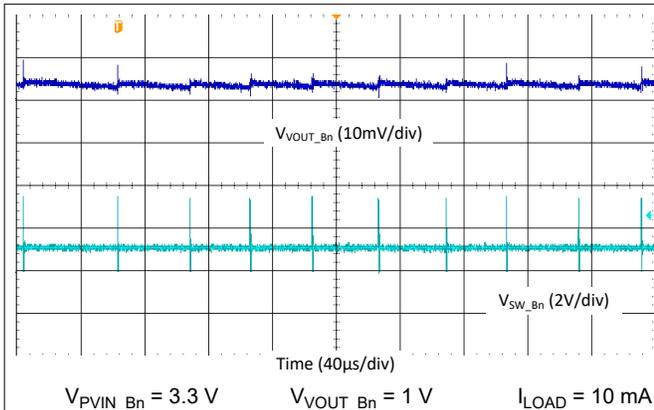
图 9-28. Buck Output Ripple - 3-Phase, Auto Mode
