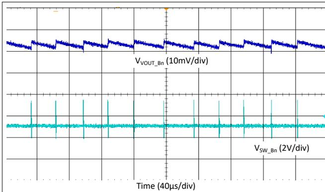
$V_{PVIN\_Bn} = 3.3\text{ V}$     $V_{VOUT\_Bn} = 1\text{ V}$     $I_{LOAD} = 10\text{ mA}$
