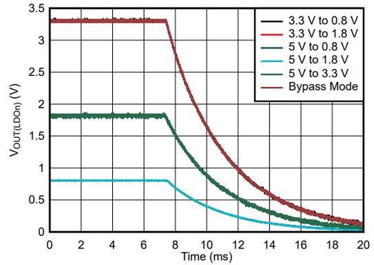
$V_{IN(LDOn)} = 3.3\text{ V or }5\text{ V}$   $LDO_n\_PLDN = 500\ \Omega$   $TA = 25^\circ\text{C}$
