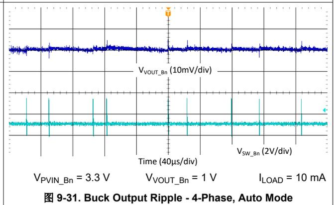
图 9-31. Buck Output Ripple - 4-Phase, Auto Mode
