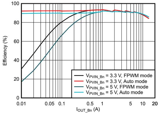
$V_{VOUT\_Bn} = 1.8\text{ V}$   $F_{sw} = 2.2\text{ MHz}$  4-Phase
