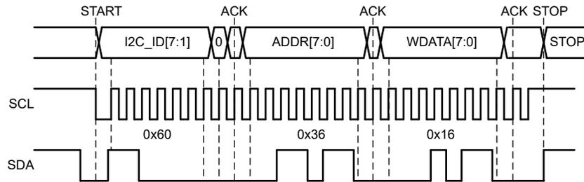
图 8-54. I<sup>2</sup>C Write Cycle without CRC
