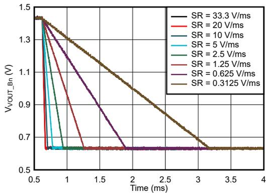
$V_{PVIN\_Bn} = 3.3\text{ V}$  Buck VSET = 1.4 V to 0.6 V TA = 25°C
