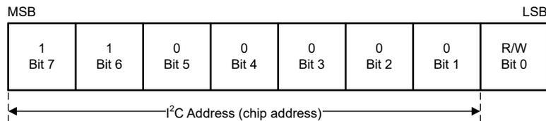
图 8-53. Example Device Address
