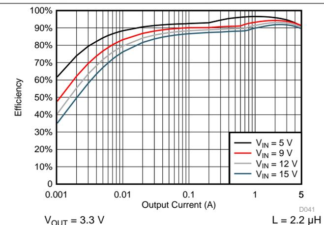
Figure 12. TPS565201 Efficiency vs Output Current
