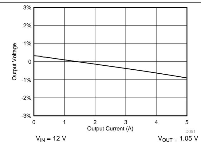
Figure 16. Load Regulation,  $V_{IN} = 12\text{ V}$
