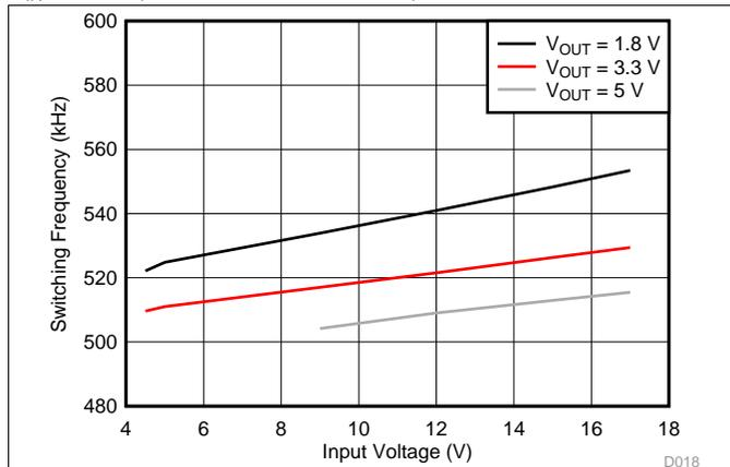
Figure 7. TPS565201 Switching Frequency vs Input Voltage
