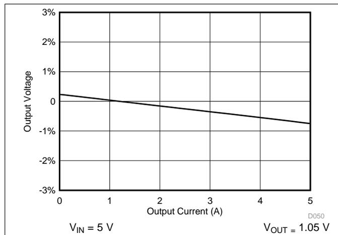
Figure 15. Load Regulation,  $V_{IN} = 5\text{ V}$
