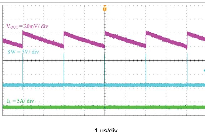
Figure 20. TPS565201 Output Voltage Ripple, No Load
