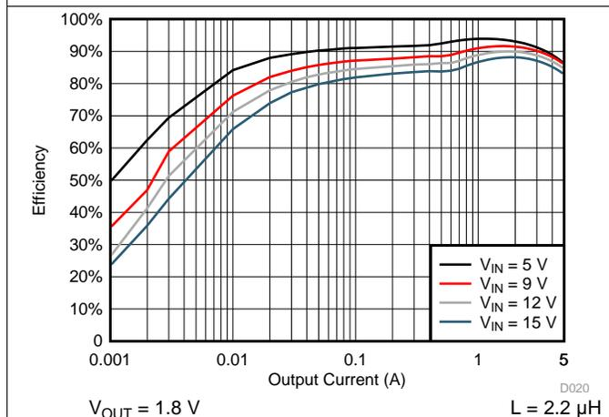
Figure 11. TPS565201 Efficiency vs Output Current
