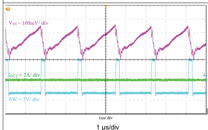
Figure 19. TPS565201 Input Voltage Ripple
