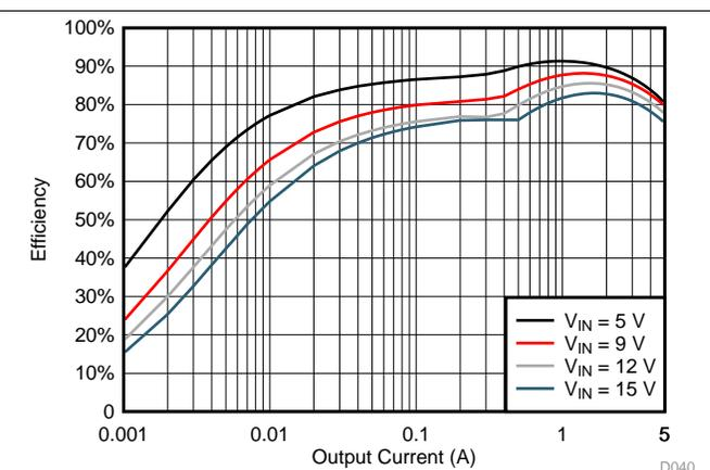
Figure 18. Efficiency vs Output Current
