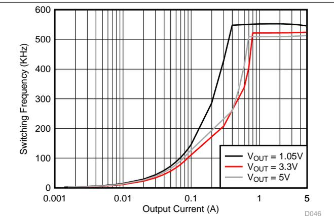
Figure 8. TPS565201 Switching Frequency vs Output Current
