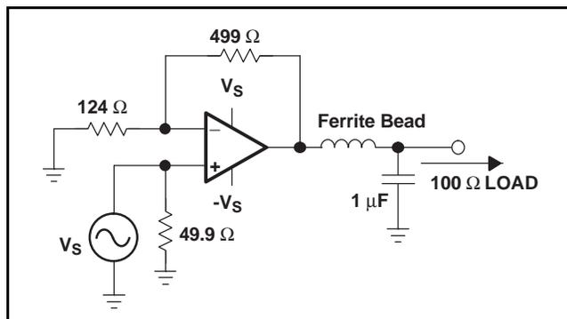
Figure 53. Ferrite Bead to Isolate Capacitive Load
