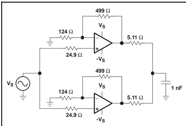
**Figure 56. Parallel Amplifiers for Higher Output Drive**
