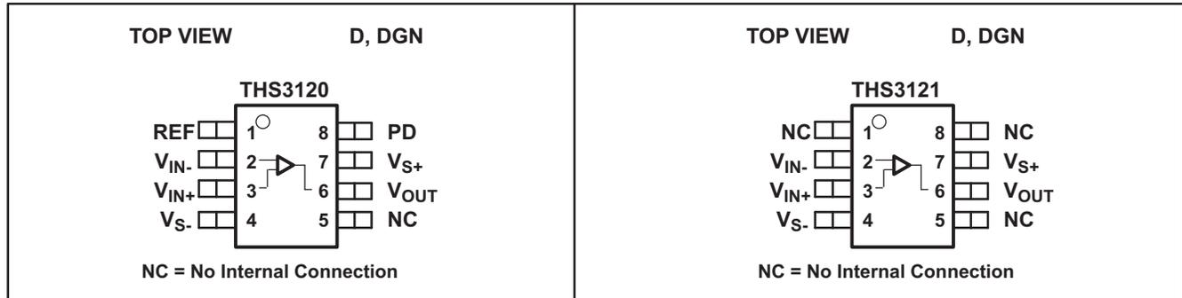
NOTE: The device with the power down option defaults to the ON state if no signal is applied to the PD pin. Additionally, the REF pin functional range is from  $V_{S-}$  to  $(V_{S+} - 4 V)$ .
