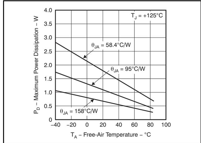
Results are with no air flow and PCB size = 3 inches x 3 inches (76.2 mm x 76.2 mm);  $\theta_{JA} = 58.4^\circ\text{C/W}$  for MSOP-8 with PowerPAD (DGN);  $\theta_{JA} = 95^\circ\text{C/W}$  for SOIC-8 High-K test PCB (D);  $\theta_{JA} = 158^\circ\text{C/W}$  for MSOP-8 with PowerPAD without solder.
