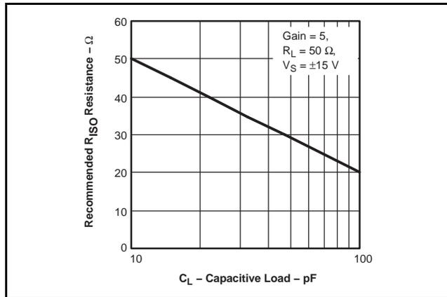
Figure 51. Recommended R<sub>ISO</sub> vs Capacitive Load
